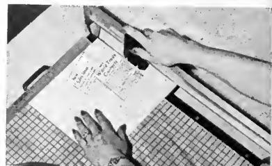
steel, which rotates as it travels on an I-beam track. The wheel blade is enclosed to prevent cutting or pinching fingers. The Crusader Company, Department 179, P.O. Box 368, Woodland Hills, California.
