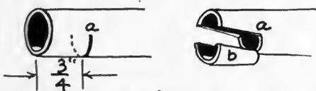
B. Leave  $\frac{1}{3}$  diameter at end of pipe - cut to point (a) to remove section (b).
