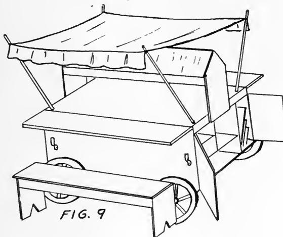
The main body is made from four large pieces of wood: the two hobby horses for the sides and two rectangular pieces—one for the top of the table and the other to be placed underneath about twelve inches from the ground.
