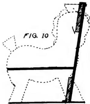
top will not interfere as one will fall down and remain flat along the top, while the other will fold up at the back. (See Fig. 10.) The principle involved is the same as that used in the making of the combination bench and table formerly used on farm porches and now sought after by the antique shops.
