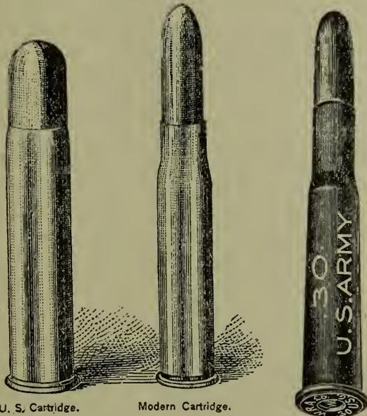
The large cartridge is for the Springfield single loader. It contains 70 grains of powder and 500 grains of lead. The smaller cartridge is for the Krag-Jorgensen, contains about 30 grains of chemical powder and the bullet weighs 230 grains. The bullet is sheathed or jacketed hard metal.
