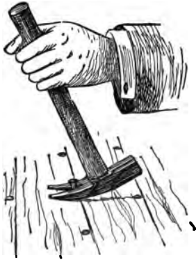
FIG. 100. A hammer: A lever with a short arm near the nail—the fulcrum is the point where the hammer touches the floor —and a long arm from the floor to where your hand takes hold of the handle.
