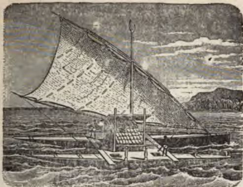
FIG. 385. A double canoe invented by the Fiji Islanders. It will not tip over, you see; and it will go either end foremost by simply shifting the sail.
