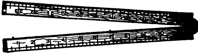
FIG. 47. A carpenter's two-foot rule. It is usually made so as to be only six inches long when folded up.
