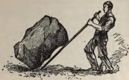
FIG. 97. A stone raised by a crowbar used as a lever. The point where the crowbar rests on the ground is called the fulcrum of the lever—the point about which it turns.
