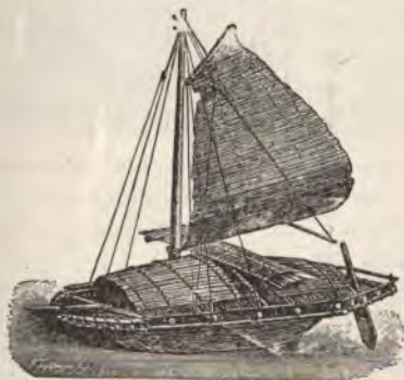
FIG. 386. A boat of the Tagals of the island of Luzon in the Philippines. Notice that the sail and the roofs of the cabins are made of bamboo. Such boats are now in use there,
