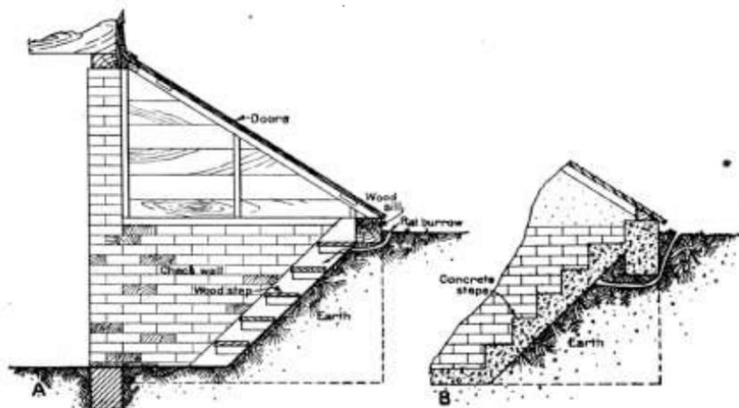
FIGURE 15.—A, Cellarway before rat proofing; B, cellarway rat proofed
