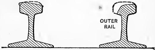
FIG. 121.—RAIL WEAR ON CURVES.
