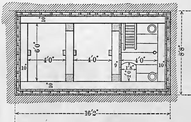
FIG. 91.—CROSS-SECTION, LARGE MAIN SHAFT.
