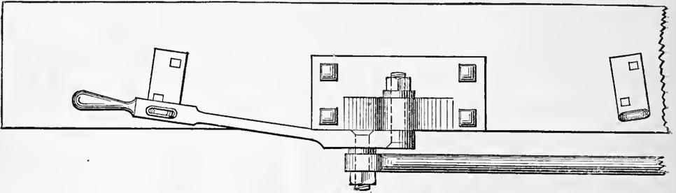
FIG. 134.—GROUND LEVER FOR THROWING A SWITCH.
