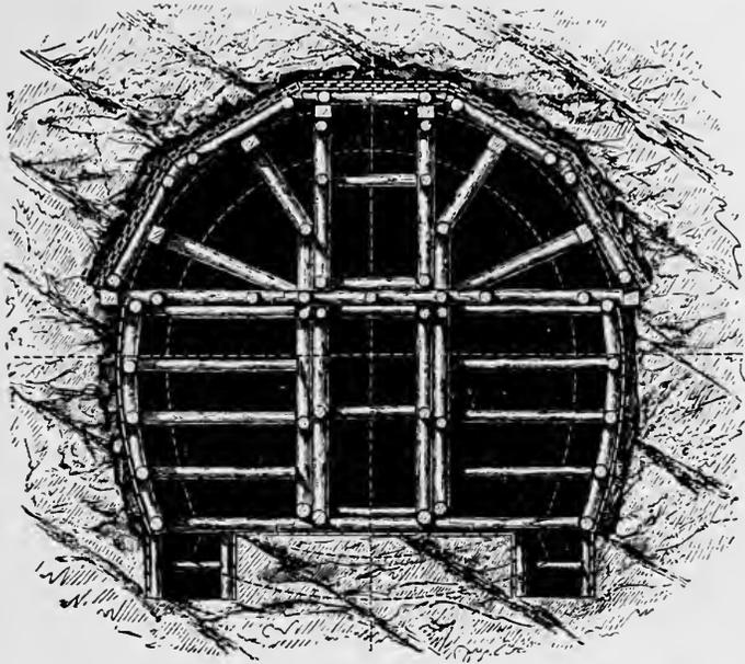
TUNNEL-TIMBERING—AUSTRIAN SYSTEM (*f*).
