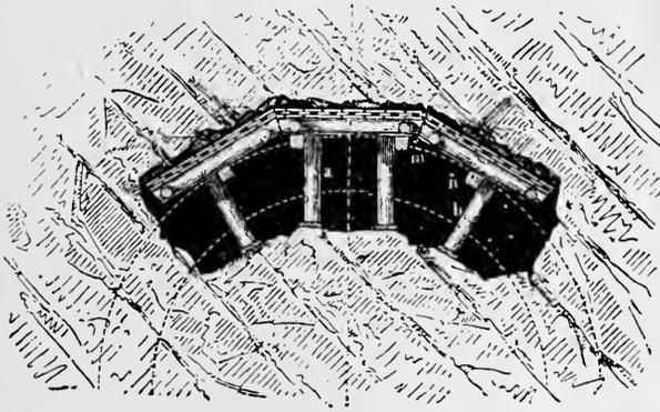
TUNNEL-TIMBERING—AUSTRIAN SYSTEM (b).
