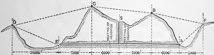
FIG. 85.—SKETCH OF SECTION OF THE HOOSAC TUNNEL.
