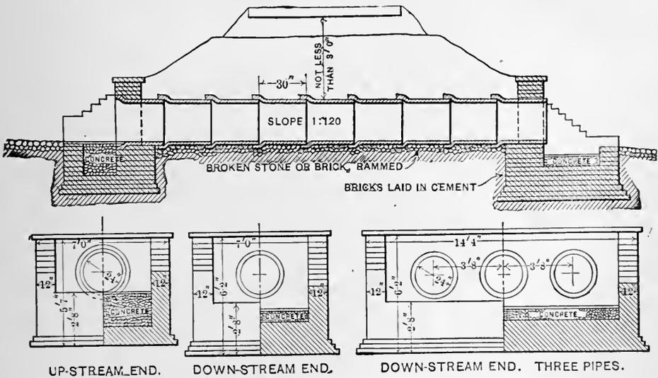
FIG. 98.—STANDARD VITRIFIED-PIPE CULVERT. PLANT SYSTEM. (1891.)
