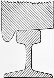
FIG. 114. — RELATION OF RAIL TO WHEEL-TREAD.
