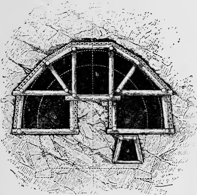
TUNNEL-TIMBERING—GERMAN SYSTEM (c).
