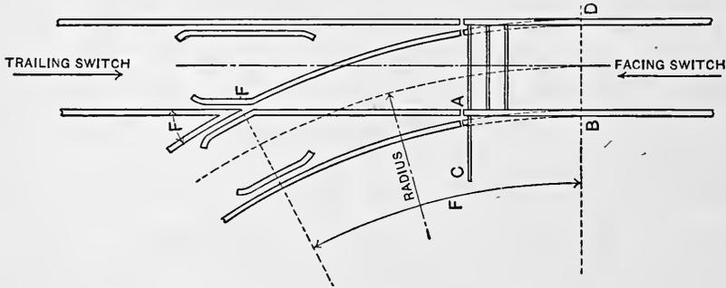
FIG. 131.—STUB SWITCH.
