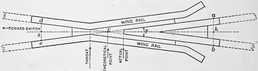
FIG. 130.—DIAGRAMMATIC DESIGN OF FROG.
