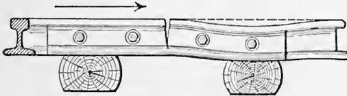
FIG. 118.—EFFECT OF “WHEEL DROP” (EXAGGERATED).
