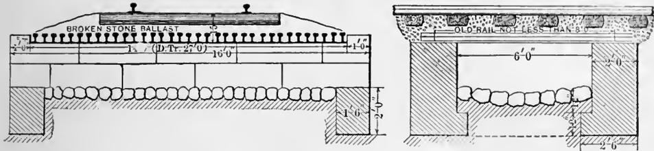
FIG. 101.—STANDARD OLD-RAIL CULVERT. N. & W. R.R. (1895.)
