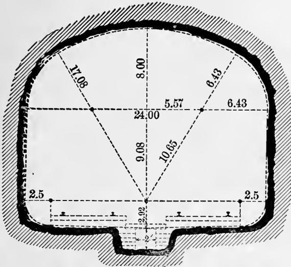
FIG. 87.—HOOSAC TUNNEL. SECTION THROUGH SOLID ROCK.
