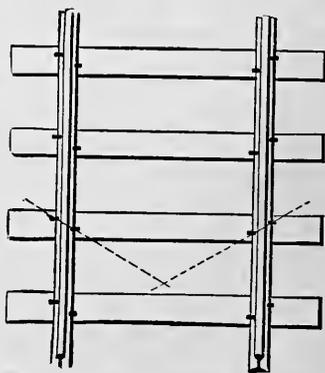
FIG. 124. SPIKE-DRIVING. This will tend to prevent any twisting of the tie in the ballast, which would otherwise loosen the rail from the tie.
