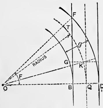
is to consider that the lead-rails curve out from the main track-rails by arcs of circles which are tangent to the main rails and which extend to the frog-point *F*. The simple curve from *D* to *F* is of such radius that  $(r + \frac{1}{2}g)$  vers  $F = g$ , in which  $F$  = the frog angle,  $g$  = gauge,  $L$  = the “lead” ( $BF$ ), and  $r$  = the radius of the center of the switch-rails.
