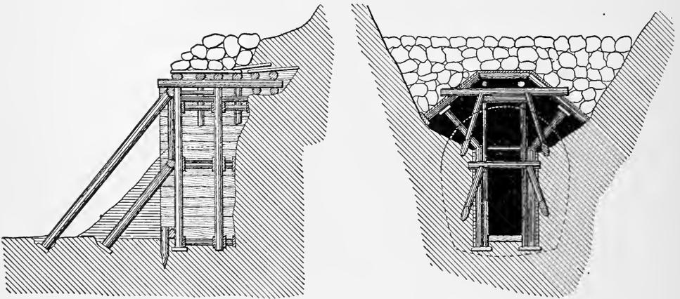
FIG. 96.—TIMBERING FOR TUNNEL PORTAL.
