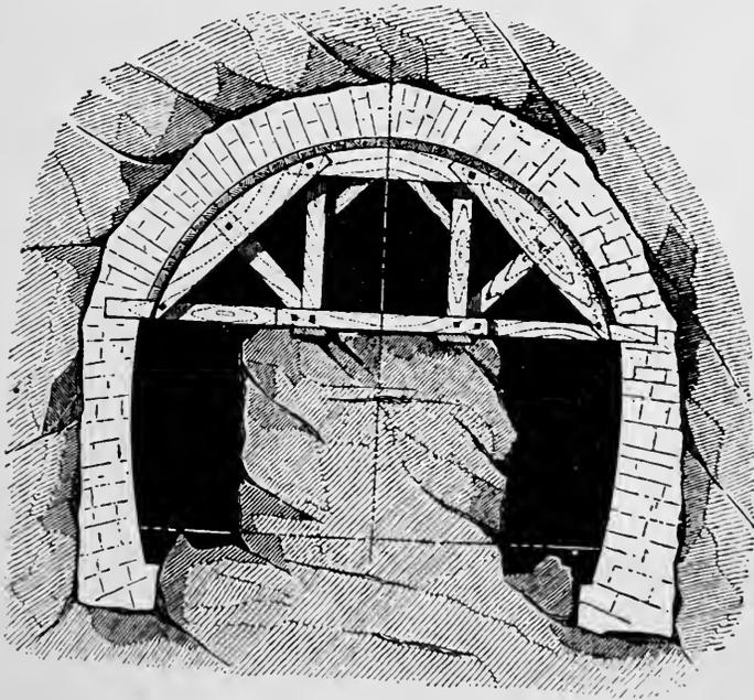
TUNNEL-TIMBERING—FRENCH SYSTEM (b).
