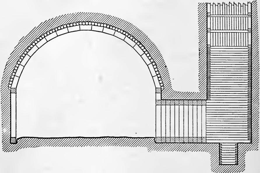
FIG. 90.—CONNECTION WITH SHAFT, CHURCH HILL TUNNEL.
