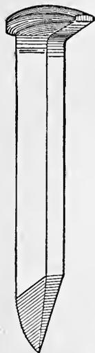
FIG. 123. the fibers to press still harder on the spike and thus increase the resistance.
