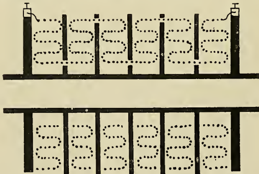
FIG. 7.—Diagram of sectional winding of secondary coil. (R. S. Wright, A. M.I.E.E.)
