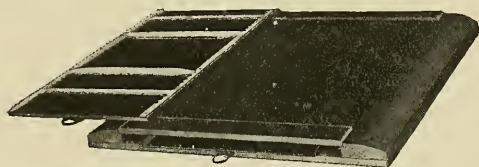
FIG. 133.—Gouldsbrough's plate-holder, with displaceable centre. (A. E. Dean.)
