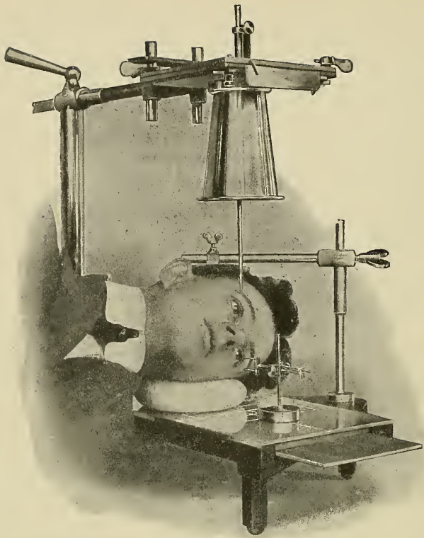
FIG. 149.—Sweet's eye localiser. Position of tube for first exposure. (A. E. Dean.)
