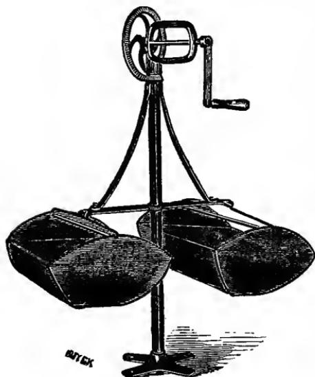
This machine consists of a central spindle, set in a base that is screwed fast to the floor or a wide board. The gearing is placed on the top of this spindle, and by turning the crank, the suspended arms are made to revolve around the spindle as rapidly as is necessary. On a hook on the end of each arm is hung a peculiarly-shaped bucket of tin, over which is laid a frame of wire cloth.
