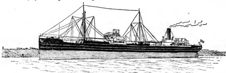
Twin-Screw Cargo Vessel *Monte Penedo*. Fitted with Two-Stroke Single-Acting Diesel Motors
