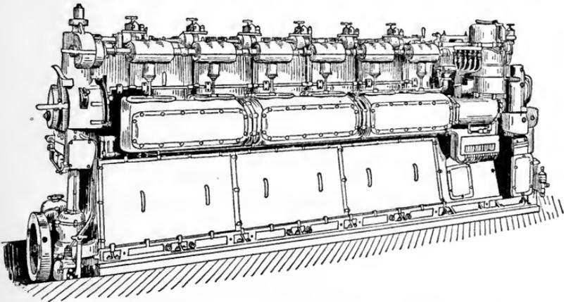
Four-Stroke, Direct-Reversible Diesel Marine Engine
