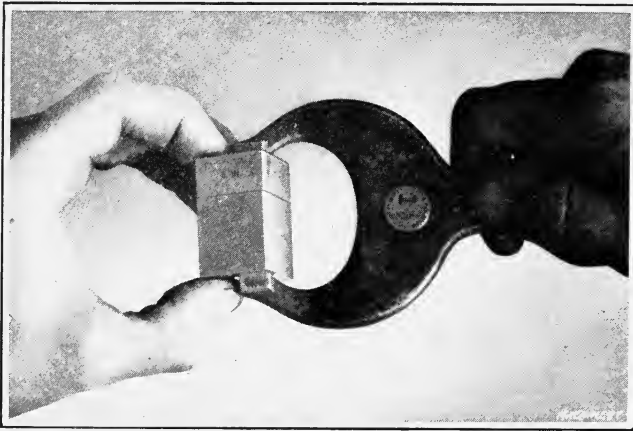
Fig. 33. Size Blocks being used to check the Distance between the Gaging Surfaces of a Snap Gage
