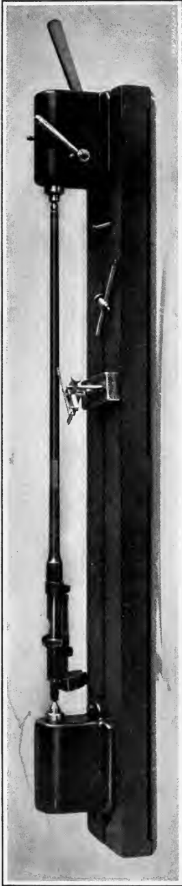
Fig. 30. Indicator set on Bench Centers for testing the Concentricity of a Rifle Barrel
