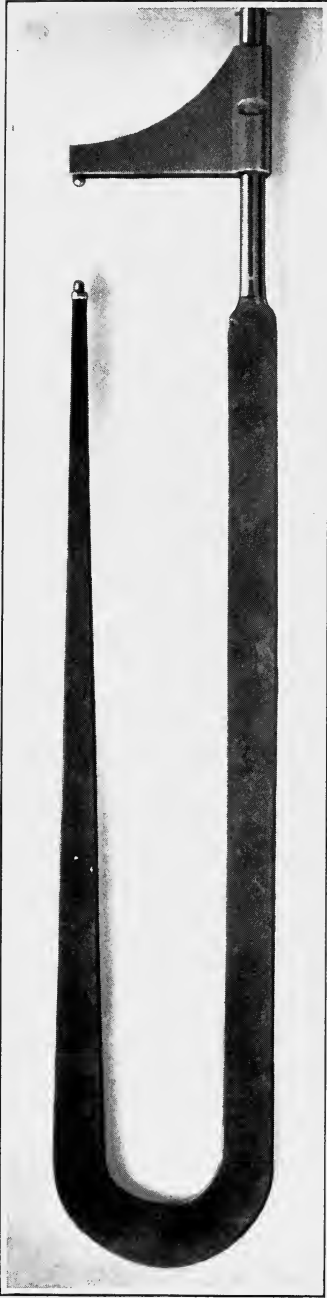
Fig. 19. Sliding-bar Gage used in testing the Thickness of the Bottom of a Shell
