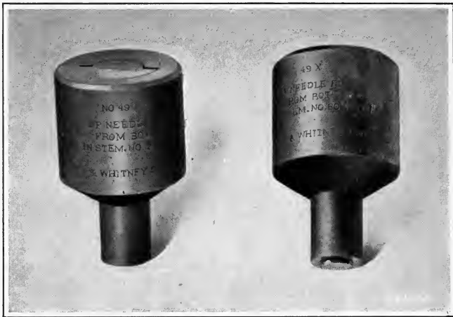
Fig. 18. Simple Form of Flush-pin Gage, consisting of a Plunger which slides in a Sleeve
