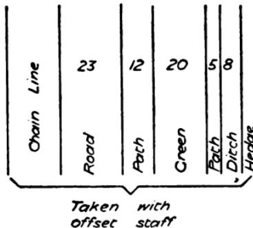
FIG. 30.—Measurements taken with offset-staff.
