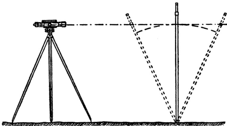
FIG. 128.—Obtaining reading when staff is vertical.
