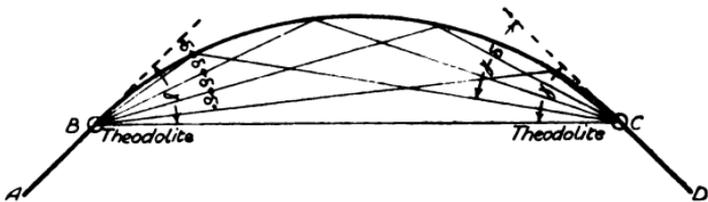
FIG. 208.—Setting out curves with two theodolites.
