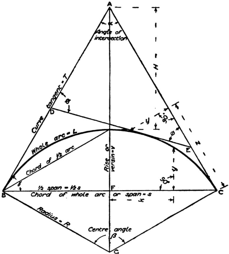
FIG. 190.—Diagram showing curve elements.
