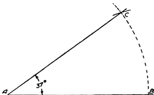
FIG. 155.—Setting off angle by scale of chords.
