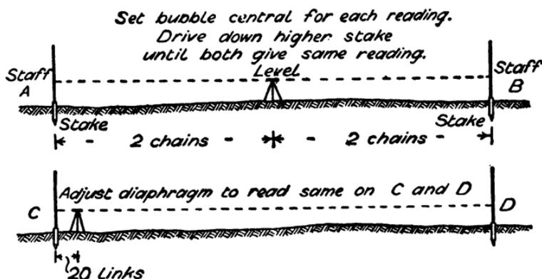
FIG. 127.—Adjustment of level for collimation.
