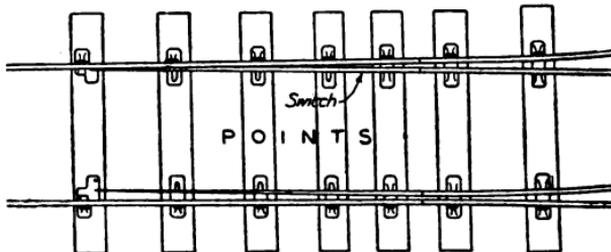
FIG. 210.—Pair of points or switches.
