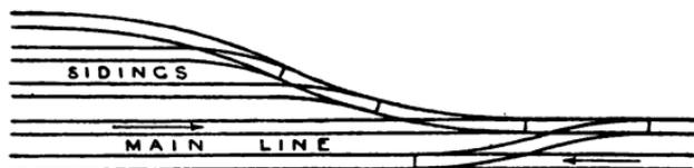
FIG. 213.—Connection of sidings with main line.
