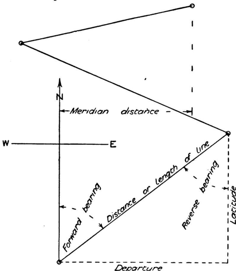
FIG. 107.—Illustration of terms used in compass traversing.
