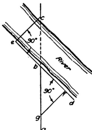
FIG. 73.—Measuring width of river diagonally.
