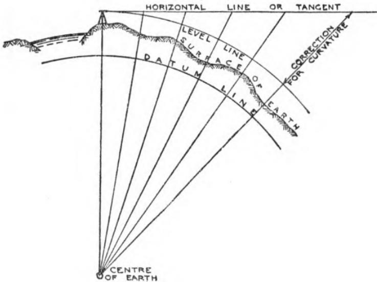
FIG. 123.—Correction for curvature.
