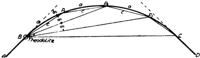
FIG. 207.—Setting out curves with one theodolite.
