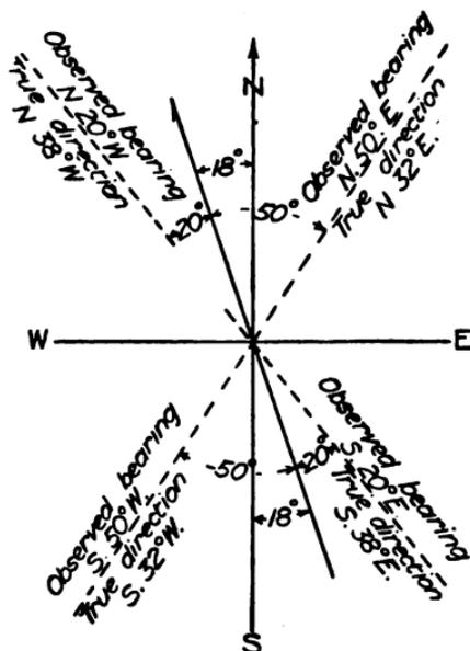
FIG. 104.—True direction of lines.
