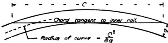
FIG. 206.—Finding radius of existing curve.
