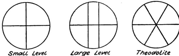
FIG. 126—Arrangement of wires in levels and theodolite.
