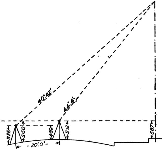
FIG. 170.—Sketch showing necessary observations to find the height of a church spire.
