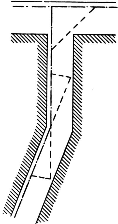
Fig. 177.—Tying bend in street in chaining.
