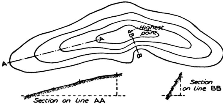
FIG. 90.—Plan of contour lines round a hill.
