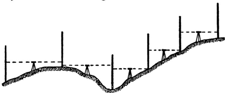
FIG. 124.—Compound levelling.
