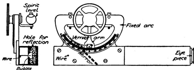
FIG. 87.—Abney's reflecting level.
