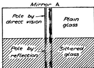
FIG. 63.—Enlarged view of mirror.
