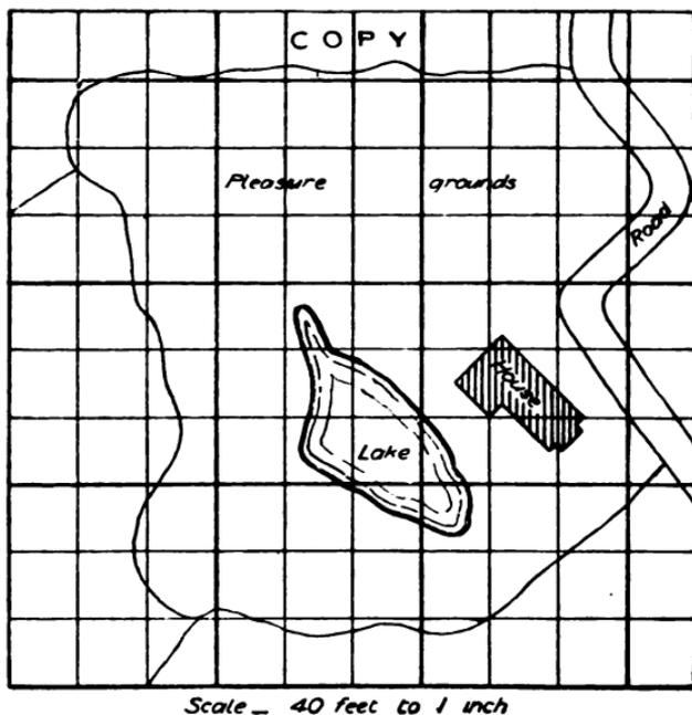
FIG. 114.—Method of enlarging by proportional squares.
