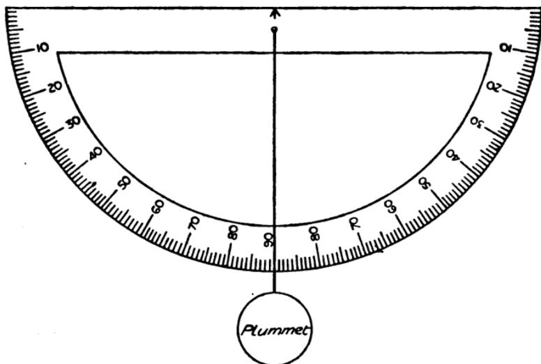
FIG. 85.—Protractor with plummet.
