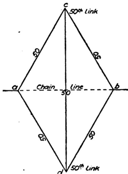
FIG. 66.—Setting off perpendicular to line.
