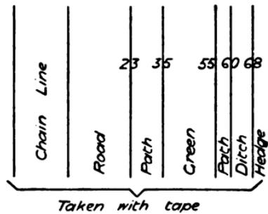
FIG. 31.—Measurements taken with tape.
