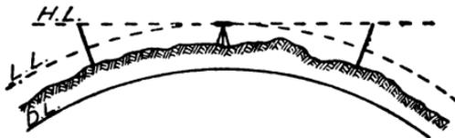
FIG. 125.—Corrections equal when distances equal.
