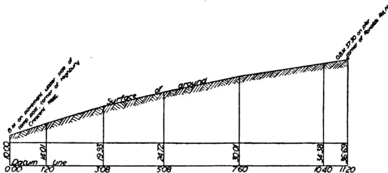
FIG. 182.—Section plotted from Fig. 181.
