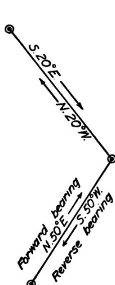
FIG. 103.—Forward and reverse bearing of line.
