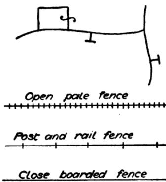
FIG. 40.—Methods of showing fences and boundaries.
