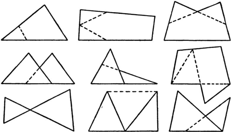
FIG. 52.—Main lines for surveys.
