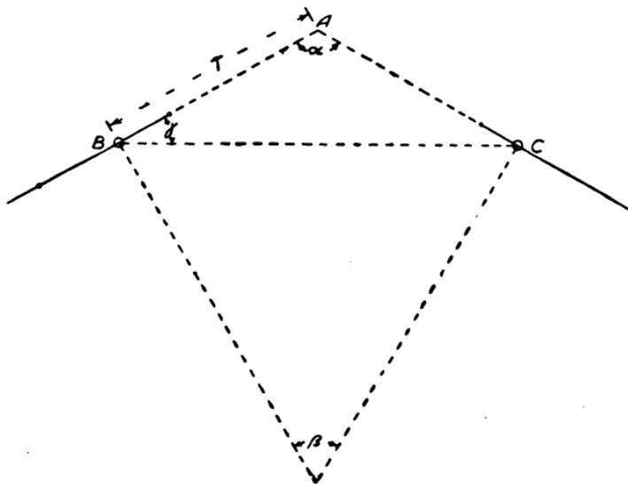
FIG. 209.—Practical example of setting out curve.
