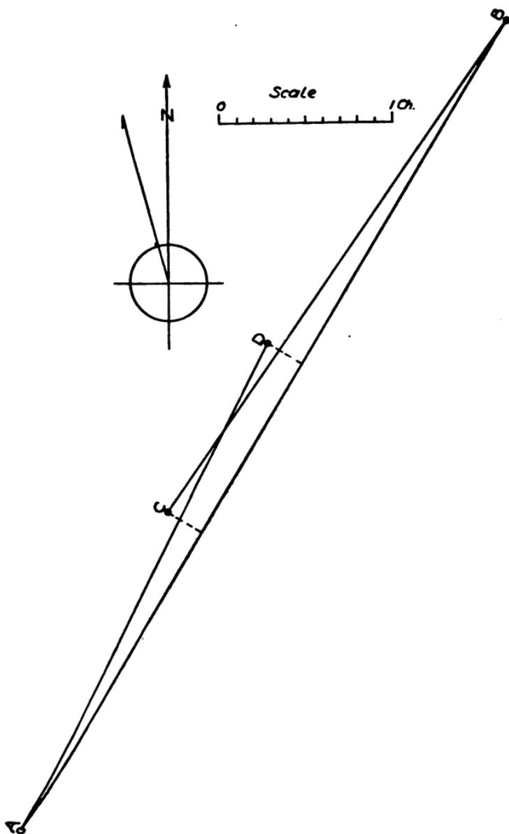
FIG. 43.—Method of poling out the line over hilly ground.
