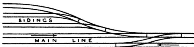
FIG. 213.—Connection of sidings with main line.
