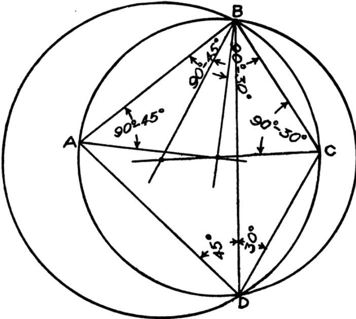
FIG. 161A.—Three-point problem in plane-tableing.
