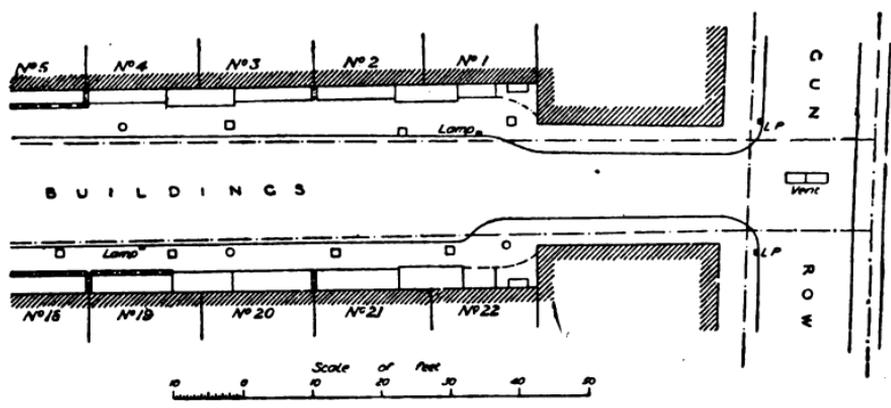
FIG. 178.—Detail plotting of street in town survey.
