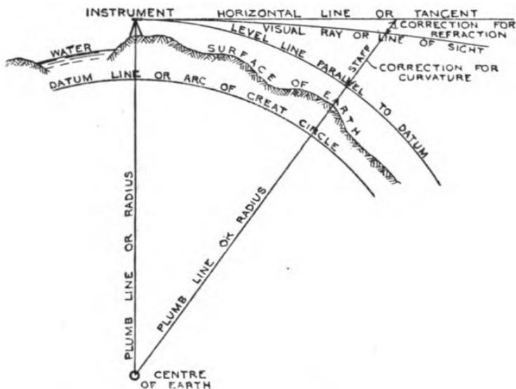
Fig. 122.—Difference between level and horizontal lines.
