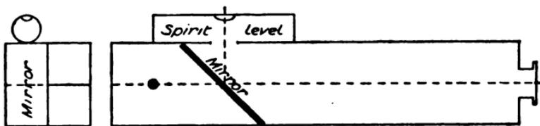
FIG. 91.—Hand reflecting level.
