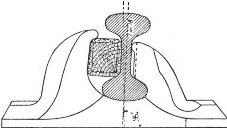
FIG. 196.—Double-headed rail in a cast-iron chair.
