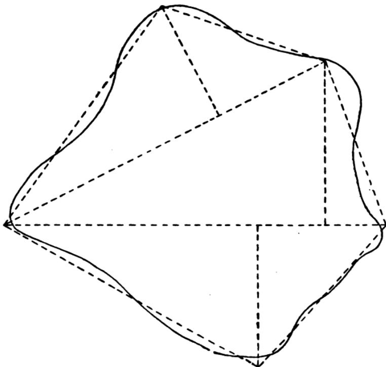
FIG. 47.—Obtaining area of irregular figure.
