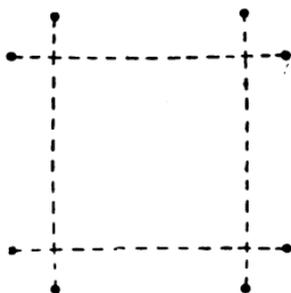
FIG. 182.—Pegs for setting out a square block.
