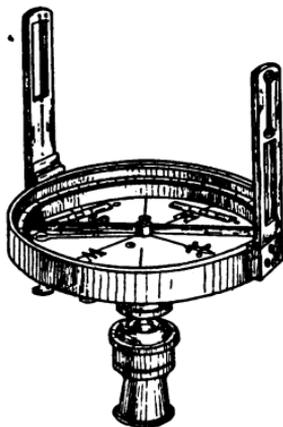
FIG. 105.—Surveyors' compass.
