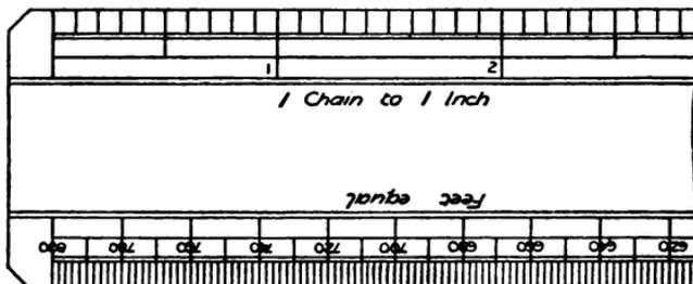
FIG. 13.—Scale of chains and feet corresponding.
