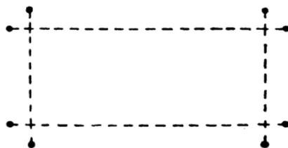
FIG. 183.—Pegs for setting out a trench.
