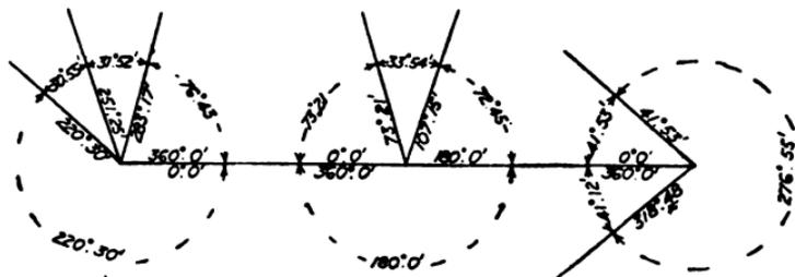
FIG. 163.—Recording angles on chain lines.
