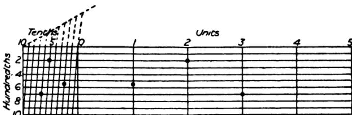
FIG. 156.—Diagonal scale.
