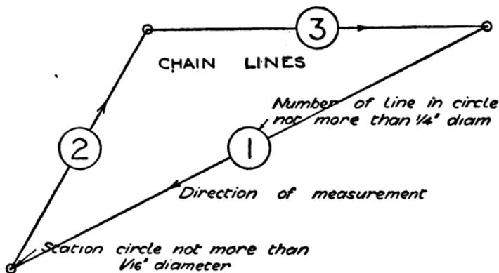
FIG. 28.—Drawing chain lines on plan.
