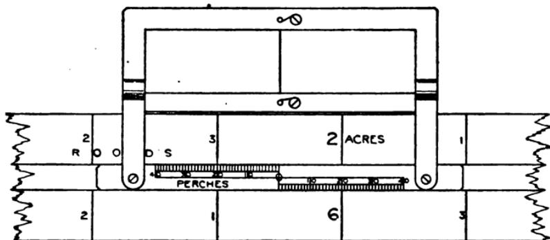
FIG. 48.—Computing scale.
