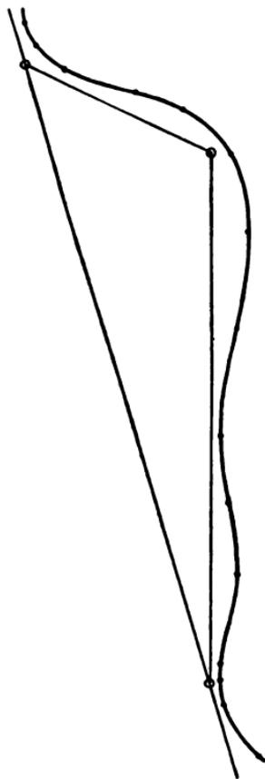
FIG. 34.—Supplementary triangle on chain line.
