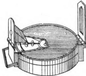
FIG. 100.—General view of prismatic compass.
