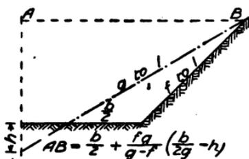
FIG. 184.—Formulæ for earthwork calculations (side-widths).
