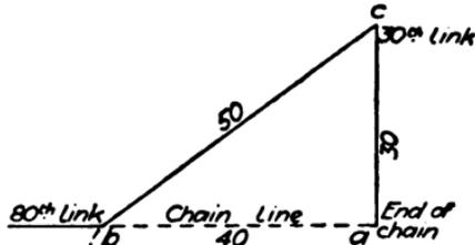
FIG. 64.—Setting off right angle with chain.
