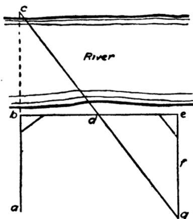
FIG. 72.—Measuring width of river at right angles.
