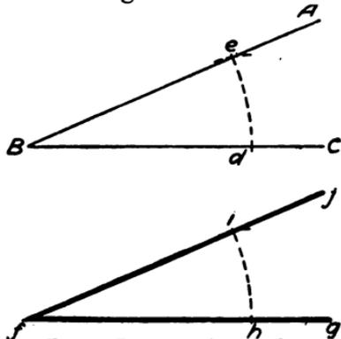
FIG. 3.—To copy a given angle.
