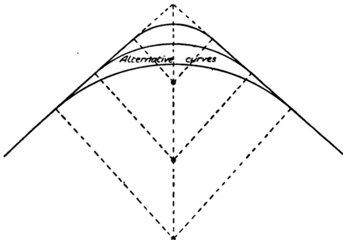
FIG. 187.—Simple curve.
