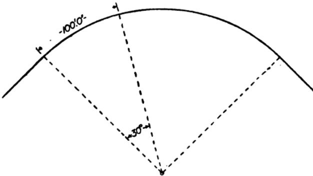
FIG. 186.—“30 degree curve.”
