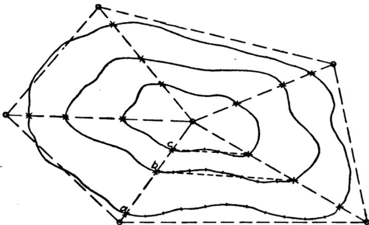
FIG. 92.—Method of setting out contour lines.
