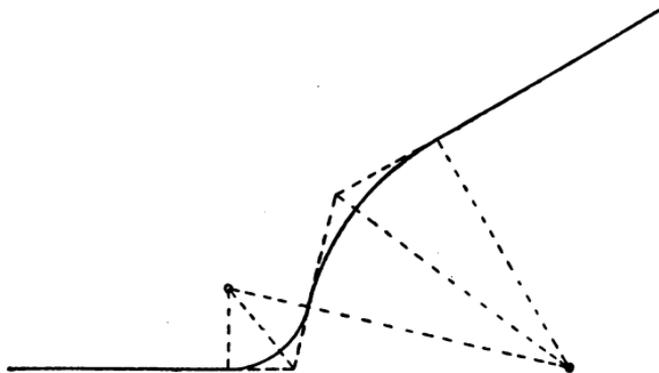
FIG. 189.—Inverted, reverse, or S curves.
