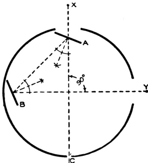
FIG. 62.—Plan of optical square.
