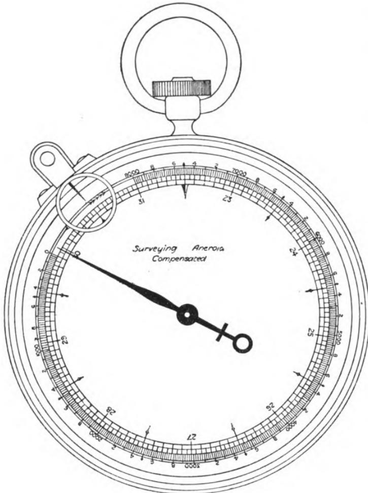
FIG. 149.—Aneroid barometer.
