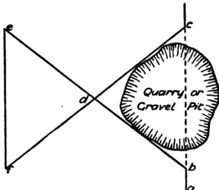
FIG. 75.—Measuring across quarry or gravel pit.
