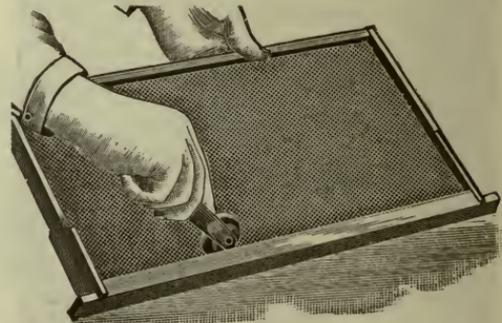
Fig. 5.—Foundation roller for fastening in frames. (After A. I. Root Co.)
