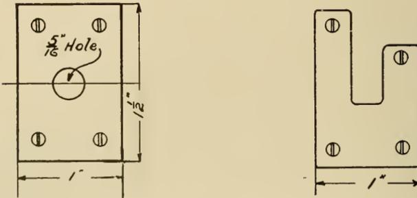
Fig. 11.—Simple wooden holder for curtain rods.
