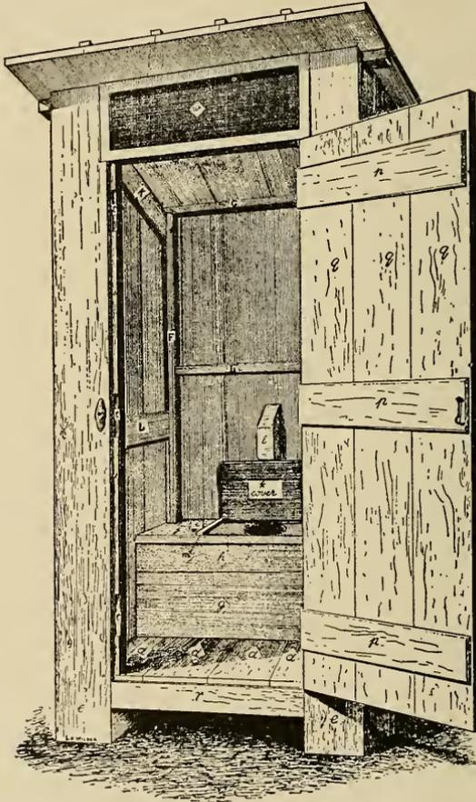
Fig. 28.—A single-seated sanitary privy. Front view. (After Stiles.)
