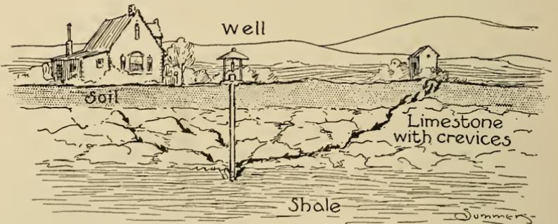
Fig. 40.—Contamination through crevices.
