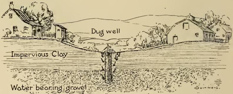
Fig. 38.—Surface contamination.
