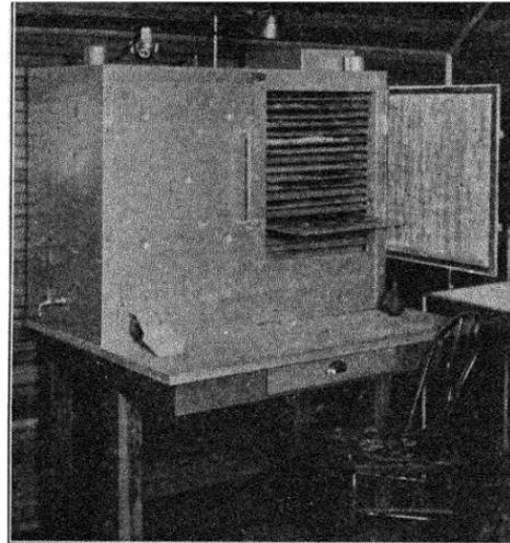
FIG. 64.—A common commercial type of seed germinator. The cloths or blotters holding the seeds are placed on the sliding trays. The germinator is heated by an electric plate and the temperature is controlled by a thermostat.
