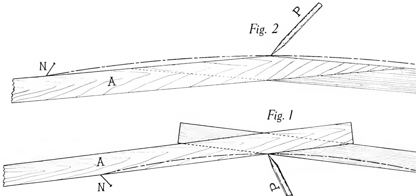
**F**OR laying out true sweeps or curves where it is impractical to strike the radius with the compasses or trammel points, we illustrate the following example, and although the principle has long been in use, it is unknown to a great many mechanics.
