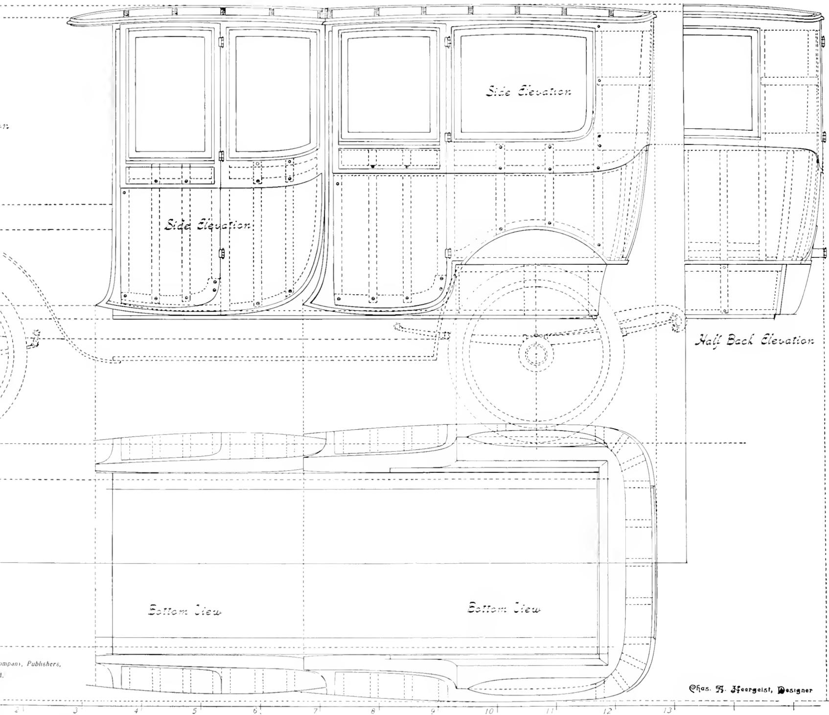
FIG. 1. PLAN OF AN EXTENSION-FRONT BROUGHAM BODY, SHOWING SIDE ELEVATION, HALF FRONT AND HALF BACK ELEVATION AND BOTTOM VIEW.
