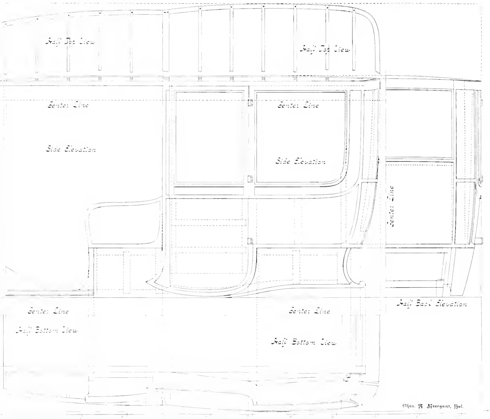
41 1/2" SIZE LIMOUSINE BODY WITH SOLID REAR CORNERS, FITTED TO A THREE-INCH DROP FRAME.
