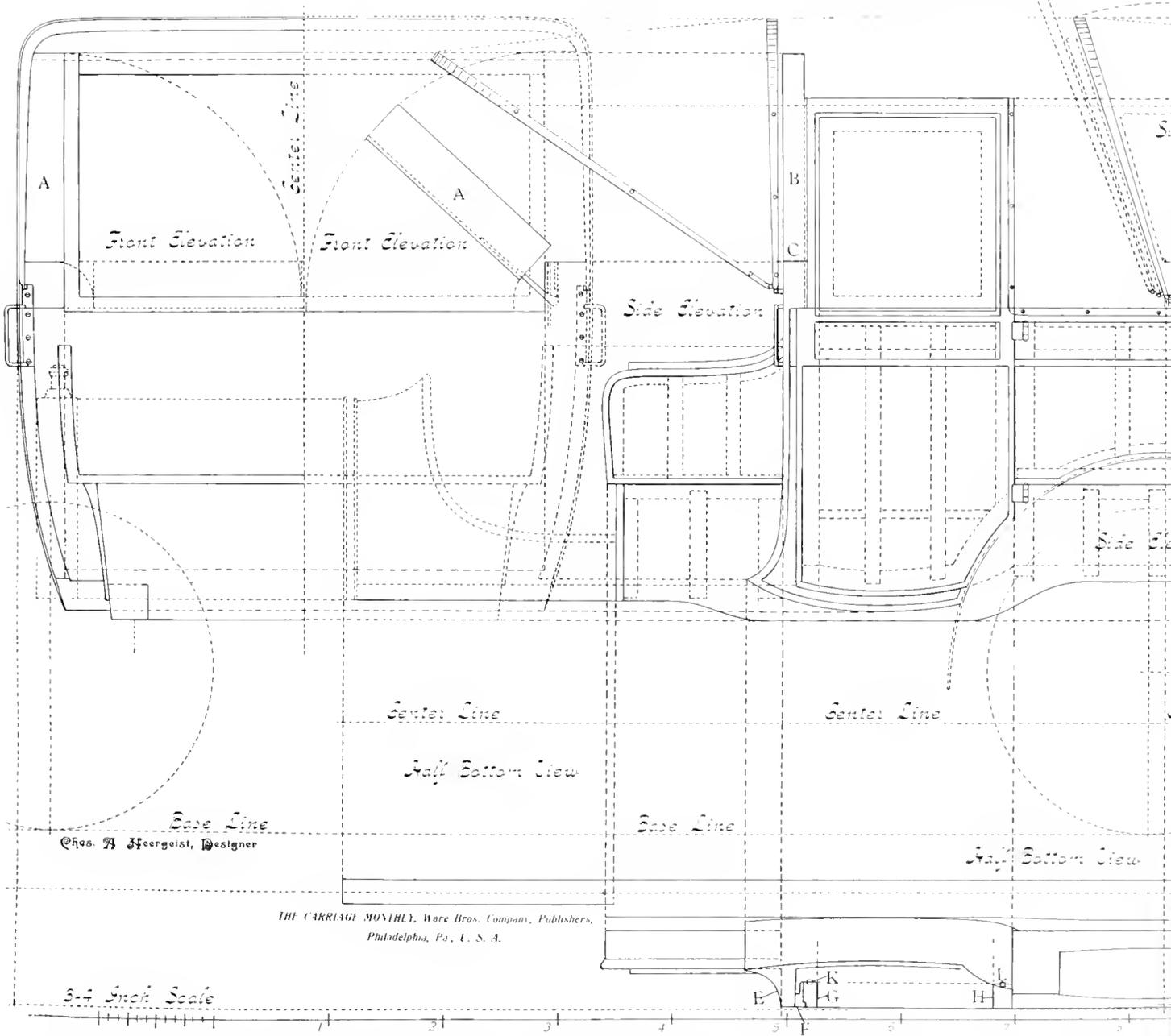
WORKING DRAFT OF TOURING CAR BODY, WITH NEW FOLDING TOP, DROP CHASSIS, ILLUSTRATING FRONT, SIDE AND BOTTOM VIEW.
