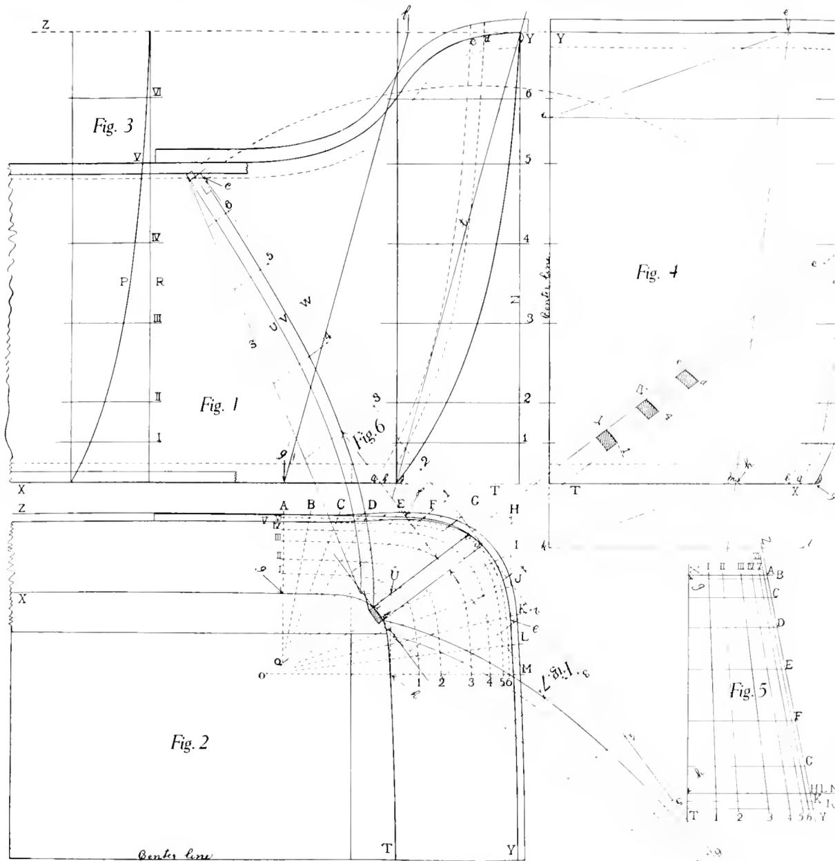
ILLUSTRATING THE PROPORTIONAL CORNER, HORIZONTAL SECTIONS AND CORNER STRAIGHT
