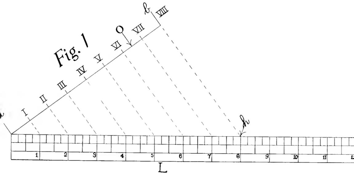
s to divide a line  $6\frac{1}{2}$  inches long into 7 parts. The easiest and quickest method is
