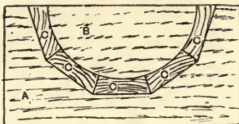
Fig. 83.—Half Box for Large Circular Core.
