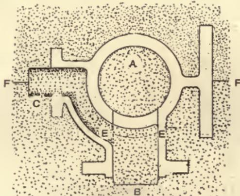
Fig. 99.—Mould for Engine Cylinder.
