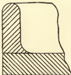
Fig. 41.—Fillet Worked Out of Flange.
