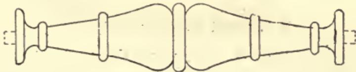
Fig. 57.—Pillar with Chucking Pieces at Each End.
