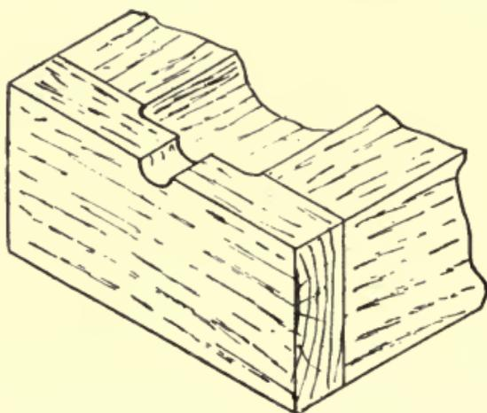
Fig. 79.—Core-box with End of Small Diameter.
