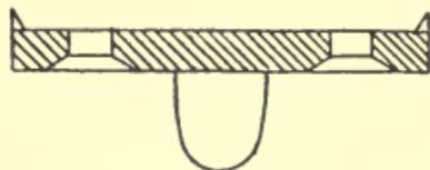
Fig. 30.—Section of Metal Peg Dowel.
