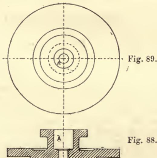
Figs. 88 and 89.—Casting of Cylinder Cover.
