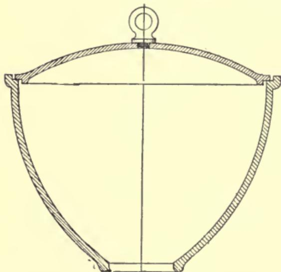
Fig. 66.—Section of Circular Pan, with Cover.
