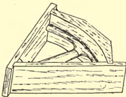
Fig. 87.—Core-box for Making Flywheel.
