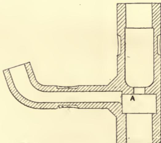
Fig. 278.—Core-box for Body for Screw-down Valve.
