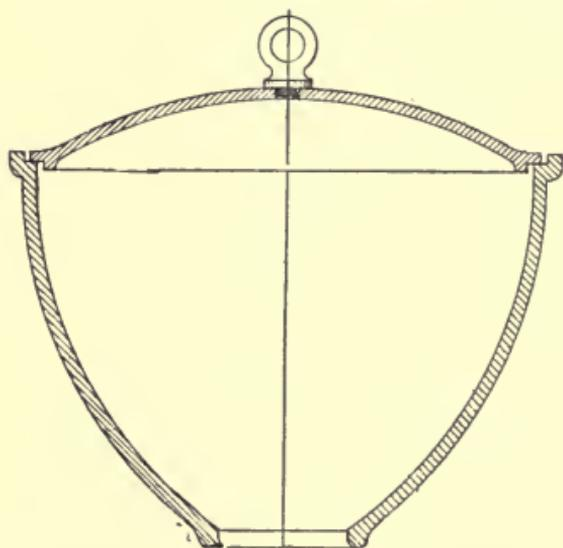
Fig. 66.—Section of Circular Pan, with Cover.
