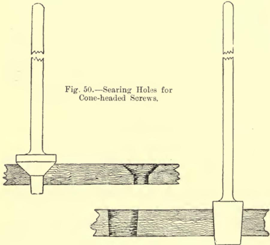
Fig. 50.—Searing Holes for
