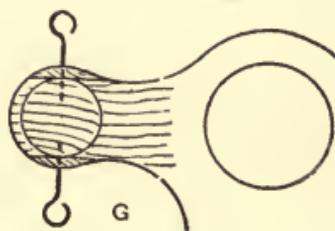
Fig. 228.—Curved Horn for Mandrel Bearings.
