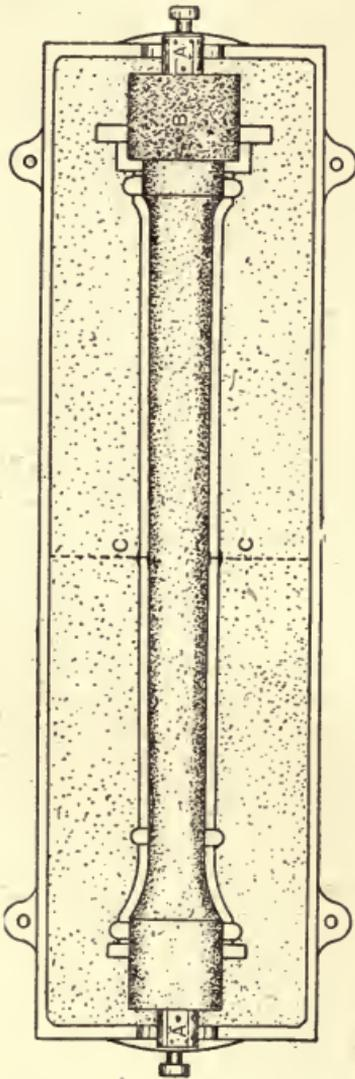
Fig. 157.—Plan of Mould for Columns.
