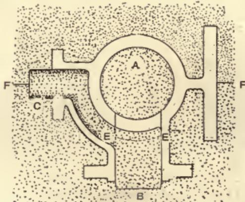
Fig. 99.—Mould for Engine Cylinder.
