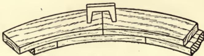
Fig. 62.—Segments Tightened with Dog.
