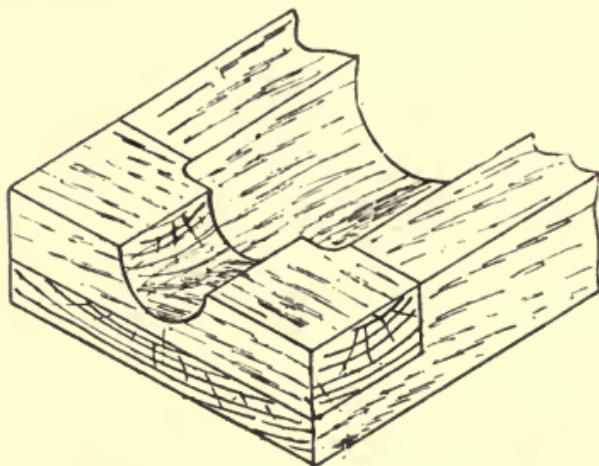
Fig. 78.—Core-box for Chamber Core.
