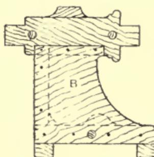
Fig. 250.—Half of Lathe Poppet Pattern.
