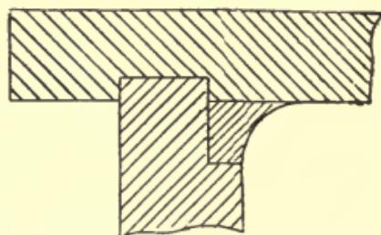
Fig. 45.—Fillet for Core-box with Loose Ends.
