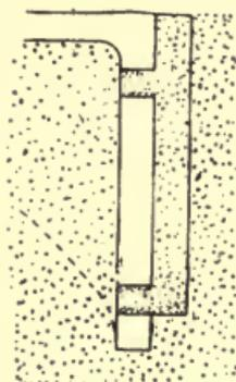
Fig. 123.—Section through Portion of Cored Mould.
