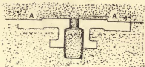
Fig. 93.—Mould for Cylinder Cover.
