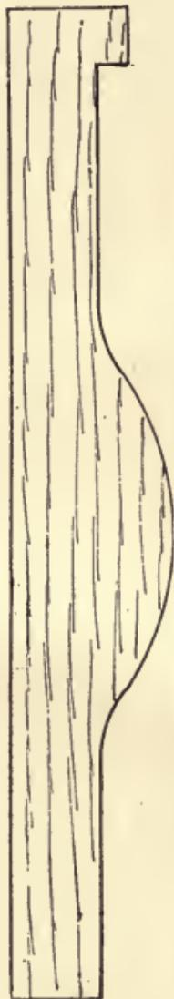
Fig. 288.—Shouldered Template for Globe Valve Core-box.
