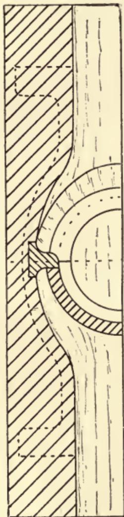
Fig. 287.—Section of Globe Valve Core-box.
