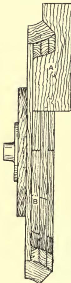
Fig. 192.—Turning Inside of Wheel Rim by Template.
