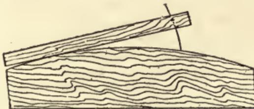
Fig. 194.—Template for Marking Tooth Curves.
