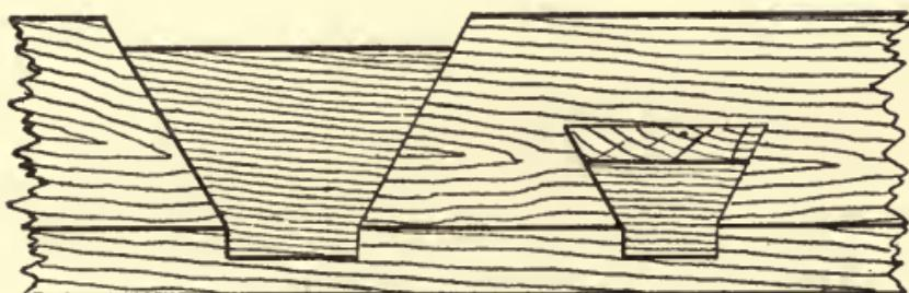
Fig. 22.—Dovetail Half-check.
