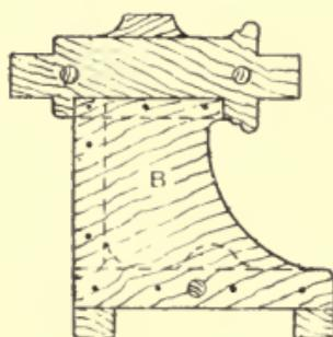
Fig. 250.—Half of Lathe Poppet Pattern.
