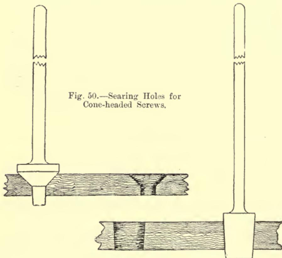
Fig. 50.—Searing Holes for
