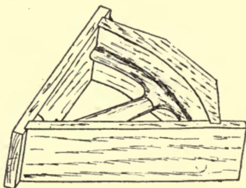
Fig. 87.—Core-box for Making Flywheel.
