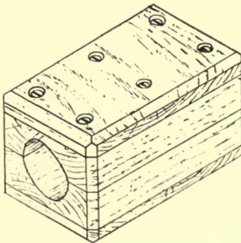
Fig. 70.—Core-box for Plain Circular Core.
