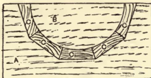
Fig. 83.—Half Box for Large Circular Core.
