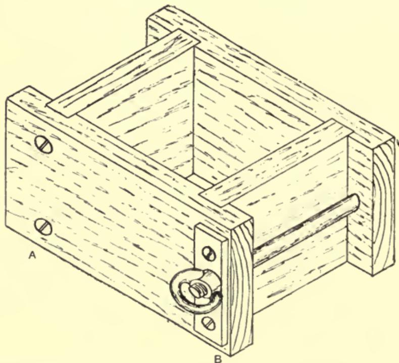
Fig. 82.—Built-up Box for Large Rectangular Core.
