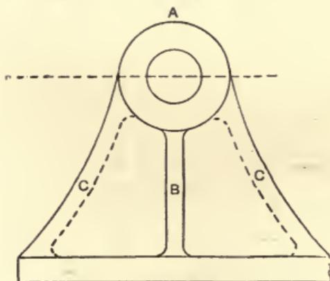
Fig. 146.—Double Bracket Casting.
