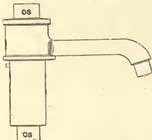
Fig. 277.—Body Pattern for Screw-down Valve.
