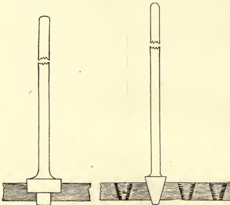
Fig. 51.—Searing Hole for Cheese-headed Screw.
