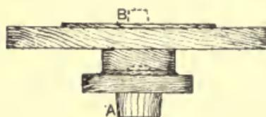
Fig. 90.—Cylinder Cover Pattern.
