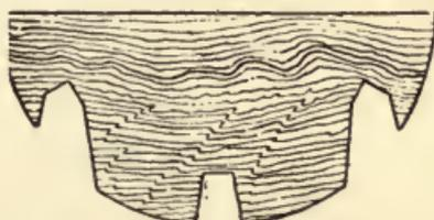
Fig. 139.—Stopping-over Piece used without Prints.
