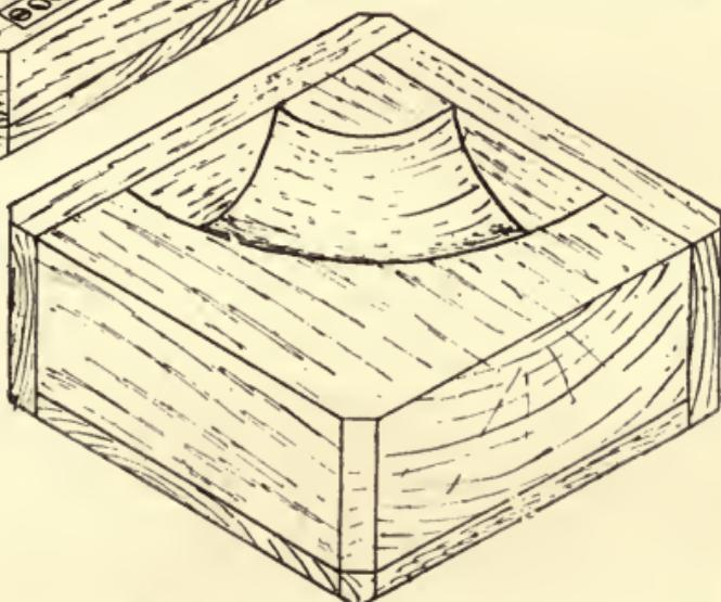
Fig. 72.—Core-box for Bend-pipe.
