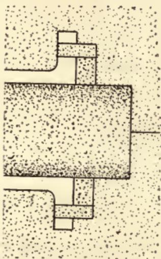
Fig. 138.—Mould for Pipe Casting, with Cores Inserted.
