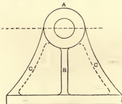
Fig. 146.—Double Bracket Casting.
