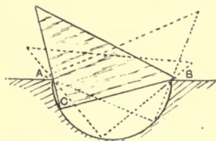
Fig. 74.—Working Out Circular Core-box with Set-square.
