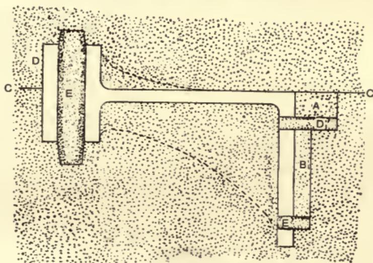
Fig. 122.—Section through Cored Mould.
