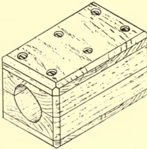
Fig. 70.—Core-box for Plain Circular Core.
