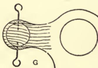
Fig. 228.—Curved Horn for Mandrel Bearings.
