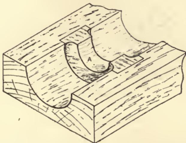
Fig. 76.—Internal Flange Fitted into Core-box.
