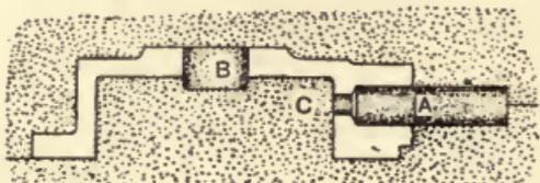
Fig. 110.—Mould for Steam-chest.
