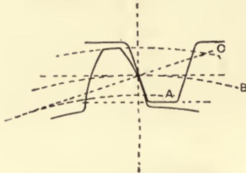
Fig. 193.—Forms of Teeth on Worm and Wheel.
