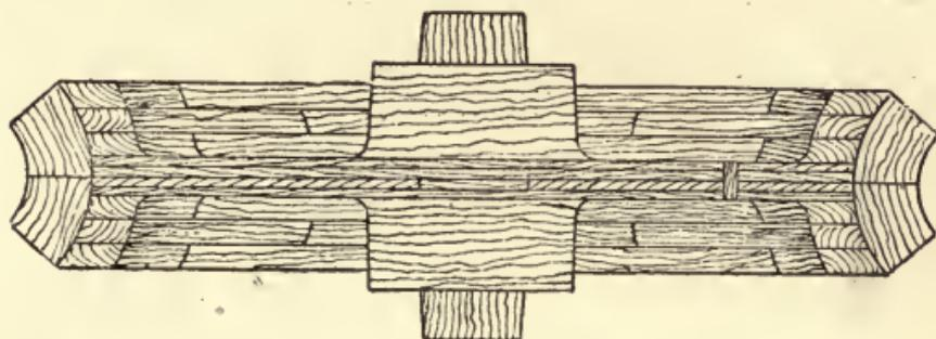
Fig. 196.—Cross Section of Finished Worm Wheel Pattern.
