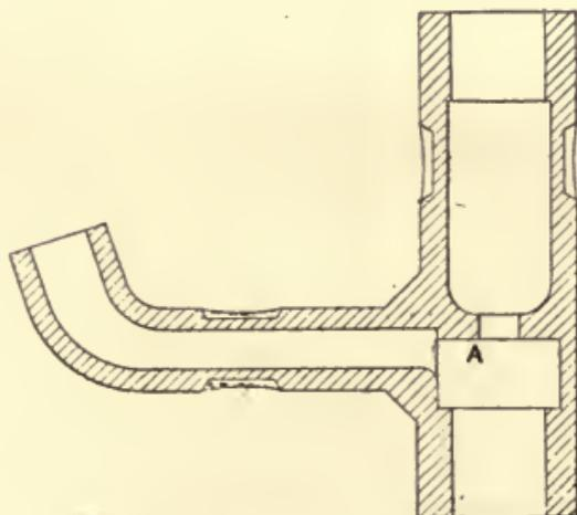
Fig. 278.—Core-box for Body for Screw-down Valve.
