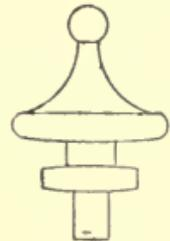
Fig. 56.—Correct Shape for Knob Pattern.
