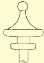
Fig. 56.—Correct Shape for Knob Pattern.
