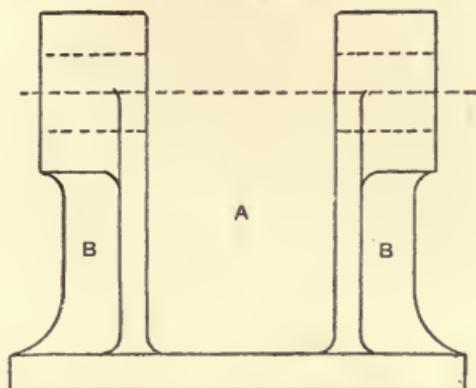
Fig. 145.—Double Bracket Casting.
