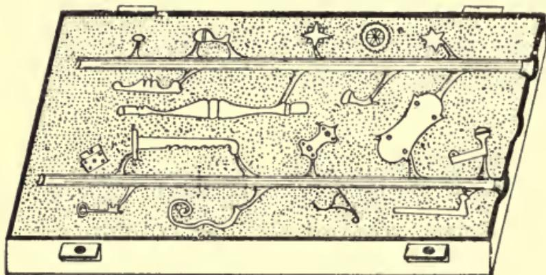
Fig. 19.—Arrangement of Runners in Mould.
