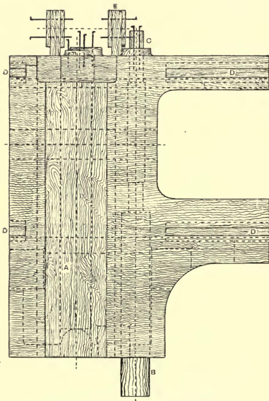
Fig. 251.—Plan of Slide-rest Saddle Pattern.
