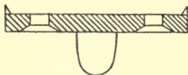
Fig. 30.—Section of Metal Peg Dowel.
