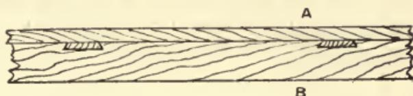
Fig. 212 —Fitting Bearers with Dovetails.
