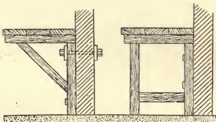
Fig. 17.—Ramming Bench Bolted to Wall.
