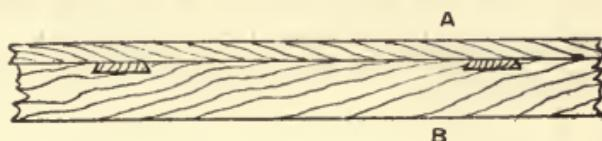
Fig. 212 —Fitting Bearers with Dovetails.
