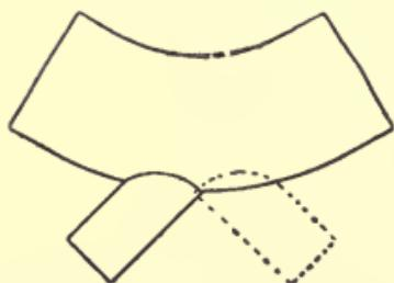
Fig. 86.—Core for Bend-pipe with Branch.
