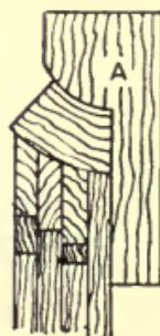
Fig. 191.—Turning Tooth Points by Template.
