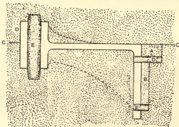
Fig. 122.—Section through Cored Mould.
