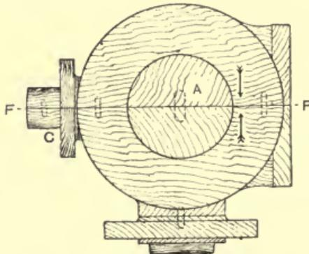
Fig. 97.—Engine Cylinder Pattern.
