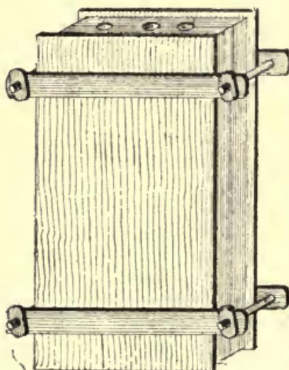
Fig. 7.—Flask ready for Vertical Pouring.
