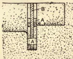
Fig. 140.—Stopping-over Piece in Use.
