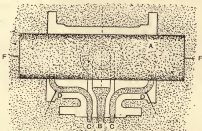
Fig. 98.—Mould for Engine Cylinder.
