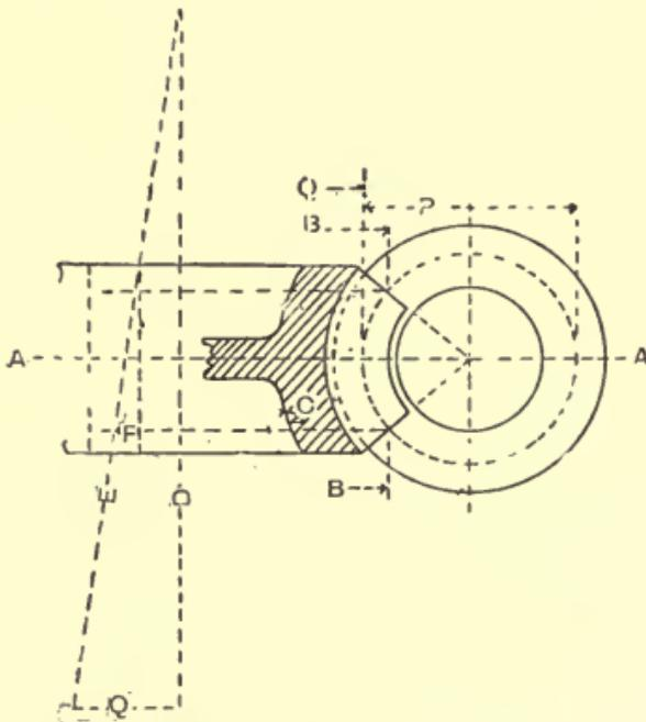
Fig. 184.—Marking Section of Worm Wheel.
