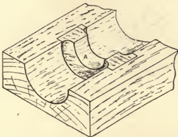
Fig. 76.—Internal Flange Fitted into Core-box.
