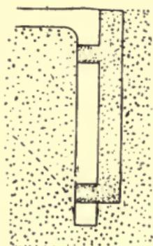
Fig. 123.—Section through Portion of Cored Mould.
