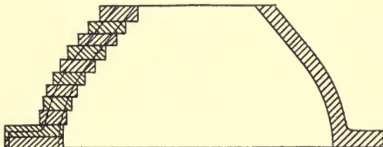
Fig. 63.—Building Pattern of Varying Section.
