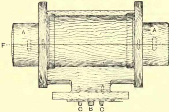
Fig. 96.—Engine Cylinder Pattern.
