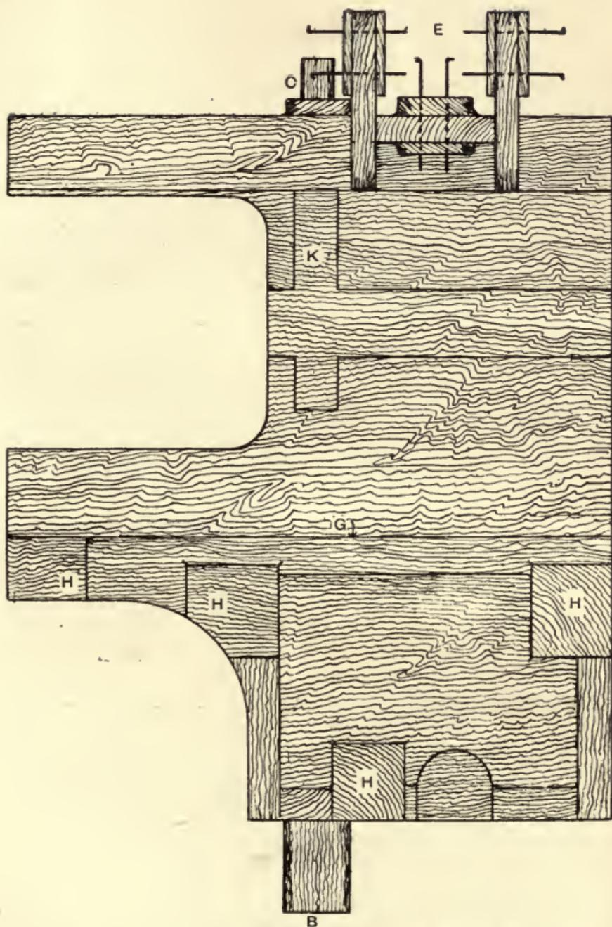
Fig. 252.—Underneath Plan of Slide-rest Saddle Pattern.
