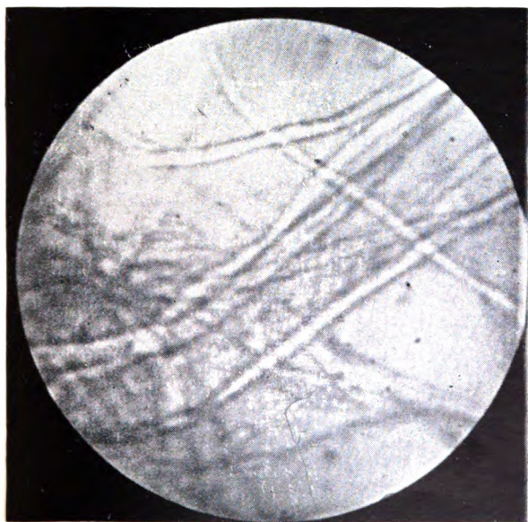
FIG. 12.—MANILLA AND COTTON \times 122 .
