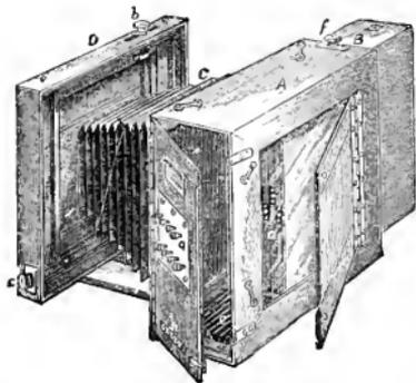
SINCE the introduction of Dry Plates a want has been felt for a Camera that should combine in itself an arrangement for holding several plates, permitting of their exposure being made in rotation, thus avoiding the cumbersomeness and inconvenience of several extra dark slides or backs, and which shall be also of light weight, yet strong and rigid.
