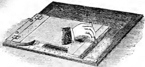
No. 2. For cutting glass photographic sizes from  $\frac{1}{4}$ -plate up to  $10 \times 8$ . A rule, a movable stop, and a firm straight edge for the diamond to work on, form the simple means of this time and labour-saving instrument.
