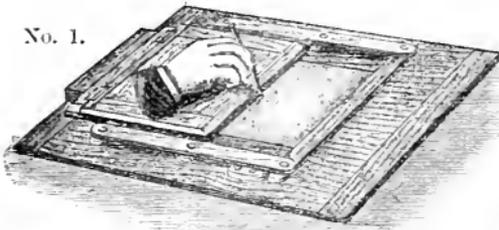
No. 1. For centring and cutting glass. Any piece put on the Board can be immediately cut exactly into half. For Dry-Plate work it is a great economiser of time.
