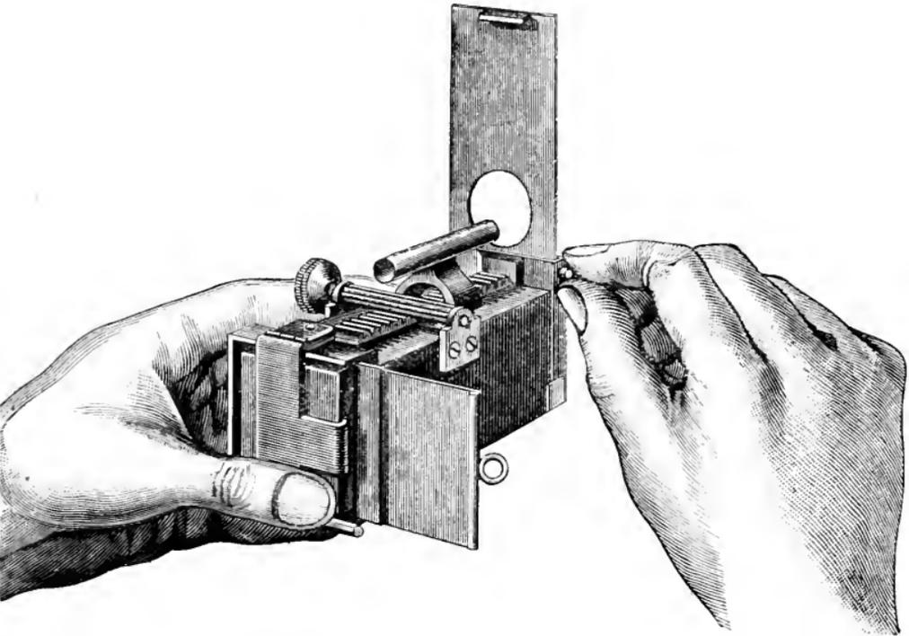
the inverted image on the ground glass. Also that the shutter is a drop instead of a revolving one. This makes sheeling of the camera less likely. Lastly, that instead of the plates being carried in the apparatus, they are carried in small separate shutters, of which the photographer may carry any number he pleases. By this arrangement the bulk of the apparatus actually to
