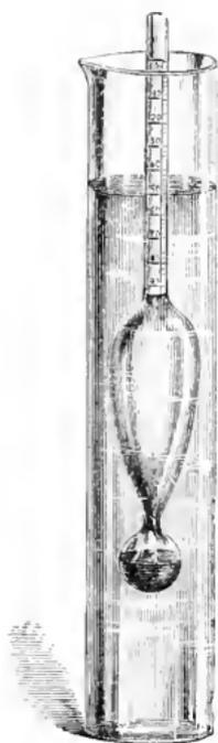
a sufficient degree of correctness, how many grains of silver nitrate there are to each ounce of solution. An argentometer is usually provided with a tall glass vessel, which will hold just enough solution to float it.
