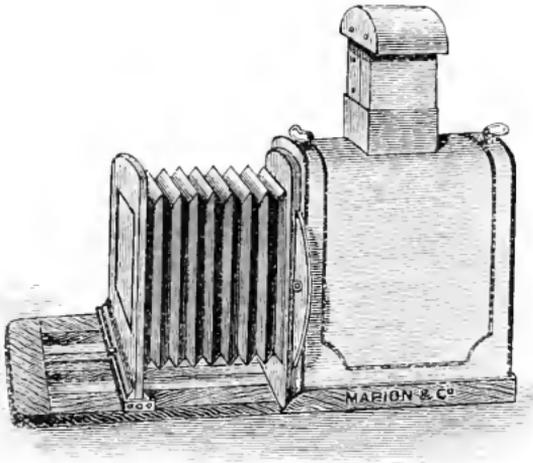
in the engraving, but any photographic lens of suitable focus will do well. A portrait lens, or one of the rapid type of about six or seven inches equivalent focus, will be found the best.
