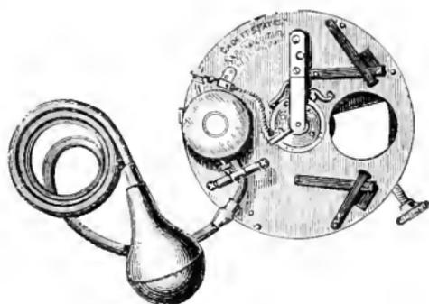
second to any longer period of time without limit, and these results are obtained by the simplest of means;—a revolving ebonite disc, worked by a coiled spring in the centre, two catches, and with Cadett's pneumatic apparatus. Five minutes' careful inspection will enable any one to work it.
