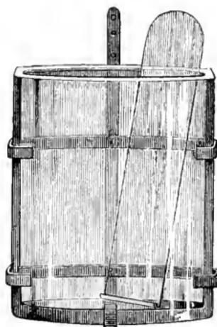
simply a vertical vessel so shaped as to hold a plate surrounded with solution. The best material is glass. The dipper is a little piece of apparatus for lowering a plate into the bath.
