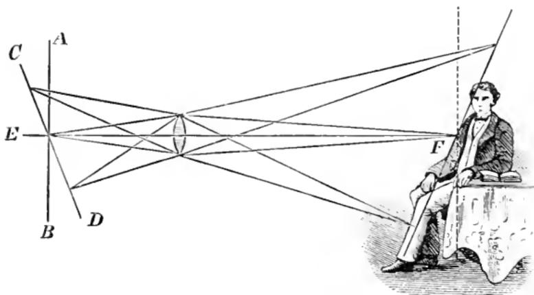
the lens, the rays of light coming from the head would focus in front of it, those coming from the feet would focus behind it. If, however, we *swing* the ground glass so as to occupy the position  $C D$ , then both the rays from the head and the feet will come to a focus approximately upon it.
