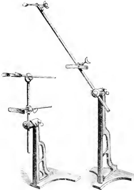
The frame is made of cast-iron so as to be heavy and give a sufficient support. There is an adjustable piece for the waist and another for the head.
