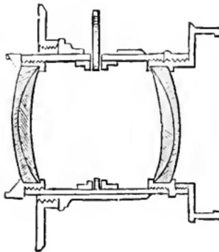
*The Rapid Rectilinear or Rapid Symmetrical Lens.*
