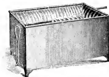
This Apparatus offers all the desiderata for a complete and thorough wash to the Plates. The water falls in a gentle shower; when nearly full the overflow syphon begins to work, so there will be a constant inflow and outflow. When the water is turned off the syphon sucks out the last drop, thus there is no fear of Hypo deposit remaining.
