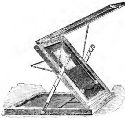
that it consists essentially of a framework or desk at which the retoucher sits, the negative being so placed that he can see through a portion of it whilst his head is shaded from the light. The negative rests with its lower edge against a slip of wood, so that it can be raised or lowered, or canted to one side or to the other. There
