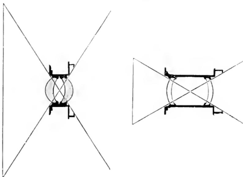
It may be asked, Why not use at all times the wide-angle lens, and simply employ a smaller plate, if we do not wish to include all the angle which it will take in? The reason is this:—The surface of the glasses of a lens which has to include a very wide angle are so ground that even for a narrow angle it will not give definition, unless a small stop be used, and therefore it is at best a slow lens.
