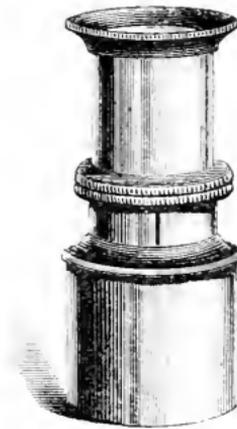
Now we have to select the diaphragm to use. We shall probably perceive that, although the principal object is now quite sharp, neither the distance nor the foreground is so. We place the stop with the largest aperture in position, when we shall perceive a notable improvement on the definition of these parts. We try another and another stop till we get to the one which gives everything *just* sharp. With this we expose.
