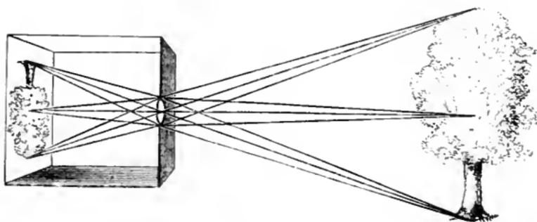
The lens which we show here is the simplest possible, and is one which, although by its means photographs of a kind might be taken, yet is not by any means a very perfect instrument. Still, however complicated a photographic lens may be, its sole object is to produce the
