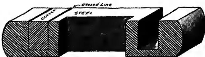
Fig. 65. Cross Section of Fork Handle
