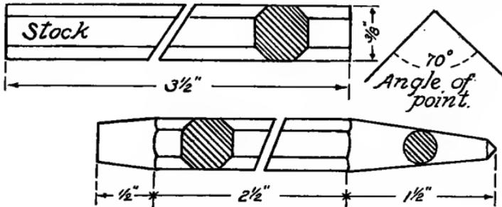
Fig. 120 (above). Center Punch. Fig. 121 (below).
