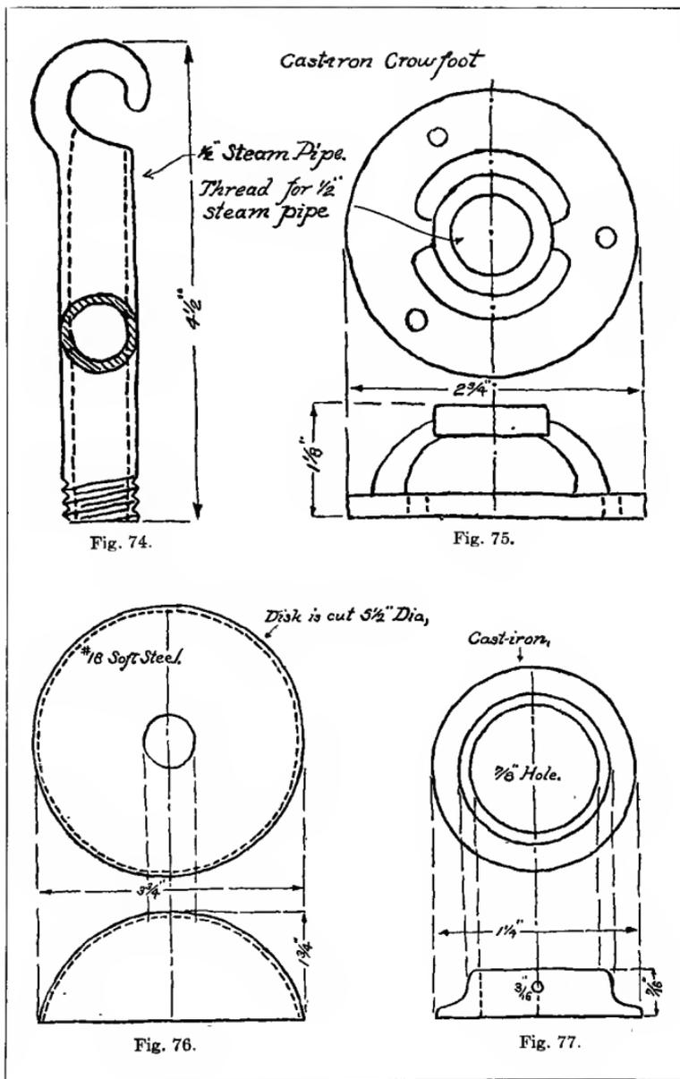
ing cap is necessary. This may be a piece of  $\frac{1}{2}$ -in. steam pipe threaded on one end and a hook made on the other.
