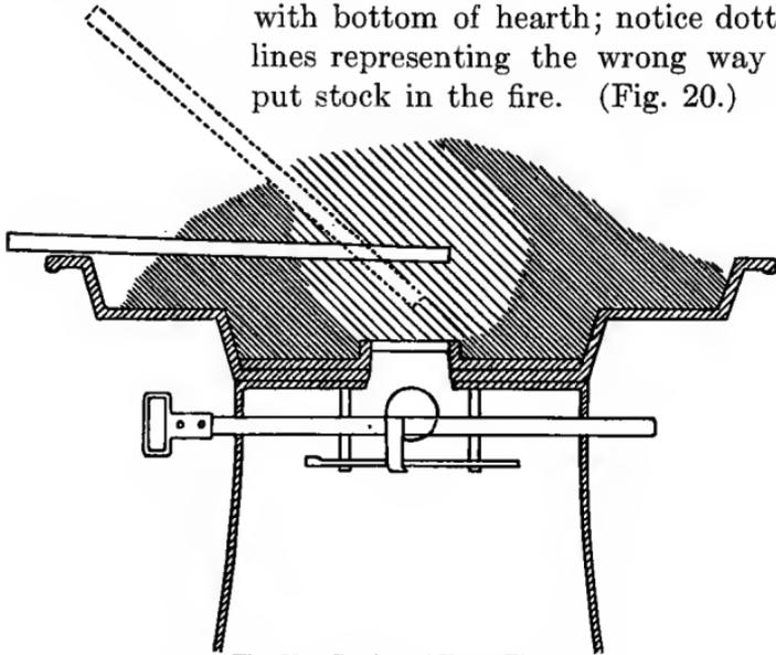
Fig. 20. Section of Forge Fire.
