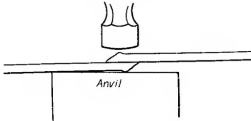
Fig. 115. Welding Thin Steel.
