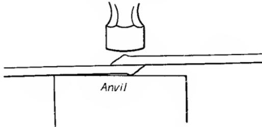
Fig. 115. Welding Thin Steel.
