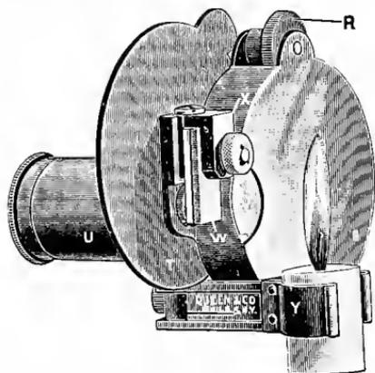
FIG. 161.—Dare's hemoglobinometer. *W*. Blood holder. *R*. Wheel to turn color glass. *V*. Color glass. *U*. Observation tube. *T*. Shade. *Y*. Candle.
