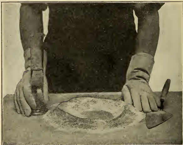
FIG. 50.—Making Briquettes—Adding the Water.
