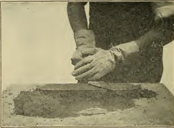
FIG. 54.—Making Briquettes—Troweling the Surface.
