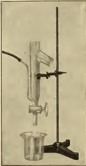
FIG. 29.—Apparatus for Determining Fineness by Washing.
