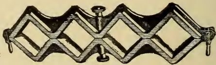
FIG. 111.—Gang Mould for 2-in. Cubes.
