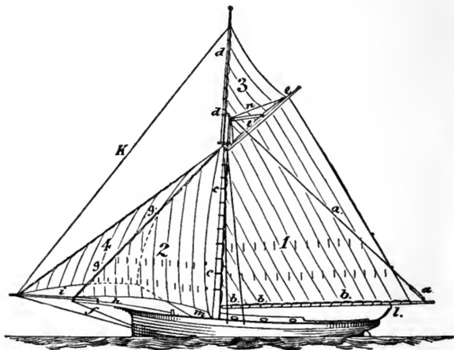
end in a small ball, called the *truck*, through the sides of which are fitted little *sheaves* (i.e., wheels), by means of which, and the use of a small-sized rope, called *signal-halliards*, the flag, or private signal of the boat, is hoisted to the *topmast's* head, and displayed.
