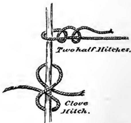
anchor, it is customary to stop the end of the rope down upon the standing part by means of a rope-yarn, so as to prevent all chance of its coming apart whilst chafing about at the bottom of the sea. *A clove hitch* is this same knot made around a spar or other article, instead of on its own standing part. (See diagram.)
