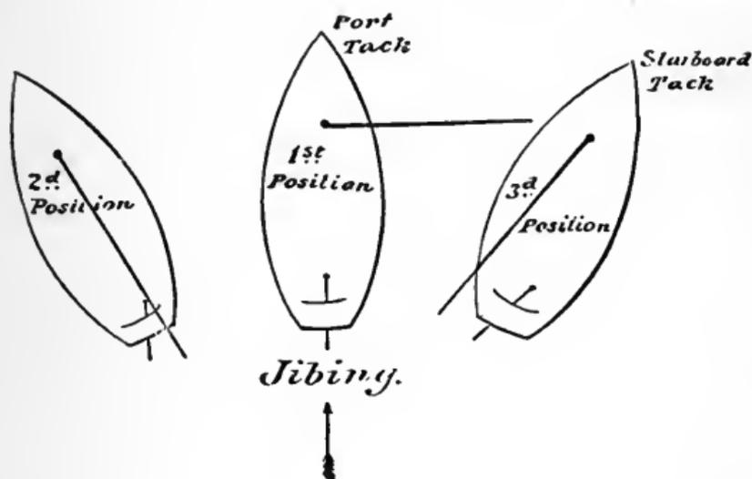
and the main-boom almost amidships ; then take a good turn with it, and shift the helm gradually, till the wind is on the starboard side slightly, and the sail has filled with a slat upon that tack ; when the main-sheet may be slackened, the peak hoisted, and the yacht kept on her course.
