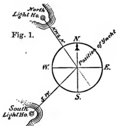
the face of the compass, which is always between the observer and the object to be observed; and line the bearing of this lighthouse by compass, in the same manner, which we will suppose to be S.W. With these two results marked upon pa-
