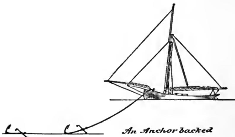
small kedge-anchor, by fastening it by small ropes, passed around the shank and through the ring, to the cable of the large anchor, and cast it over the bows. This is called "backing an anchor" (see diagram), and strengthens the hold of the first anchor in a marked degree, especially if the holding-ground be poor. It is supposed, of course, that, as the yacht comes head to wind, the jib is hauled down ; and now the next thing is to down
