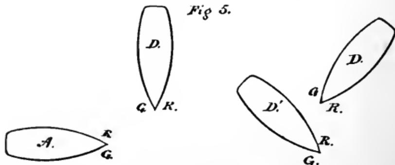
knows that either, first, a vessel is approaching him on his port bow, as B, or, second, a vessel is crossing his bows to port in some direction, as D D' D'' (Fig. 3). If A sees a *white masthead light* above the *red light*, he knows that the vessel is a steamer, and is either approaching in the same direction as B (Fig 2), or is crossing to port in the same direction as D D' D'' (Fig. 3).
