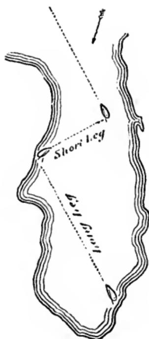
Is the art of putting a yacht about, so that the wind, which has been blowing upon the starboard side, we will say, shall blow upon the port side, or on the opposite side of the sails to which it was before the manœuvre was executed, and, when used to force the vessel by a series of angles towards the direction from which the wind proceeds, is called "beating to windward." Sometimes the wind is not dead ahead, and yet
