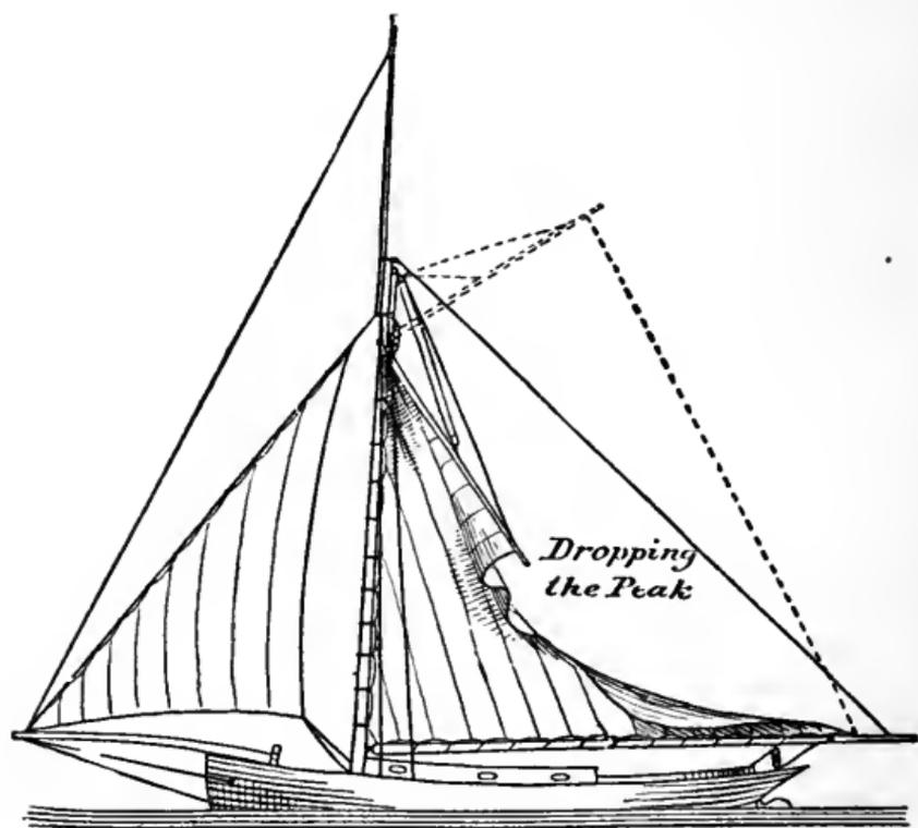
go the peak-halliards of the mainsail, so that the outer clew and head of the sail, that is attached to the gaff, will be lowered down so as to dangle alongside of the mainmast, with the gaff pointing to the deck. This makes of the mainsail, for the time being, a sort of triangular or leg-of-mutton sail, and takes off the leverage of the high part,
