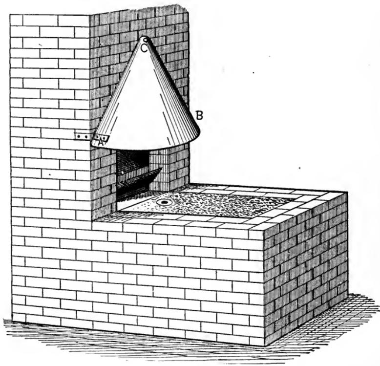
FIG. 19—SHOWING THE HOOD ATTACHED TO THE CHIMNEY.
