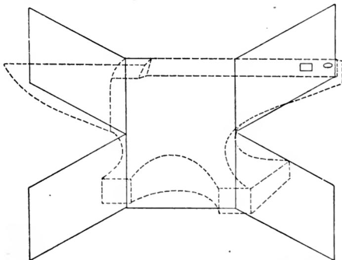
FIG. 73.—SHOWING THE STEEL FULLERED AND FORMED INTO THE OUTLINE OF AN ANVIL.
