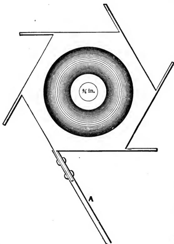
FIG. 200.—CENTER-PIECE TO WHICH FANS ARE ATTACHED.
