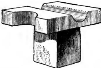
FIG. 122.—THE ANVIL SIDE OR BOTTOM SWAGE.
