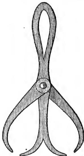
FIG. 86.—THE DOUBLE CALIPERS.
