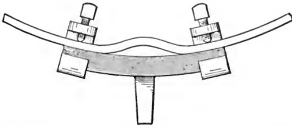
FIG. 155.—SHOWING THE METHOD OF USING THE TIRE-SETTER, NO. 5,
