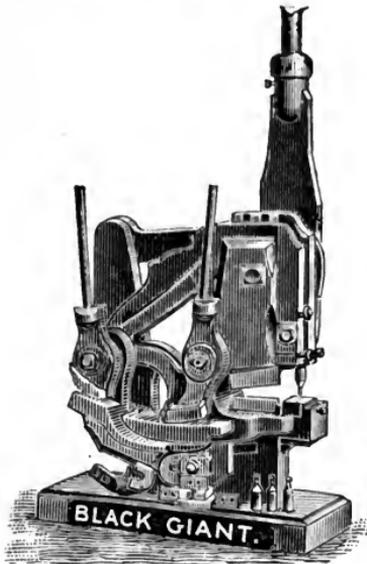
EVERY MACHINE FULLY TESTED before leaving the factory. MAIN BEARINGS are CHILLED, steel gibs in back of slide take up all wear, and WE GUARANTEE them to cut  $\frac{3}{4}$  in. square and round iron and 3 by  $\frac{1}{2}$  inch flat bars. They will punch iron  $\frac{3}{8}$  thick, and will punch  $\frac{3}{4}$  inch hole in BOILER PLATE 5-16 thick, 6 inches from the edge. Has self-adjusting dies and punches.
