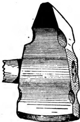
FIG. 4—THE LONG CROSS-FACE HAMMER.
