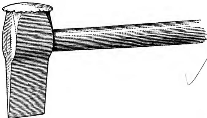
FIG. 109.—THE HOT CHISEL.
