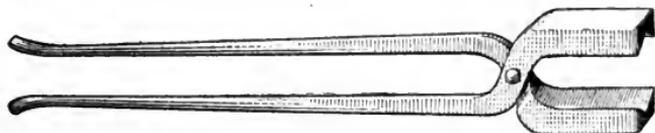
FIG. 99.—FLAT TONGS FOR HOLDING LARGE PIECES.
