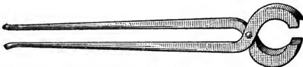
FIG. 101.—TONGS FOR BENDING IRON FLATWISE.
