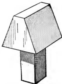
FIG. 163.—A TOOL USED IN MAKING FRENCH CLIPS.
