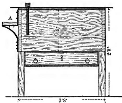
FIG. 42.—SIDE VIEW OF BENCH, SHOWING DIMENSIONS.
