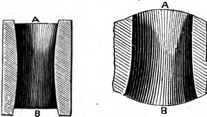
FIGS. 75 AND 76.—CORRECT SHAPE OF EYE FOR TOOL-HANDLE.
