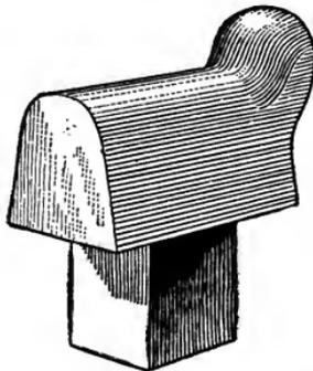
FIG. 124.—THE BOTTOM FULLER.
