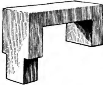
FIG. 138.—SADDLE USED FOR DRAWING OUT FORKED PIECES.
