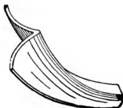
FIG. 170.—SHOWING HOW THE HARROW TOOTH IS BENT.
