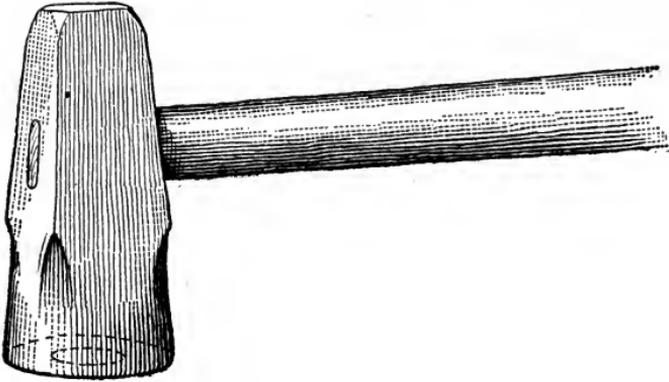
FIG. 117.—THE CUPPING TOOL.
