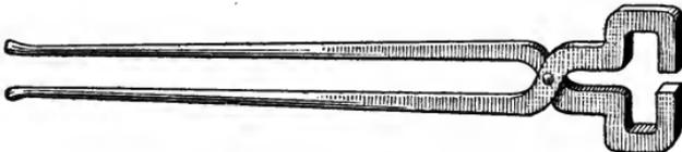
FIG. 102.—TONGS FOR HOLDING PIECES OF DIFFERENT SIZES.
