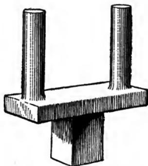
FIG. 130.—A FORK USED IN BENDING.
