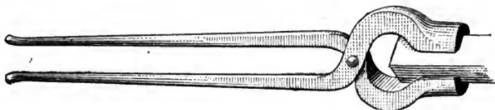
FIG. 98.—TONGS WITH SQUARE, HOLLOW BITS.
