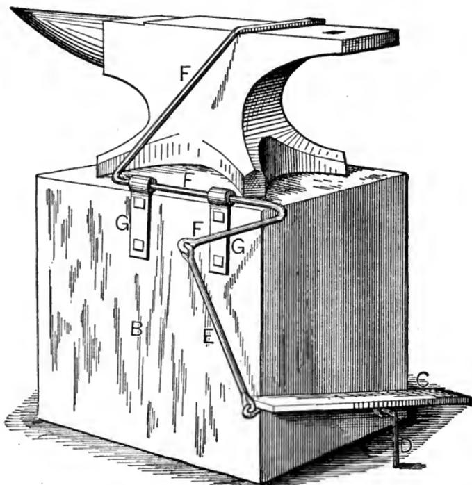
FIG. 58.—DEVICE FOR HOLDING WORK ON THE ANVIL.
