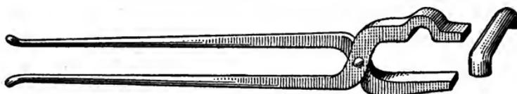
FIG. 94.—TONGS WITH BOX PIECE.
