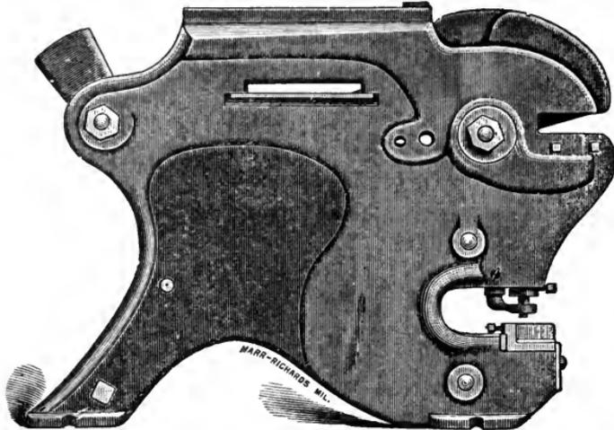
**COMBINED PUNCH AND SHEAR.** for heavy work. Cuts flat Bar  $\frac{1}{2}$  by 4,  $\frac{5}{8}$  by 3,  $\frac{3}{4}$  by 2, 1 inch round or less. Also cuts Plow Steel  $\frac{1}{4}$  by 6. Punches  $\frac{1}{2}$  inch thick—all without any change. Three sets of knives and one punch all independent of each other. Weight, 650 pounds. Punches to center of 8 inches. Price, \$85.00.
