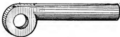
FIG. 167.—SHOWING EYE MADE WITH TOOL NO. 26, FIG. 160.
