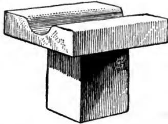
FIG. 120.—THE BOTTOM SWAGE.
