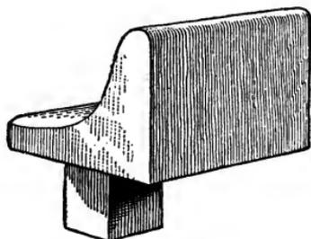
FIG. 132.—A FULLER FOR OFFSET WORK.
