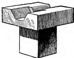
FIG. 134.—A TOOL FOR MAKING BOLTS.
