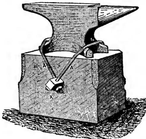
FIG. 62.—METHOD OF HOLDING AN ANVIL IN POSITION.
