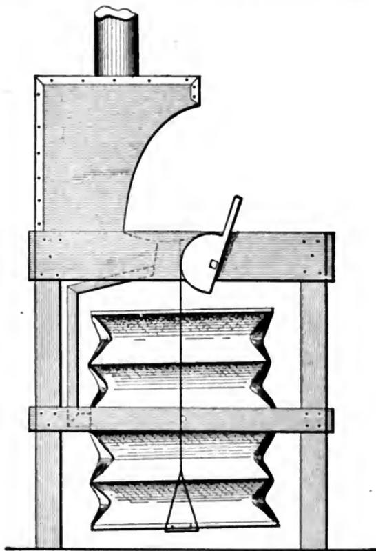
FIG. 48.—HOME-MADE PORTABLE FORGE.
