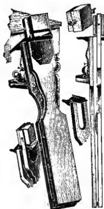
Fig 15—The Daisy foundation fastener.
