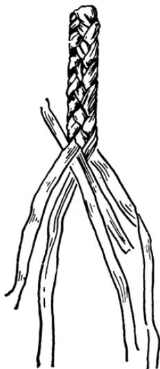
Fig. 34.—Joining Strand.
