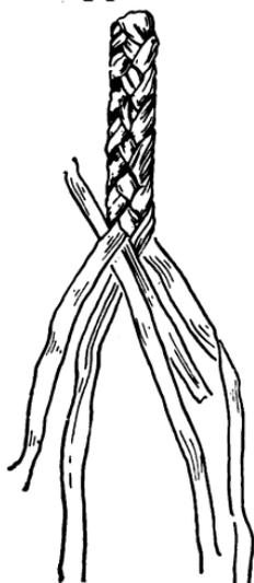
Fig. 34.—Joining Strand.
