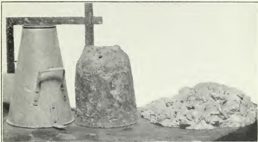
FIG. 1.—MEASURING THE CONSISTENCY OF CONCRETE BY THE SLUMP TEST.
