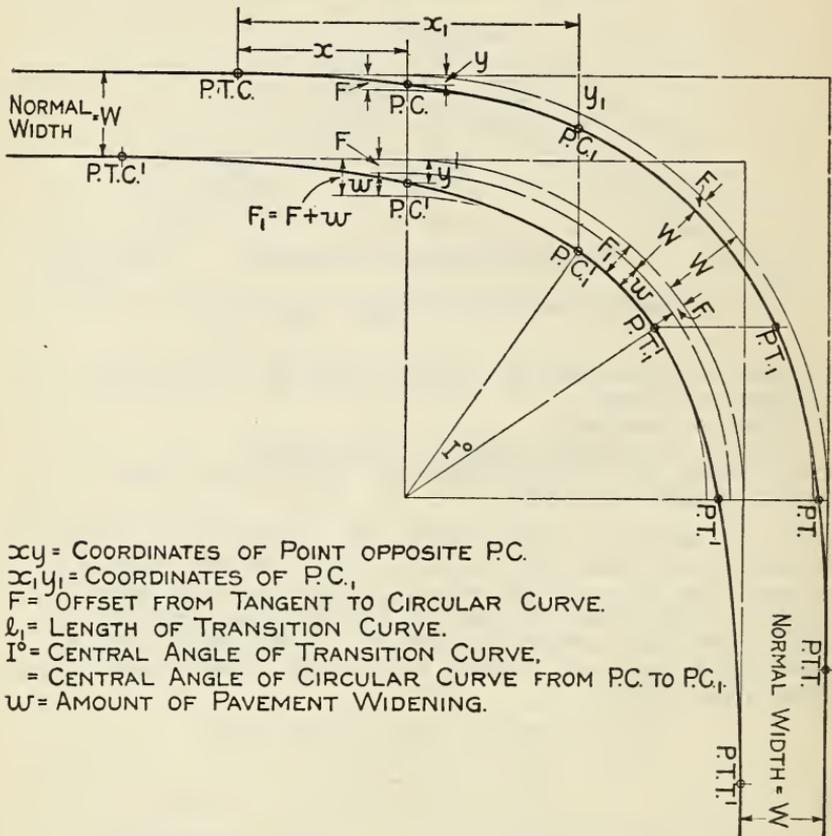
Fig. 5.—Method of widening curves using transition curves.
