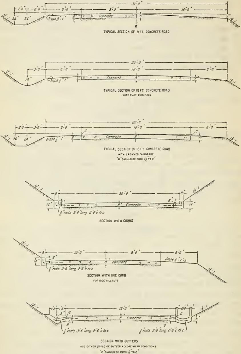
FIG. 7.—Typical pavement cross-sections.
