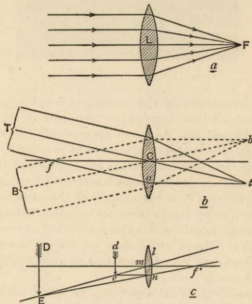
Fig. 5.—SHOWING THE ACTION OF TELESCOPE LENSES.
