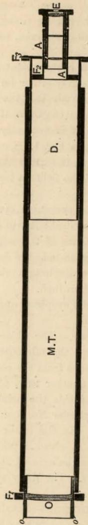
Fig. 2.—SECTION OF TELESCOPE.
