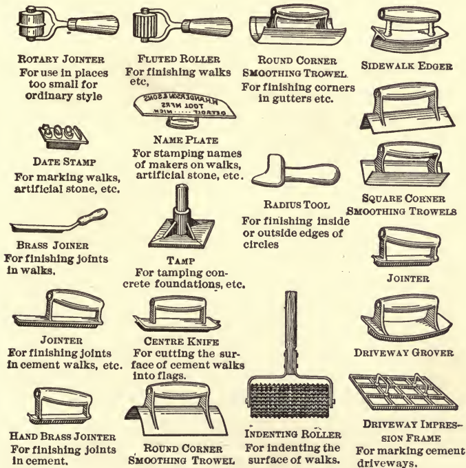
FIG. 103.—Principal Tools Employed in Building Cement Walks.
