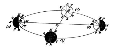
Let E be the Earth's centre, Pp its axis, S the Sun, Kk perpendicular to the plane of the orbit.
