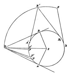
inferior planet, E the Earth: and for simplicity we shall first suppose that the Earth is at rest. Join ES, and draw the tangents EA, EB. The angle AEB is that subtended at the Earth by the orbit of P, and therefore AES or BES is the greatest angular distance from S at which P can be seen from E.
