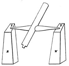
that when it is in perfect adjustment, its line of collimation moves in the plane of the meridian.
