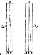
reversing, it will not appear to coincide with it after reversing, for its direction is in the line MO produced, since its image is formed at M, and therefore in the second figure its image will be formed at M, as far from C on the left, as M is on the right. Therefore it is only when the line of collimation coincides with OC, that the same distant object can coincide with the intersection of the lines before and after reversing.
