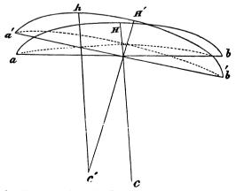
the straight line joining its lower extremities, C the centre of the circle of which ab is an arc; H the highest point.
