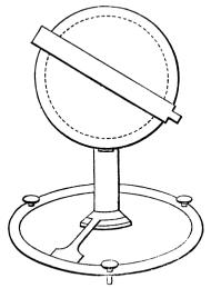
about an axis through its centre, which axis itself revolves about another axis at right angles to it. The latter axis is made to pass through the centre of another circle, to the plane of which it is perpendicular.
