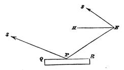
one another and to the angle PEH. Now ES parallel to PS is the direction of the star as seen from E, and by parallel lines the angle HES is equal to QPS, and therefore TES is twice the altitude of the star.
