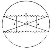
the images of two adjacent lines of graduation are made to lie just at that distance from one another which is passed over by the index in the given number of turns. This adjustment is made by placing the object-glass at a proper distance from the limb, and at such a distance from the eye-glass that the image may be formed in its focus; for the magnitude of the image depends on the distance of the object from the lens, and its distinctness to the eye on its being in the focus of the eye-glass.
