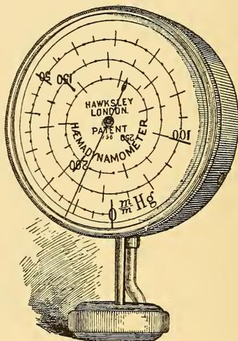
FIG. 72.—Oliver's Haemodynamometer.
