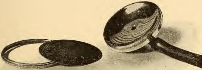
FIG. 87.—Chest Piece of Bowles' stethoscope. On the right the shallow cup communicating with the ear tubes. On the left the diaphragm which covers the cup, and the ring which holds it in place.
