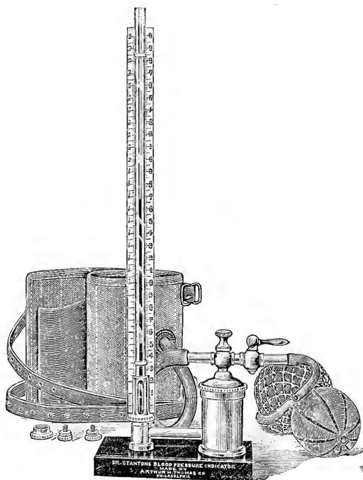
Fig. 122.—Stanton's sphygmomanometer. (From Warfield.)
