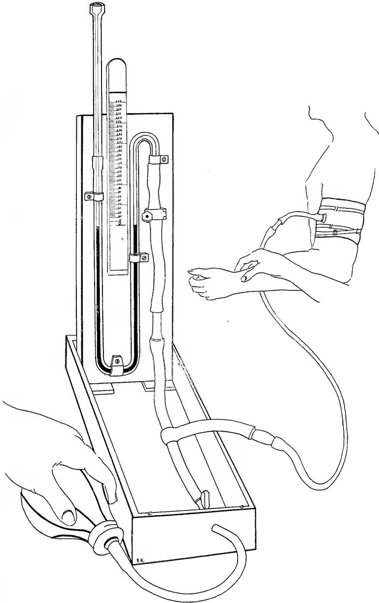
Fig. 124.—The Janeway sphygmomanometer which has been found a convenient and practicable instrument. The scale can be pushed below the level of the top of the box, the long arm of the mercury tube is disjoined and placed in the bottom of the box, the lid is then closed, and the instrument takes up but little space in the physician's bag. (From Warfield.)
