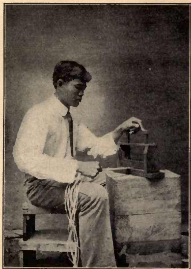
Plate VI. Stripping buri straw with the Andes stripper.
