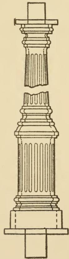
Fig. 270. Completed Column Pattern
