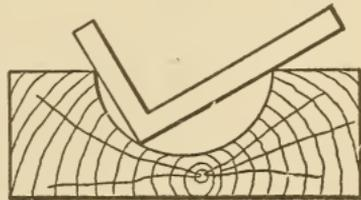
Fig. 143. Right-Angle Test of Circle
