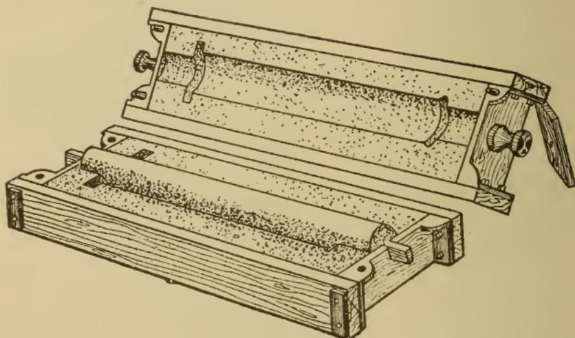
Fig. 365. Pipe Core Set in Mold
