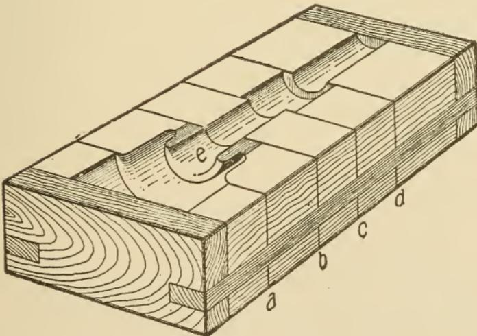
Fig. 239. Core Box for Stuffing Box
