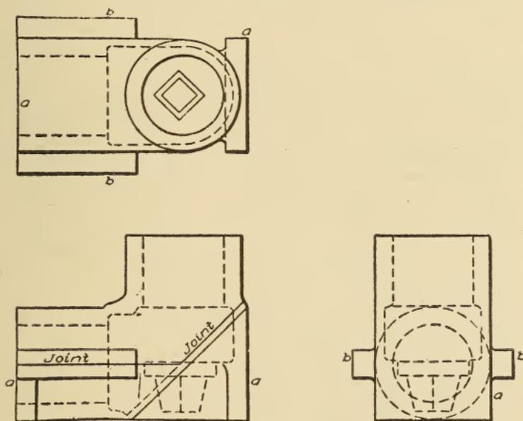
Fig. 233. Upper Iron Core-Box Details
