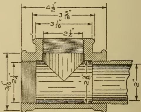
Fig. 202. Section of Tee
