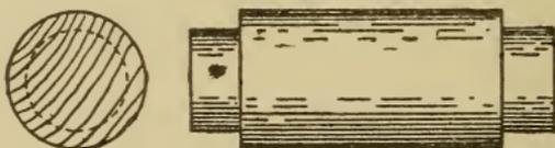
Fig. 111. Solid Pattern for Cylinder
