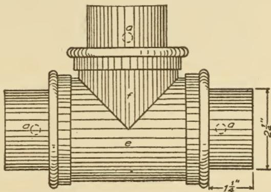
Fig. 203. Elevation of Completed Pattern for Fig. 201
