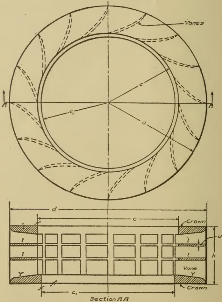
Fig. 272. Plan and Radial Section of Guide Ring
