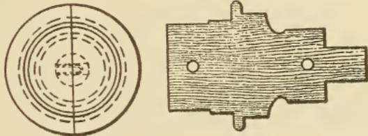
Fig. 238. Pattern for Stuffing Box
