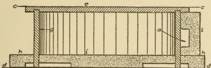
Fig. 131. Section through Vertical Center of Pattern for Fig. 127
