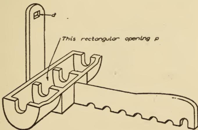
Fig. 341. Sketch of Bearing-Cap Casting
