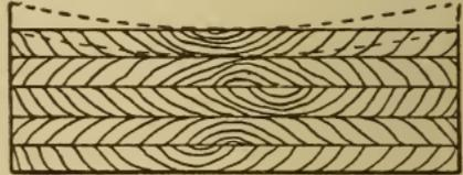
Fig 2 Warping of Pile of Boards
