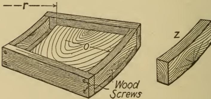
Fig. 283. Core Box for Bottom Core
