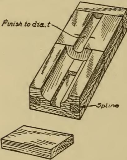
Fig. 322. Core Box for Master Pattern, Fig. 321
