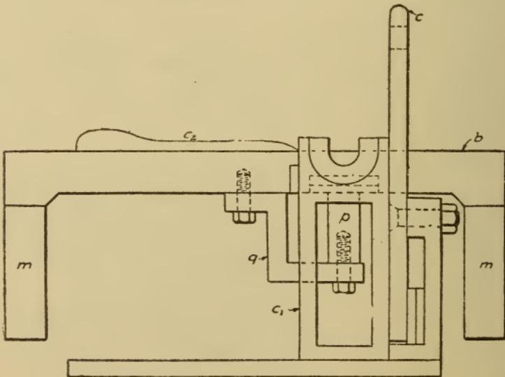
Fig. 351. Nowel End Elevation of Drag Machine
