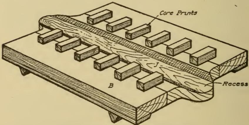
Fig. 334. Pattern for Cope Machine Stripping Plate
