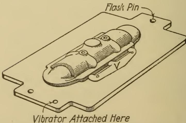
Fig. 295. Completed Plate Pattern
