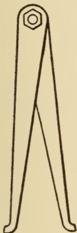
Fig. 71. Inside Calipers
