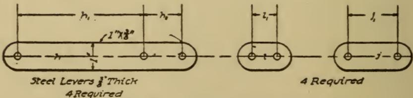
Fig. 325. Machine Steel Lever and Links
