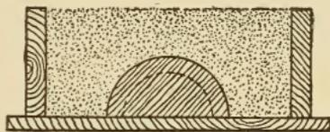
Fig. 108. Starting Split-Pattern Mold
