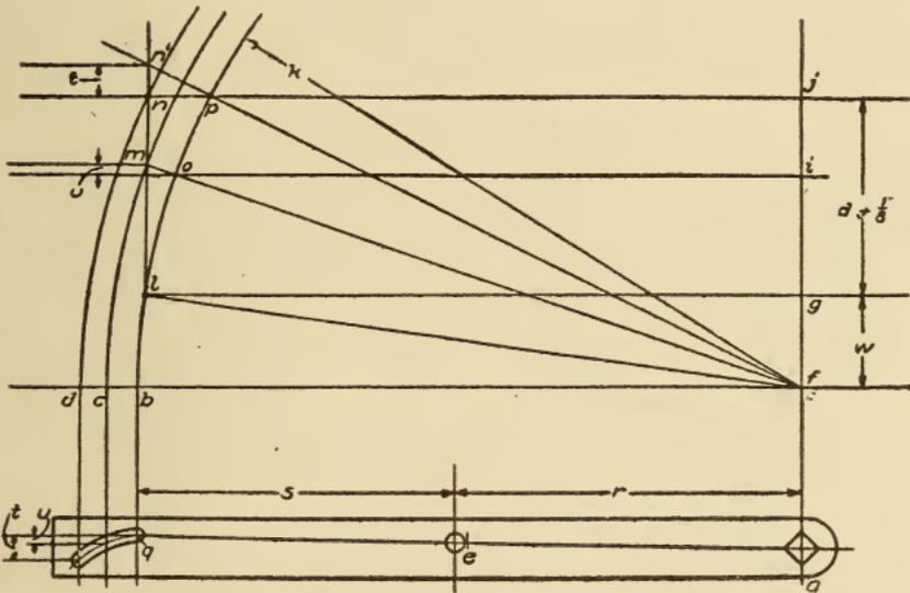
Fig. 305. Layout for Side Arm of Parallel Motion Device
