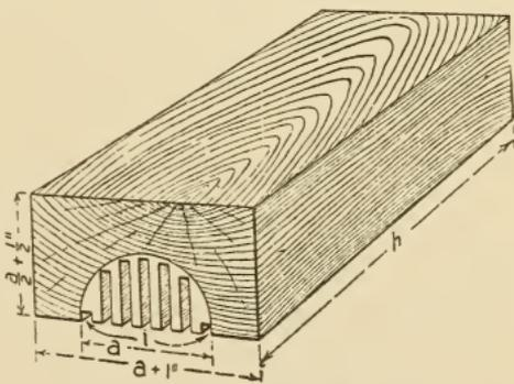
Fig. 147. Method of Removing Waste Stock
