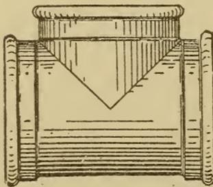
Fig. 201. Tee Pipe Fitting
