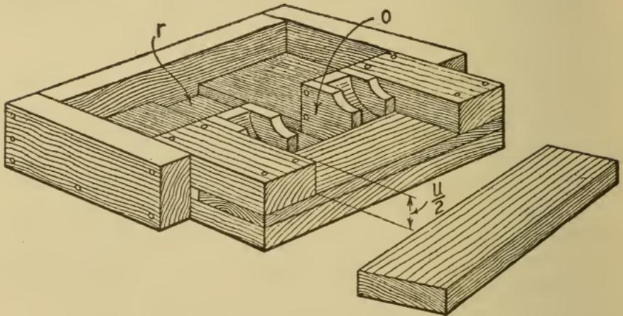
Fig. 350. Core Box for Pattern, Fig. 349
