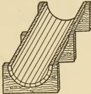
Fig. 227. Typical Core-Box Construction
