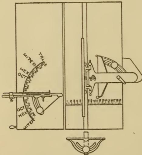
Fig. 96. Plan of Saw Table
