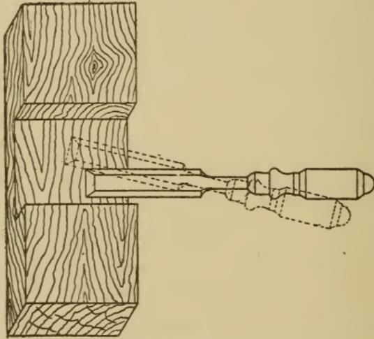
Fig. 43. Method of Using Chisel
