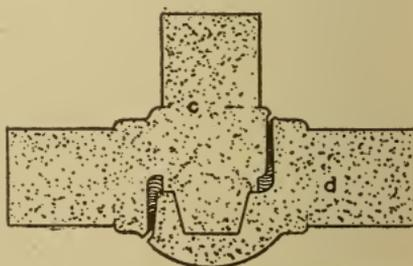
Fig. 236. Sectional View of Dry-Sand Core
