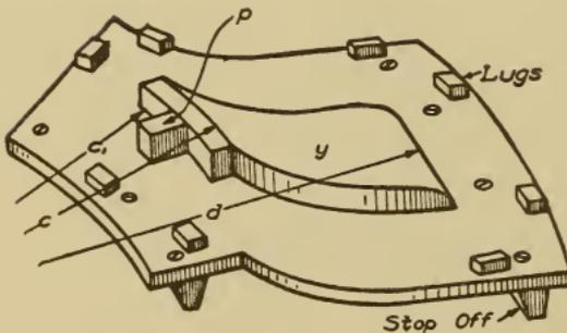
Fig. 279. Bottom of Vane Core Box
