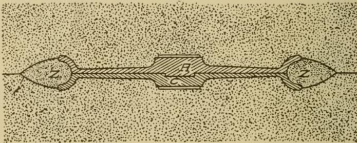
Fig. 123. Green-Sand Ring in Split-Pattern Mold
