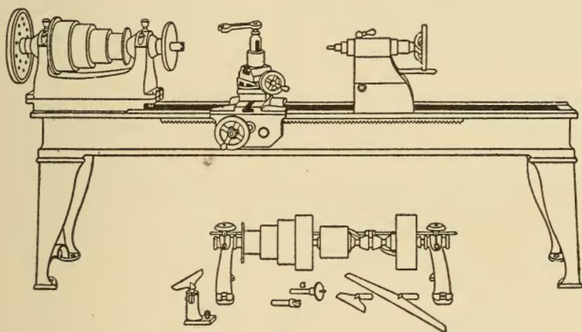
Fig. 87. Pattern Maker's Lathe
