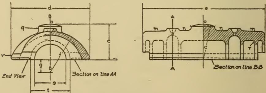
Fig. 288. Working Drawing of Cap for Hanger Bearing
