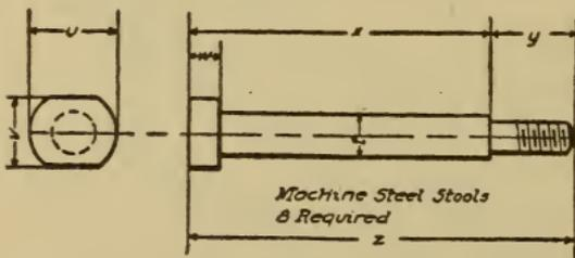
Fig. 324. Drawing of Steel Stool, Fig. 323
