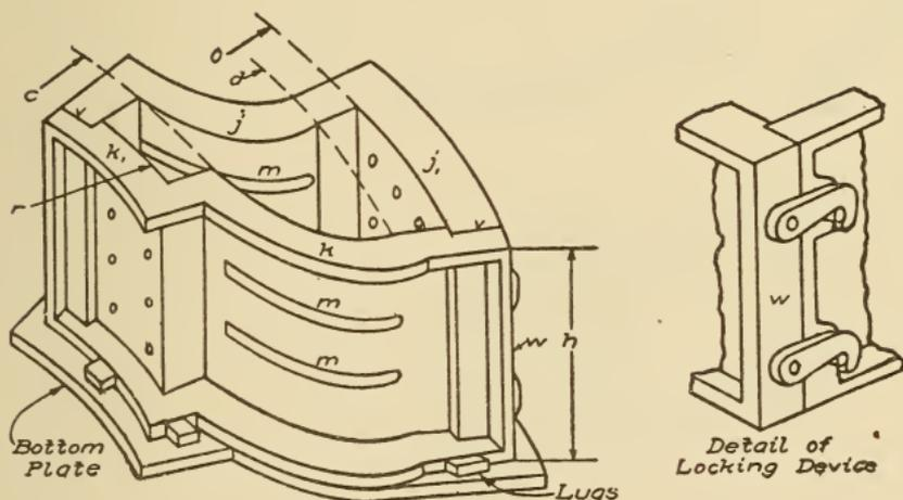
Fig. 275. Diagram of Completed Iron Core Box
