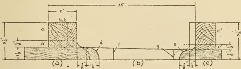
Fig. 187. Construction Diagram for Arm Pattern
