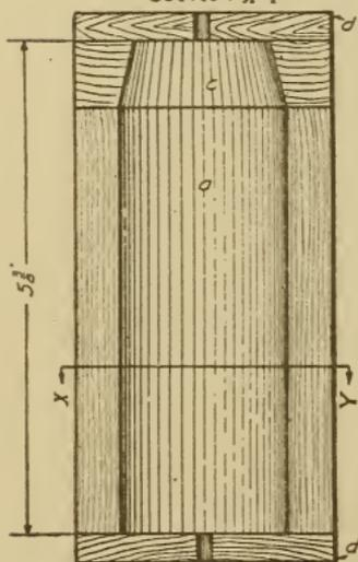
Fig. 140. Core Box for Bronze Bushing of Fig. 13S
