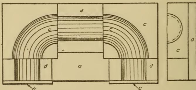
Fig. 213. Construction of Core Box for Elbow Fitting
