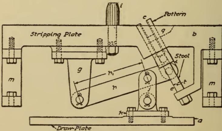
Fig. 312. End Elevation of Pattern Equipment for Reid Hand-Rammed Stripping-Plate Machine
