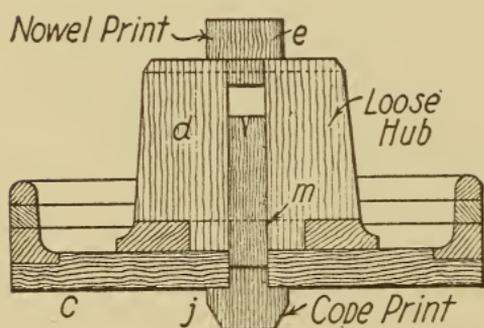
Fig. 297. Section of Hand-Molded Pattern—Loose Hub and Prints
