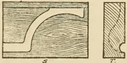
Fig. 250. Exhaust Port Core Box
