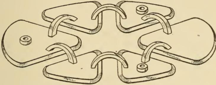
Fig. 181. Assembled Lifting Plate for Six-Arm Pulley
