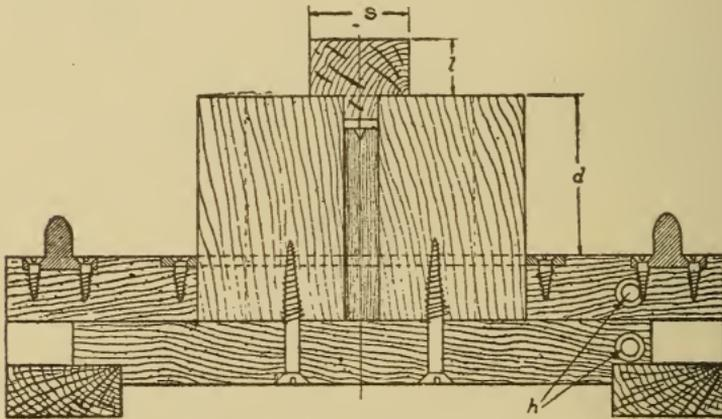
Fig. 304. Section Showing Loose Nowel Core Print
