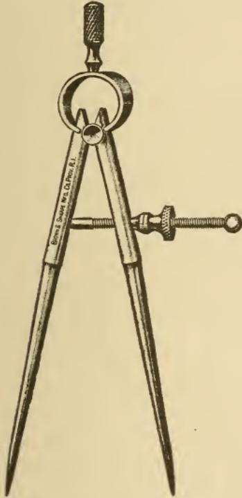
Fig. 65. Brown and Sharpe Spring-Joint Dividers
