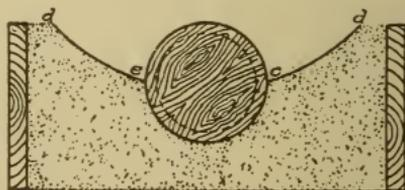
Fig. 113. Coped-Out Mold for Solid Patterns
