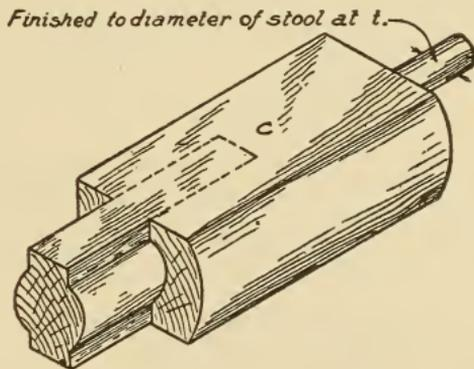
Fig. 321. Master Pattern for Part *c*
