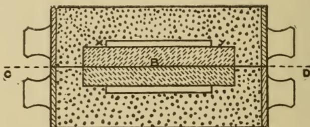
Fig. 110. Completed Mold with Core in Place
