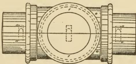
Fig. 204. Plan View of Completed Pattern for Tee
