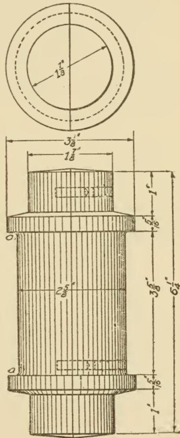
Fig. 151. Pattern for Bushing, Fig. 150
