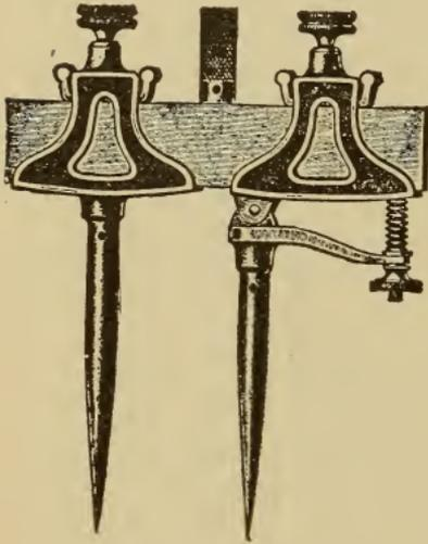
Fig. 67 Trammel with Adjustable Points
