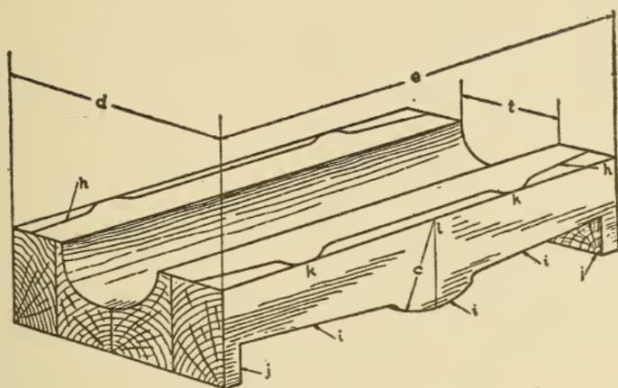
Fig. 289. Partially Completed Stock for Cap Pattern
