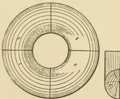
Fig. 211. Method of Turning Up Elbows
