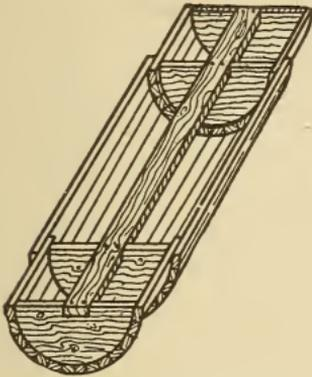
Fig. 226. Slightly Heavier Construction for Cylinder Pattern
