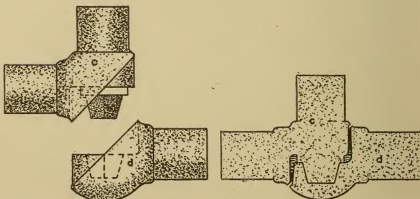
Fig. 235. Dry-Sand Cores before Pasting Together
