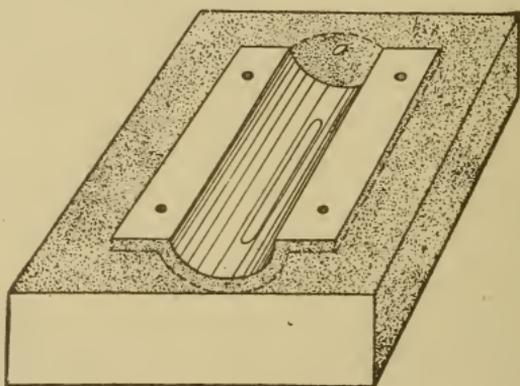
Fig. 119. Coped-Out Mold for Cap
