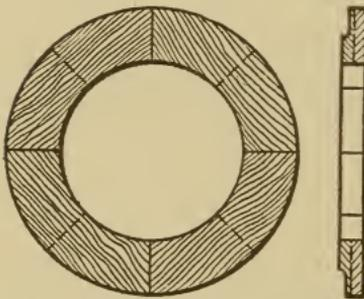
Fig. 247. Built-Up Flange for Cylinder Pattern
