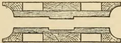
Fig. 165. Section Showing Joint of Sheave Pattern
