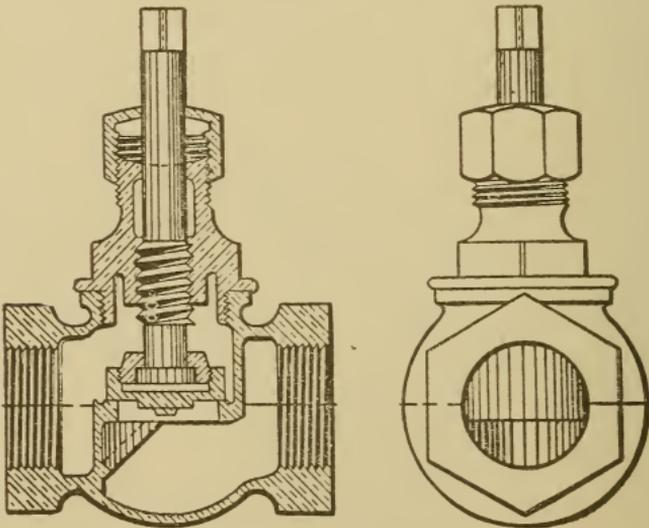
Fig. 229. Section of Globe Valve
