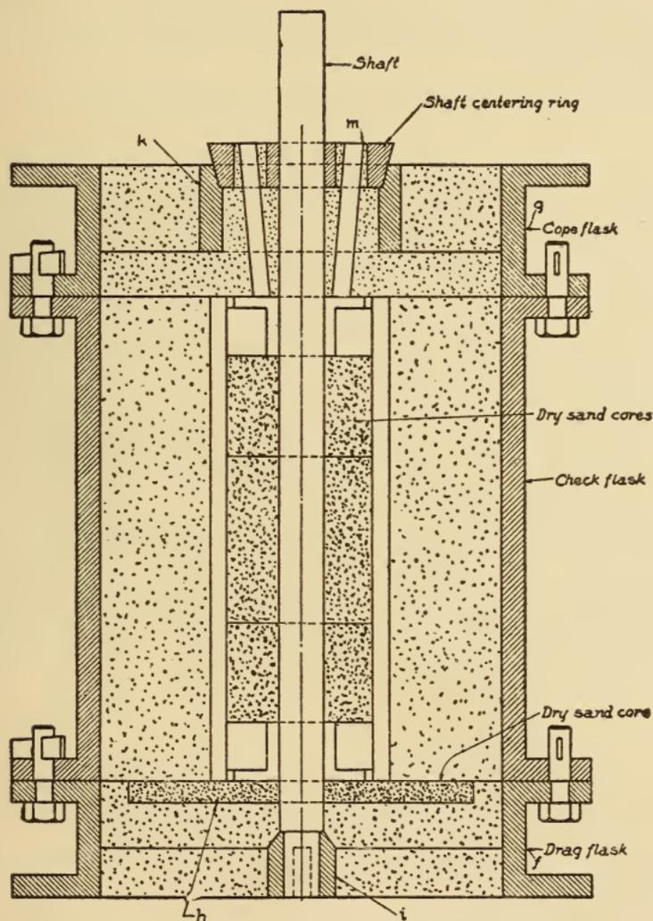
Fig. 384. Section of Complete Mold
