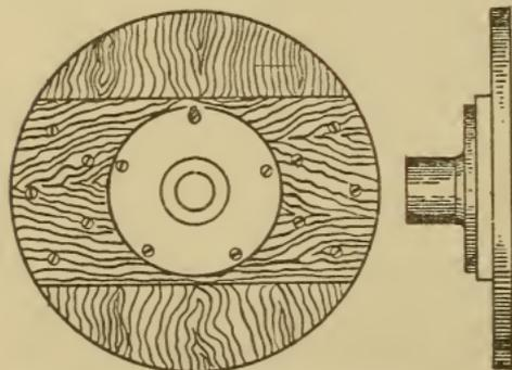
Fig. 89. Medium-Sized Faceplate Construction
