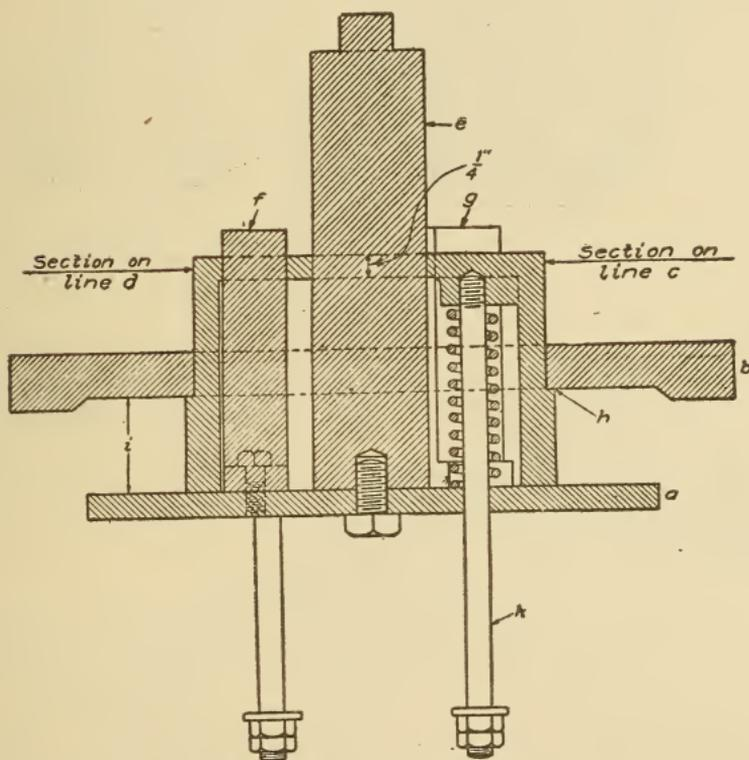
Fig. 360. Section of Pattern, Stripping Plate, and Draw Plate for Casting, Fig. 359
