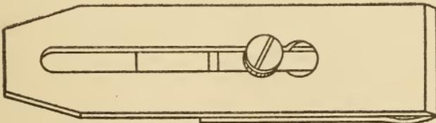
Fig. 23. Plane Iron—Cap Iron Connection
