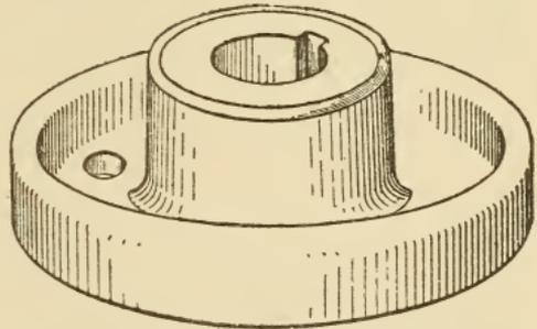
Fig. 296. One-Half of Complete Flange Coupling
