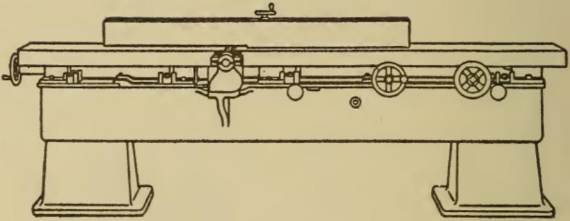
Fig. 100. Hand Planer and Jointer
