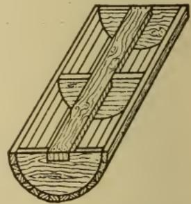
Fig. 225. Light Pattern Construction for Cylinder
