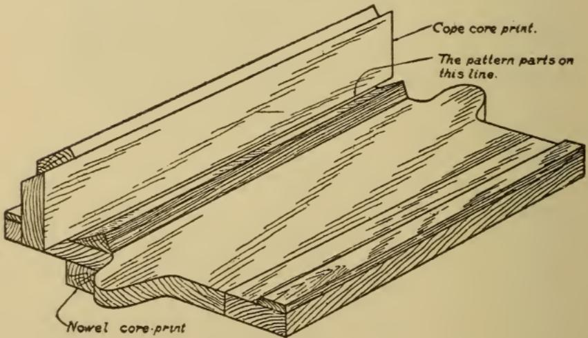
Fig. 315. Pattern for Stripping Plate
