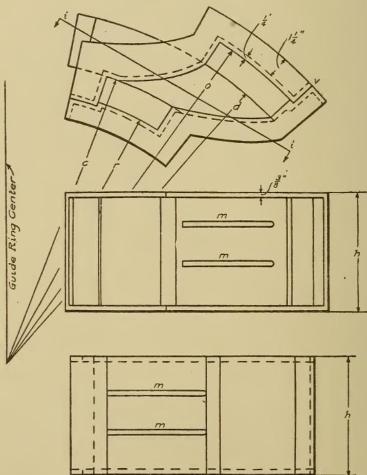
Fig. 274. Plan and Elevations of Iron Core Box
