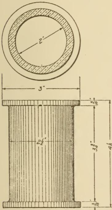
Fig. 150. Finished Bronze Bearing Flanged at Both Ends
