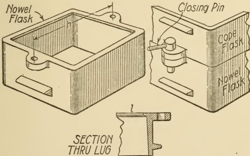
Fig. 301. Sketches of Cast-Iron Flask Showing Closing Pins
