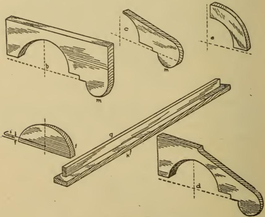
Fig. 369. Ends, Flanges, and Hinge Lugs
