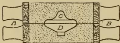
Fig. 104. Flask Showing Parting
