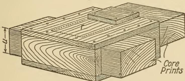
Fig. 349. Master Pattern for Part *c*<sub>1</sub>, Fig. 348
