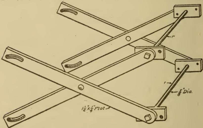
Fig. 306. Details of Parallel Motion Device
