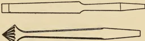
Fig. 53. Brace Screwdriver and Countersink
