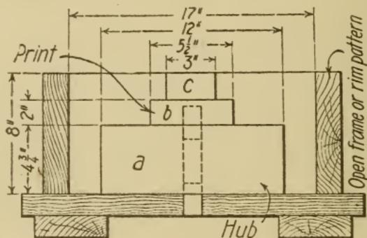
Fig. 188. Section of Hub Core Box
