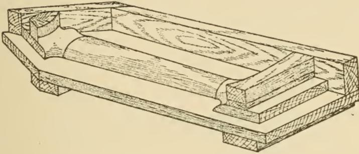
Fig. 186. Core Box for Arm
