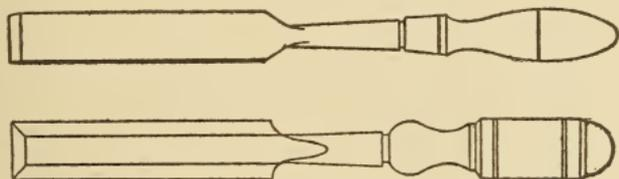
Fig. 41. Socket-Handled Chisels
