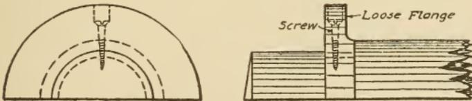
Fig. 223. Interchangeable Flanges on Pipe Pattern
