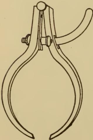
Fig. 69. Wing Calipers
