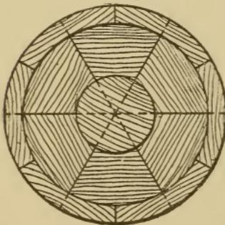
Fig. 162. Web with Rim Glued On
