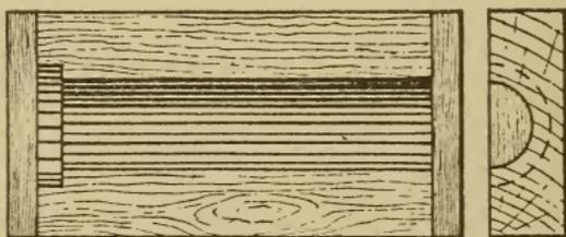
Fig. 219. Core Box for Lathe Chuck Pattern
