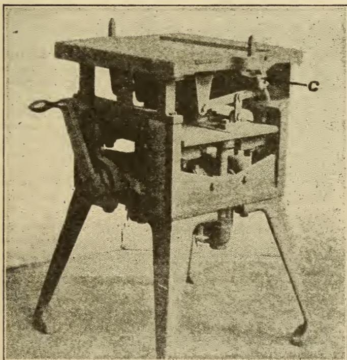
Fig. 310. Nowel or Drag Stripping-Plate Hand-Rammed Molding Machine
