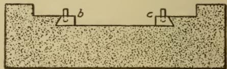
Fig. 126. Loose Pieces in Mold
