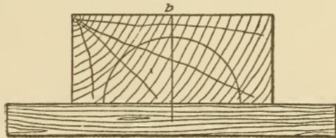
Fig. 142. Layout of Box before Gouging Cylindrical Section
