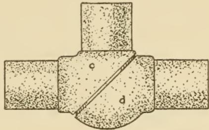
Fig. 237. Assembled View of Dry-Sand Core
