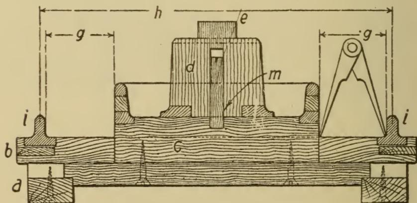
Fig. 299. Section through Center of Nowel Mold Machine
