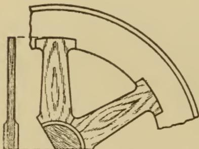
Fig. 263. Part of Arm Pattern for Miter Gear
