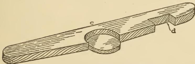
Fig. 353. Master Pattern of Part  $c$ , Fig. 352
