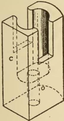
Fig. 320. Casting for Pattern *c*, Fig. 312
