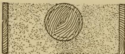
Fig. 112. Solid Pattern Rammed in Drag
