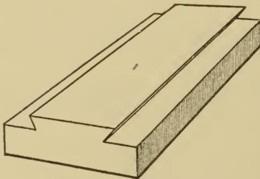
Fig. 124. Dovetailed Slide
