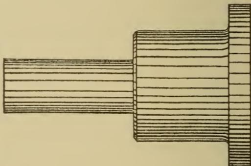
Fig. 218. Appearance of Pattern of Lathe Chuck
