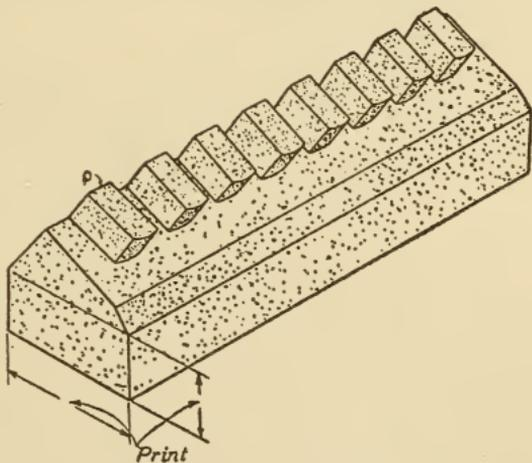
Fig. 317. Dry-Sand Core for Making Holes in Stripping Plates through Which Pattern Is Drawn
