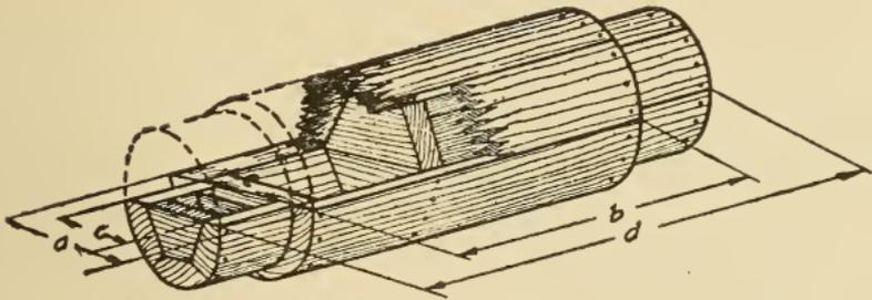
Fig. 373. Split Pattern for Cast-Iron Roll
