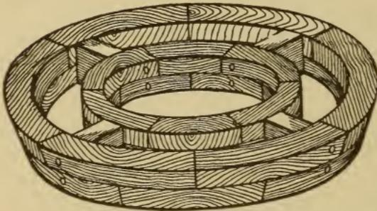
Fig. 382. Pattern for Centering Ring
