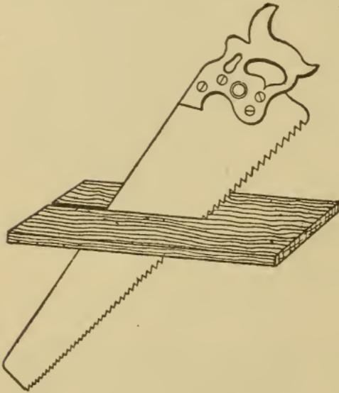
Fig. 11. Position in Ripping
