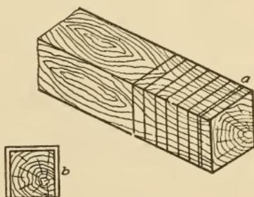
Fig. 18. Example of Back Sawing
