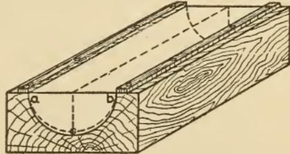
Fig. 37. Protection of Edges in Forming
