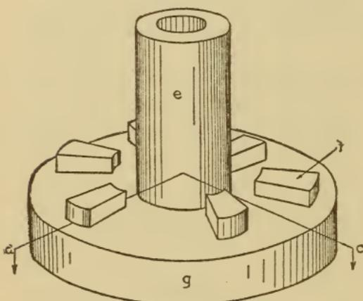
Fig. 359 Casting Molded on Double-Draw Stripping-Plate Machine
