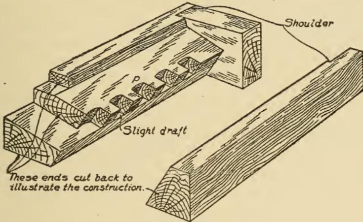
Fig. 316. Core Box for Core, Fig. 317
