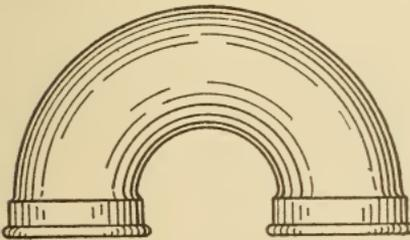
Fig. 215. Return-Bend Pipe Fitting
