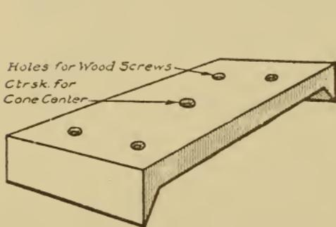
Fig. 206. Steel Center Plate
