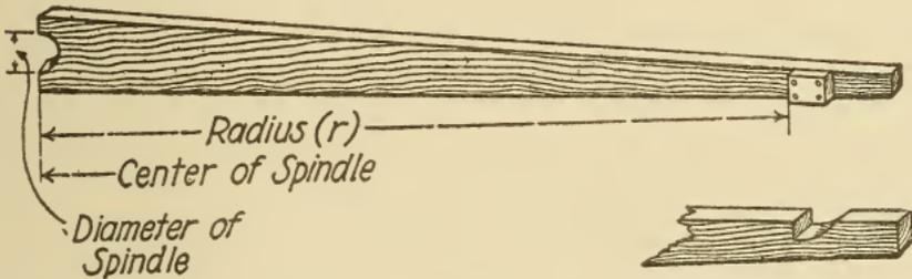
Fig. 285. Gage for Setting Bottom Cores
