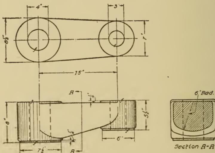
Fig. 192. Detail Drawings for Heavy Engine Crank
