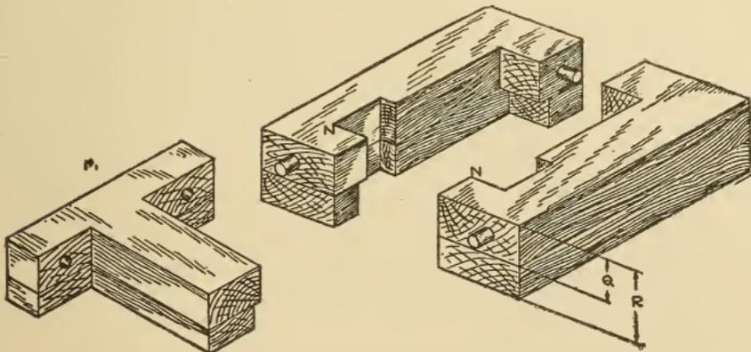
Fig. 337. Core Box for Stripping Plate
