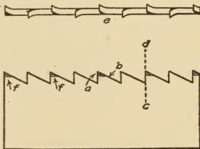
Fig. 10. Teeth of Rip Saw
