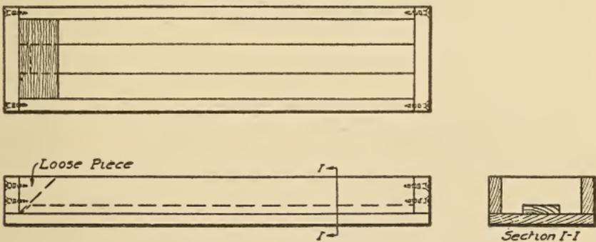
Fig. 281. Details of Core Box for Gate
