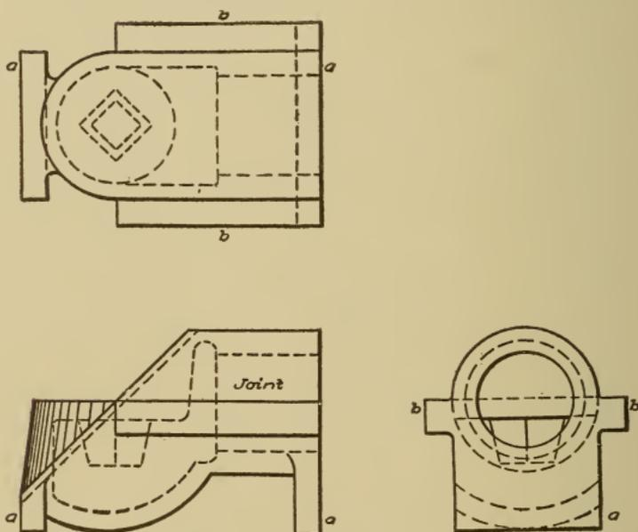
Fig. 234. Lower Iron Core-Box Details
