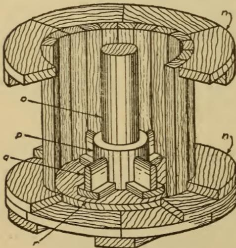
Fig. 383. Core Box for Arm Mold
