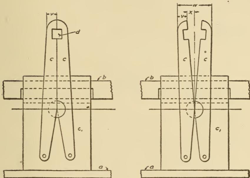
Fig. 352. Expanding or Crush-Back Motion
