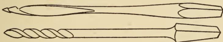
Fig. 52. Gimlet and Wood Drill
