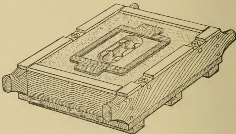
Fig. 294. Drag Mold of Cap for Hanger
