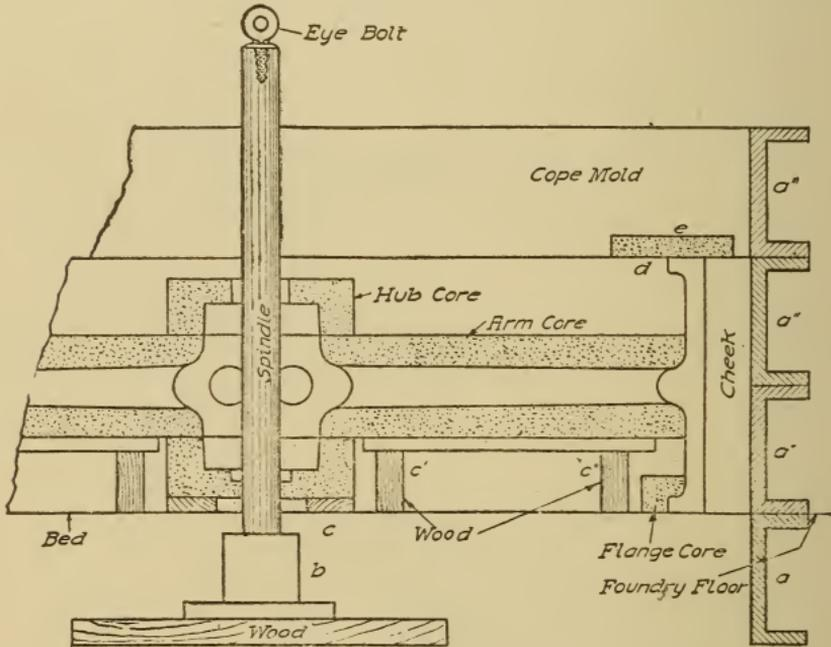
Fig. 191. Section of Cored-Arm Pulley Mold
