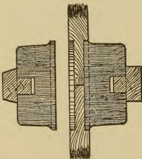
Fig. 176. Section through Center of Arm Hub and Core Prints. Novel Hub Glued to Arms; Cope Hub Loose
