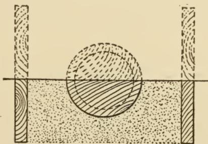
Fig. 109. Position for Molding Cope
