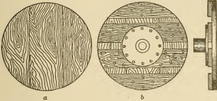
Fig. 90. Strongly Braced Faceplate for Large Work
