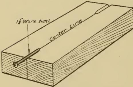
Fig. 152 Preparing Stock for Split Lathe Work
