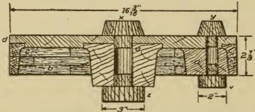
Fig. 195. Section of Pattern for Disk Crank
