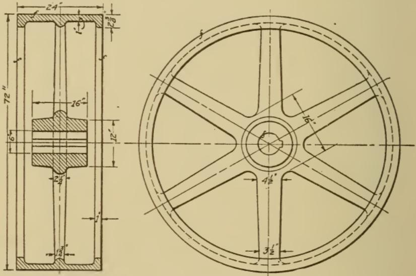
Fig. 185. Dimensions of Cored-Arm Pulley
