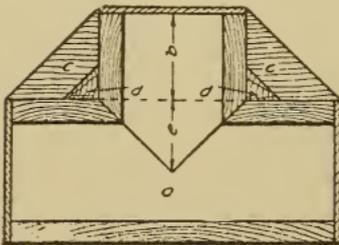
Fig. 208. Core Box for Tee
