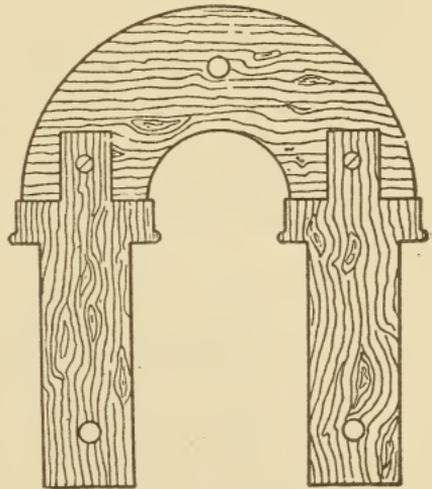
Fig. 216. Section of Pattern for Pipe Fitting
