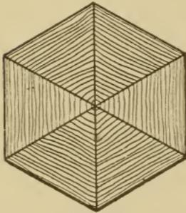
Fig. 161. Segmental Construction of Web for Sheave Pattern
