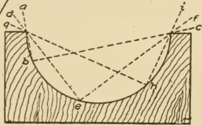
Fig. 35. Profile Cut by Core-Box Plane
