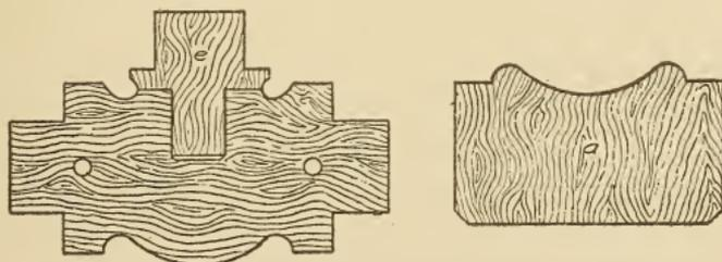
Fig. 232. Sectional View of Pattern and Template for Globe Valve
