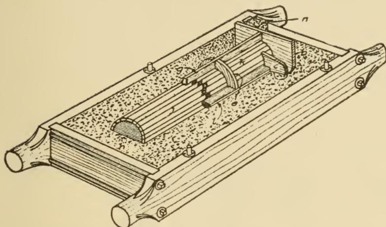
Fig. 367. Pattern Assembled on False Cope Ready for Ramming Cope Mold
