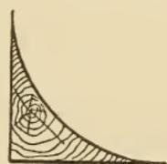
Fig. 197. Section of Wood Fillet
