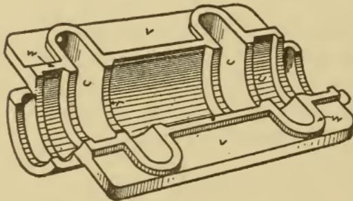
Fig. 287. Cap for Hanger Bearing
