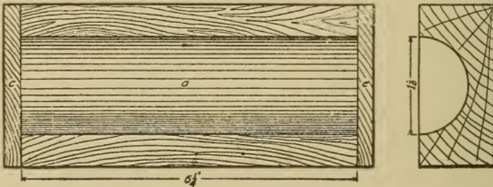
Fig. 158. Core Box for Pattern, Fig. 151
