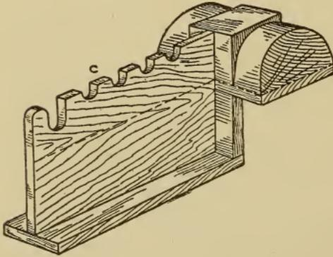
Fig. 346. Master Pattern for Cope Pattern *c*,
