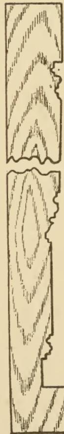
Fig. 269. Strike, for Making Loam Core for Column
