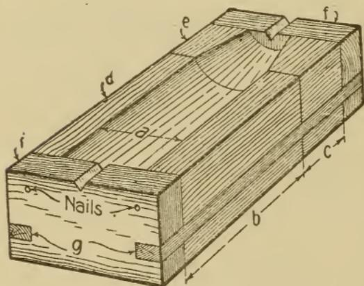
Fig. 148. Completed Core Box
