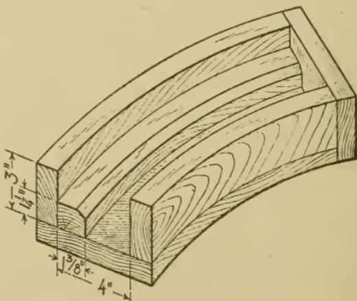
Fig. 189. Inside Flange Core Box
