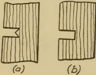
Fig. 12. Kerf Made by Crosscut Saw
