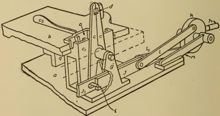
Fig. 347. Assembled View of Mechanism for Drag Machine
