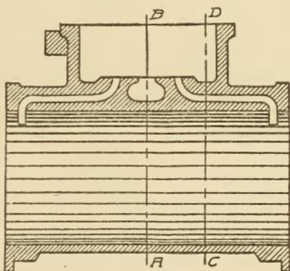
Fig. 244. Section through Slide Valve Cylinder
