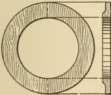
Fig. 221. Construction of Flanges for Pipe Pattern
