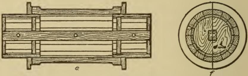
Fig. 246. Section of Cylinder Pattern
