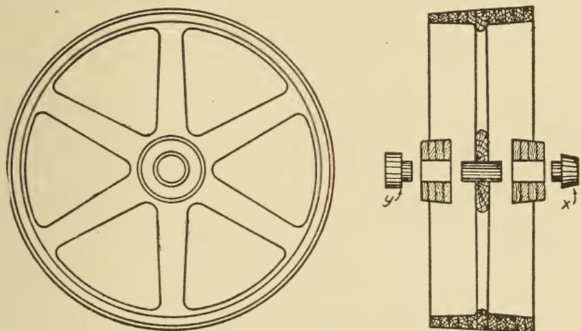
Fig. 177. Sectional View of Pattern for 20-Inch Pulley
