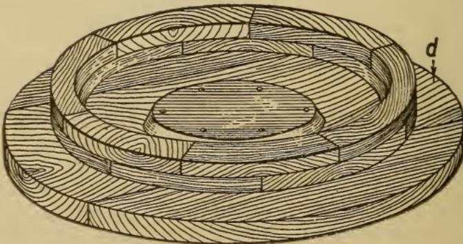
Fig. 378. Under Side of Pattern of Mold Plate
