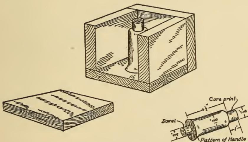
Fig. 370. Core Box for Cast-Iron Handle
