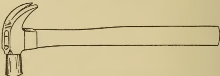
Fig. 73. Typical Pattern Maker's Hammer
