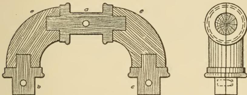
Fig. 210. Section of Double-Elbow Pattern
