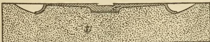
Fig. 122. Pulley Mold Coped-Out for Ring
