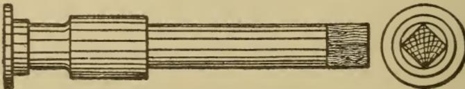
Fig. 243. Valve Spindle. (This pattern is not split)
