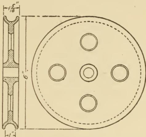
Fig. 159. Small Sheave Pulley
