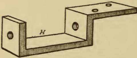
Fig. 333. Forge Steel or Iron Pattern Hanger
