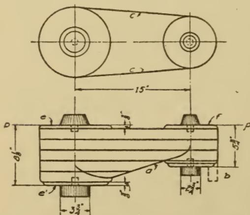
Fig. 193. Diagram of Pattern for Crank, Fig. 192
