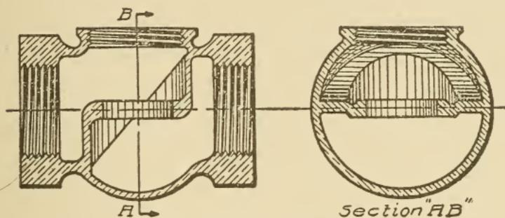
Fig. 230. Section of Valve Body
