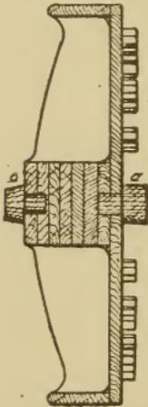
Fig. 199. Section of Pattern for Faceplate, Fig. 195
