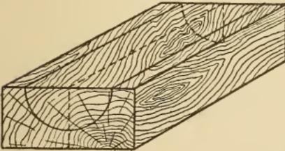
Fig. 36. Block Laid Out for Core-Box
