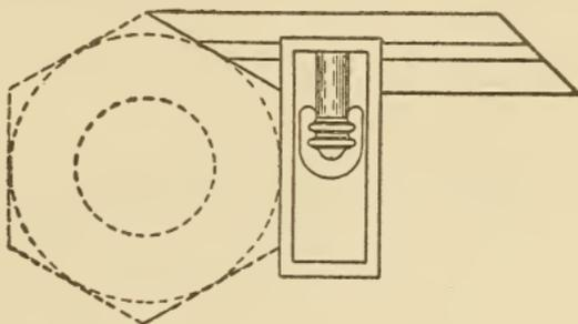
Fig. 57. Try-Square with Bevel-Ended Blade
