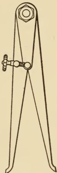
Fig. 72. Adjustable Inside Calipers
