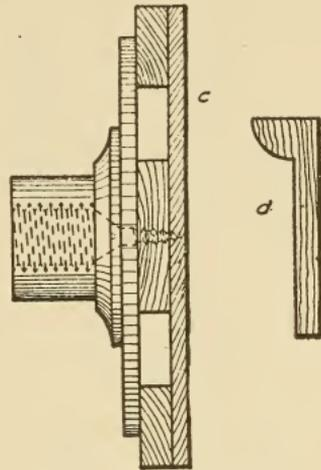
Fig. 164. Stock Mounted on Faceplate
