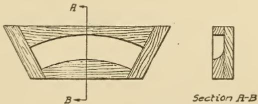
Fig. 169. Core Box for Single-Groove Rope Sheave
