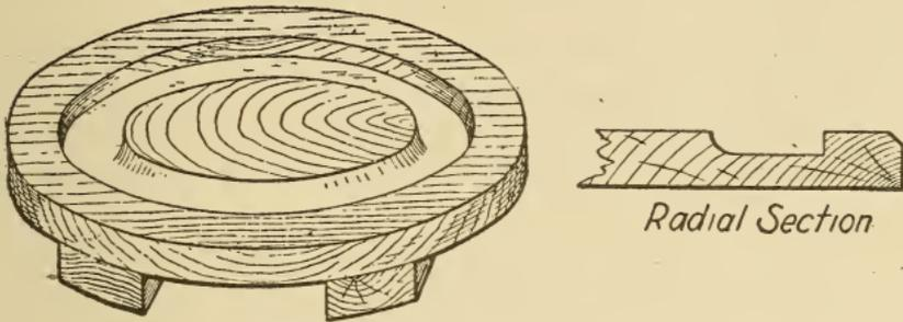
Fig. 168. Core Box for Sheave Pulley
