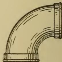
Fig. 209. Elbow Pipe Fitting
