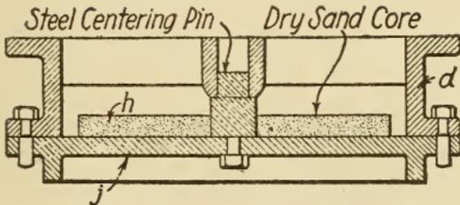
Fig. 380. Drag Flask on Mold Plate
