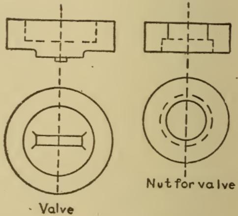
Fig. 242. Details of Valve and Valve Nut
