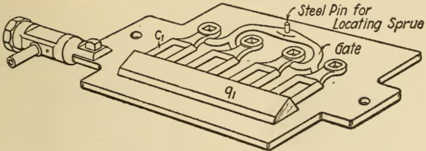
Fig. 326. Match Plate for Cope Mold with Vibrator Attached
