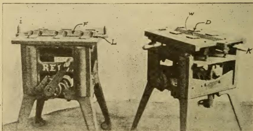
Fig. 329. Cope and Drag Machines for Molding Cover
