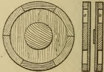
Fig. 163. Construction Views of Sheave Pattern
