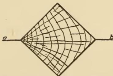
Fig. 136. Position for Molding without Added Draft
