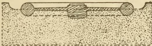
Fig. 115. Wheel Mold Coped Out
