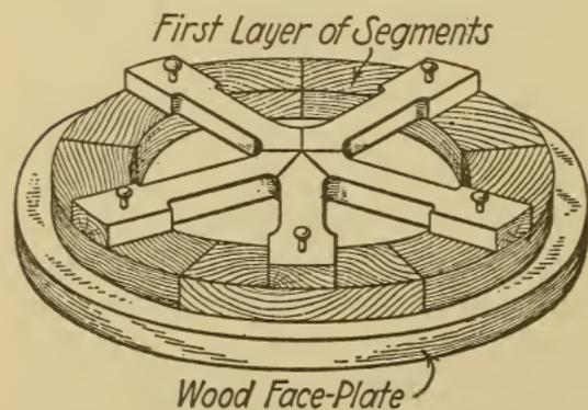
Fig. 173. Partially Assembled Rim and Pattern
