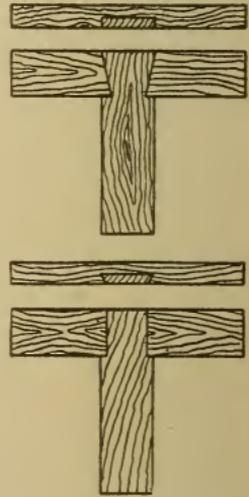
Fig. 45. Dovetail Joints
