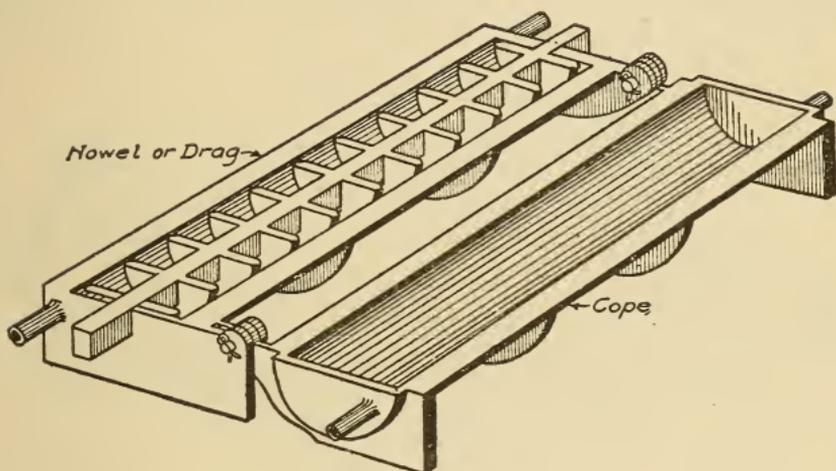
Fig. 363. Iron Core Box for Green-Sand Core
