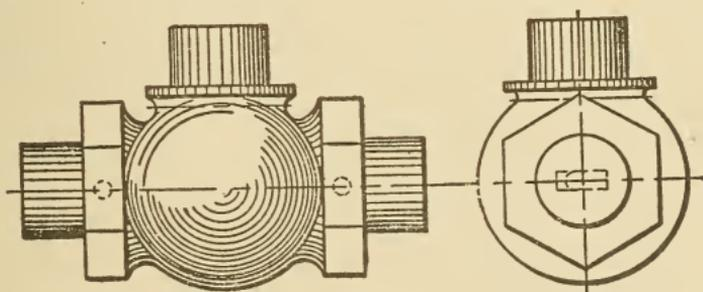
Fig. 231. Appearance of Pattern for Globe Valve
