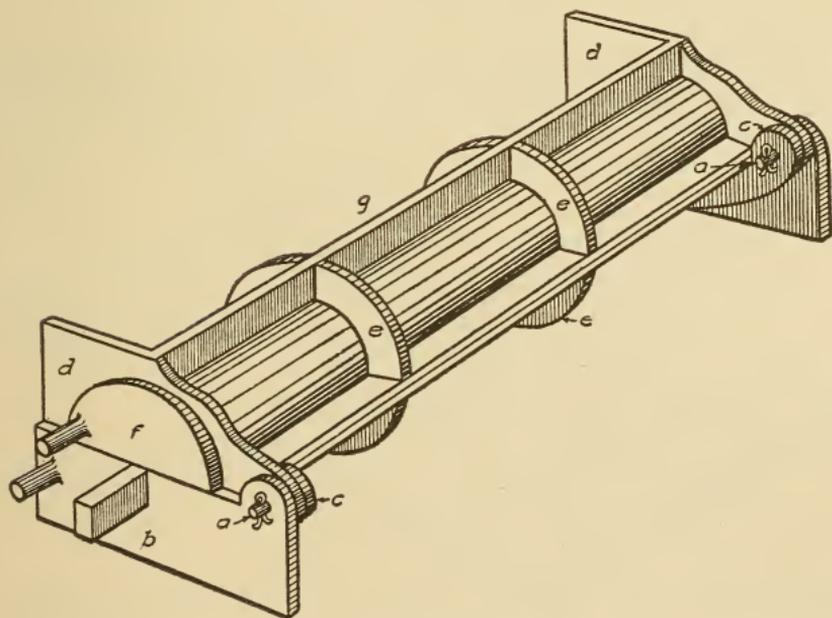
Fig. 364. Core Box Closed
