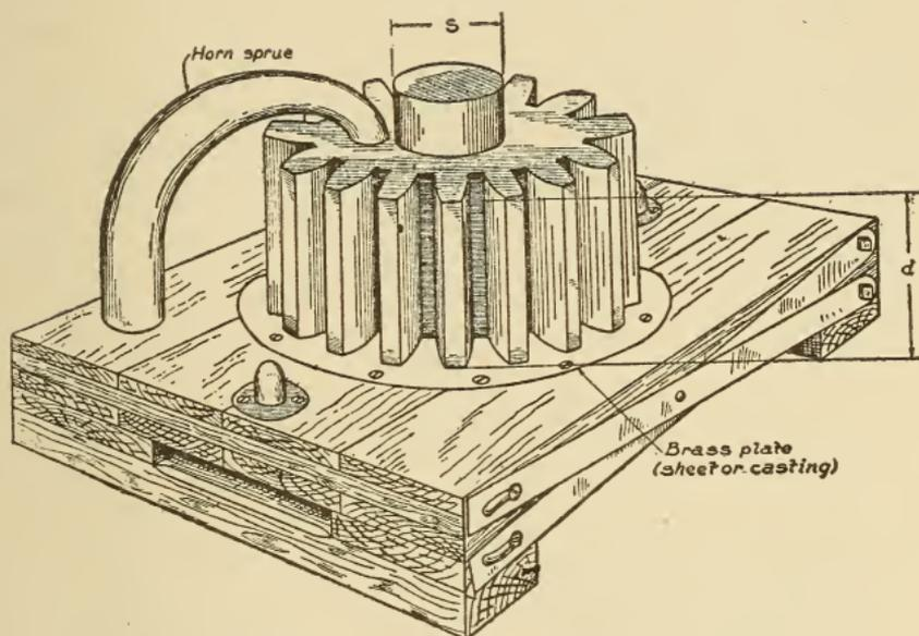
Fig. 302. Draw Plate for Spur-Gear Casting
