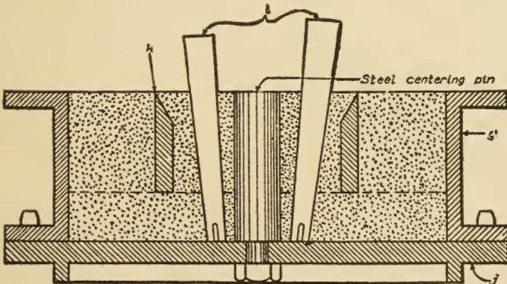
Fig. 381. Cope Mold on Mold Plate
