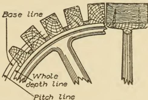
Fig. 254. Wood Spur Gear with Teeth Fastened with Wood Screws, Filler Pieces Glued between Teeth
