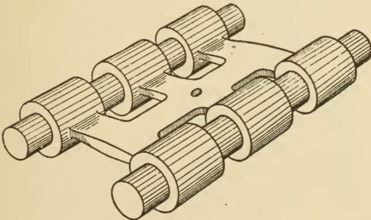
Fig. 228. Gated Pipe-Coupling Pattern
