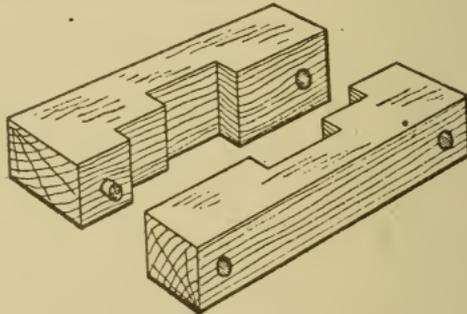
Fig. 200. Core Box for Faceplate Slots
