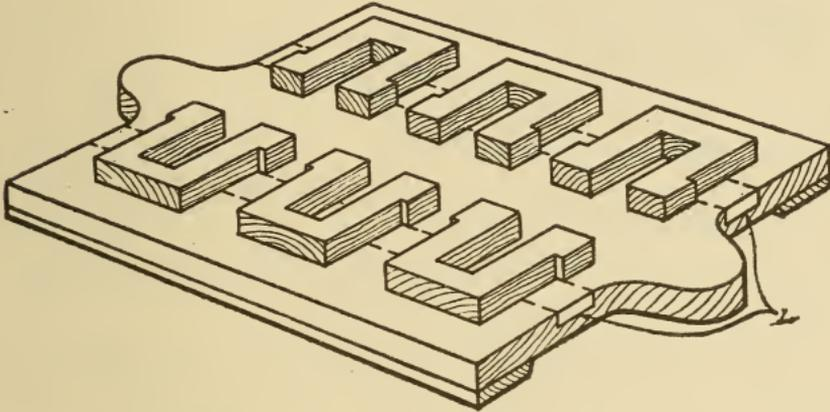
Fig. 336. Pattern for Drag Machine Stripping Plate
