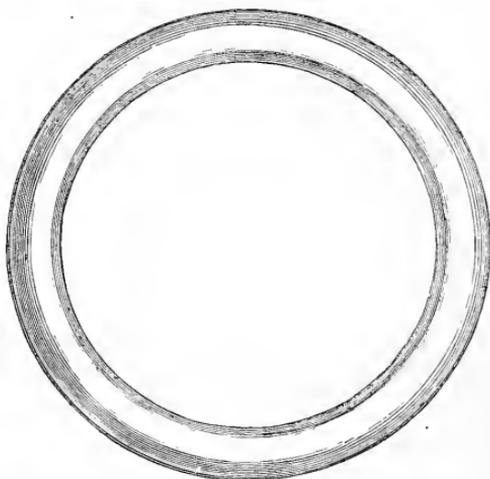
of rings of copper wire covered with gutta percha; they measure from  $2\frac{1}{4}$  inches to  $4\frac{1}{2}$  inches in diameter, and are numbered 1, 2, 3,  $3\frac{1}{2}$ , 4, 5, and so on. As supplied by the maker (Mr. Coxeter was the first to make them), they are quite round. When properly made, and the gutta percha of good quality, they are very readily moulded to a proper shape, that shape being adapted to the case, and the ring of a proper size selected for use.
