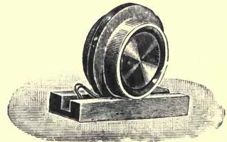
Fig. 101.—Kirchner's Apparatus for testing Resistance to Folding.
