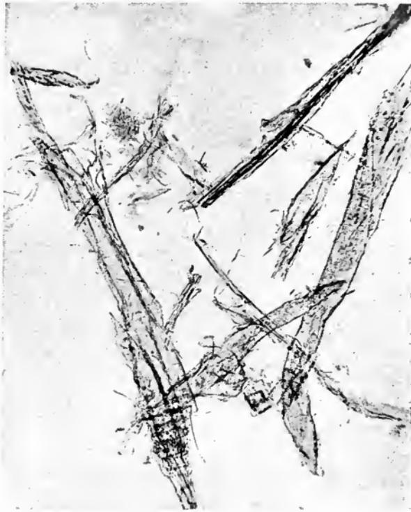
FIG. 9. MECHANICAL WOOD-PULP FIBRES
