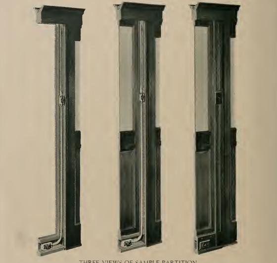
THREE VIEWS OF SAMPLE PARTITION Showing progressive steps in assembly of partition, installation of either rigid metal or flexible conduit and electrical outlets, and the concealment of the conduit in the completed partition.
