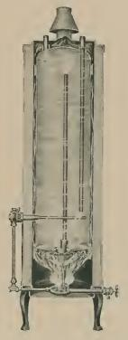
A six-jet Barber patented burner evenly distributes heat over the entire surface of the fan-shaped brass spreader, thus maintaining a uniform and constant circulation of water.
