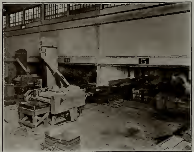
The machine method of making tinplate. Only one unskilled operator required to feed the black sheets into the machine. All the processes of tinning, handling and cleaning conducted automatically thereafter, the finished sheets being delivered on the stand shown at the left in the illustration.
