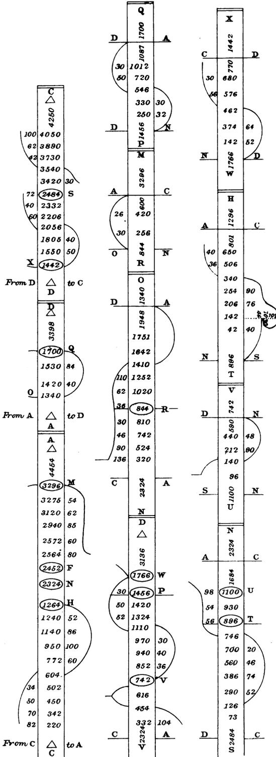
SPECIMEN OF DETAIL SURVEYING IN A TRIANGLE
