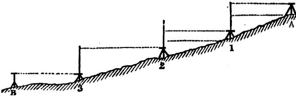
But the necessity for these corrections is avoided by simply placing the instrument half-way between the two stations, and either in the line of section, or on one side of it.
