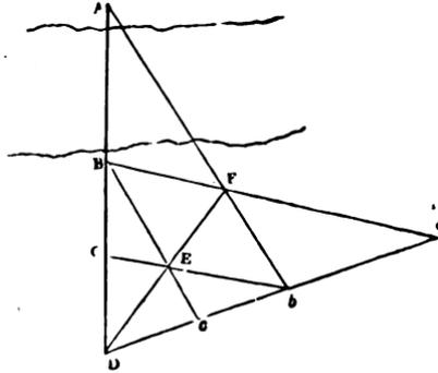
To measure the distance between  $A$  and  $B$ , both being inaccessible:—From any point  $C$  draw any line  $Cc$  bisected in  $D$ ; take any point  $E$  in the prolongation of  $AC$ , and join  $ED$ , producing the line to  $De = ED$ ; in like manner take any point  $F$  in the prolongation of  $BC$ , and make  $Df = FD$ .
