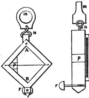
turned round, and the observer, placed between it and the wall, with his back to the latter, notes the spot where the *image of his eye* coincides with the reflected wall *above or below the former mark*. The mean distance between these two points is assumed and marked, and by turning the screw  $r$ , the centre of gravity of the mirror is altered until the image of the eye coinciding as before with the silk
