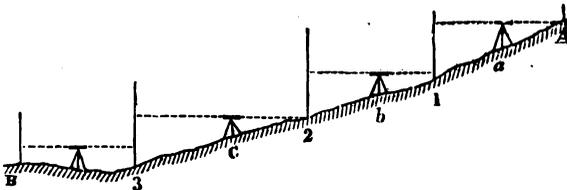
and at the forward station (1), gives at once the difference of level between the ground at these points without any correction for *refraction* or *curvature*, and also without taking into account the
