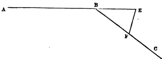
required to be measured, prolong A B to E, make B F equal to B E, and measure the chord E F, from which data the direction of B C can be laid down.
