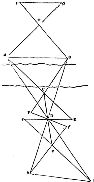
A right angle\* can often be laid off when no means of measuring other divisions of the circle are at hand. The distance A B can then be thus obtained :—
