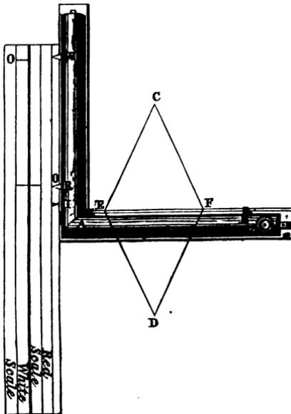
The instrument consists of a square, and a graduated scale, corresponding with that of the survey.
