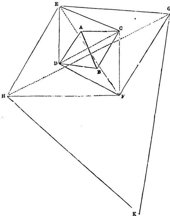
already stated that the sides of the principal triangles should increase as rapidly as possible from the measured base. The accompanying sketch will show how this is to be managed without admitting any *ill-conditioned triangles*.
