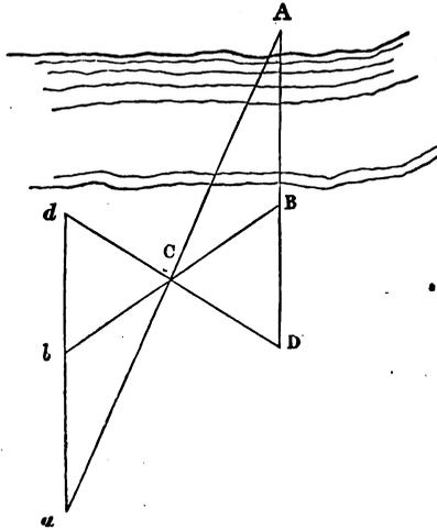
measure angles.—(This and the two following are taken from the "Aide Mémoire.") A is any inaccessible point the distance of which from B is required: produce A B to any point D; draw D d in any direction bisected in C; join B C and produce it to b, C b being made equal to B C; join d b and produce it to a, the intersection of the prolongation of A C, then
