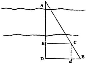
Of course with a sextant, or other means of observing the angle A C B, A B becomes simply the tangent of that angle to the radius B C : a table of natural sines and tangents engraved on the lid of the box-sextant, or on any portable reflecting instrument is often of great service, particularly in sketching ground without any previous triangulation, and in obtaining the distance to an enemy's batteries, &c., on a military reconnoissance. The height
