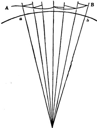
nearly enough), and  $h$  the elevation, the measured lengths must be multiplied by the fraction  $\frac{r}{r+h}$  or  $1 - \frac{h}{r}$ , or they must be diminished by the part  $\frac{h}{r}$  of the whole. If the surface slopes uniformly, the mean height may be taken ; if it is very irregular, it may be divided into several parts."
