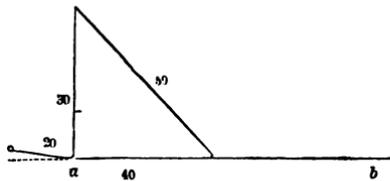
An angle equal to any other angle can also be marked on the ground, with the chain only, by measuring equal distances on the sides containing it, and then taking the length of the chord : the same distances, or aliquot parts thereof, will of course measure the same angle
