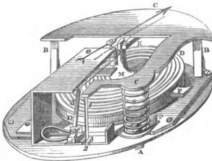
D D is the cylindrical vacuum box ; C C the lever, to the end of which is attached the vertical rod *i*, connecting it with the other levers acting by means of a piece of watch spring upon the roller carrying the index
