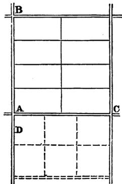
\* This figure represents rectangular sections of 80 acres, as laid out in South Australia, the length of which bore to their breadth the proportion of 2 to 1—occupation roads one mile apart, enclosing eight sections. They were, however, frequently laid out square, according to the nature of the ground.
