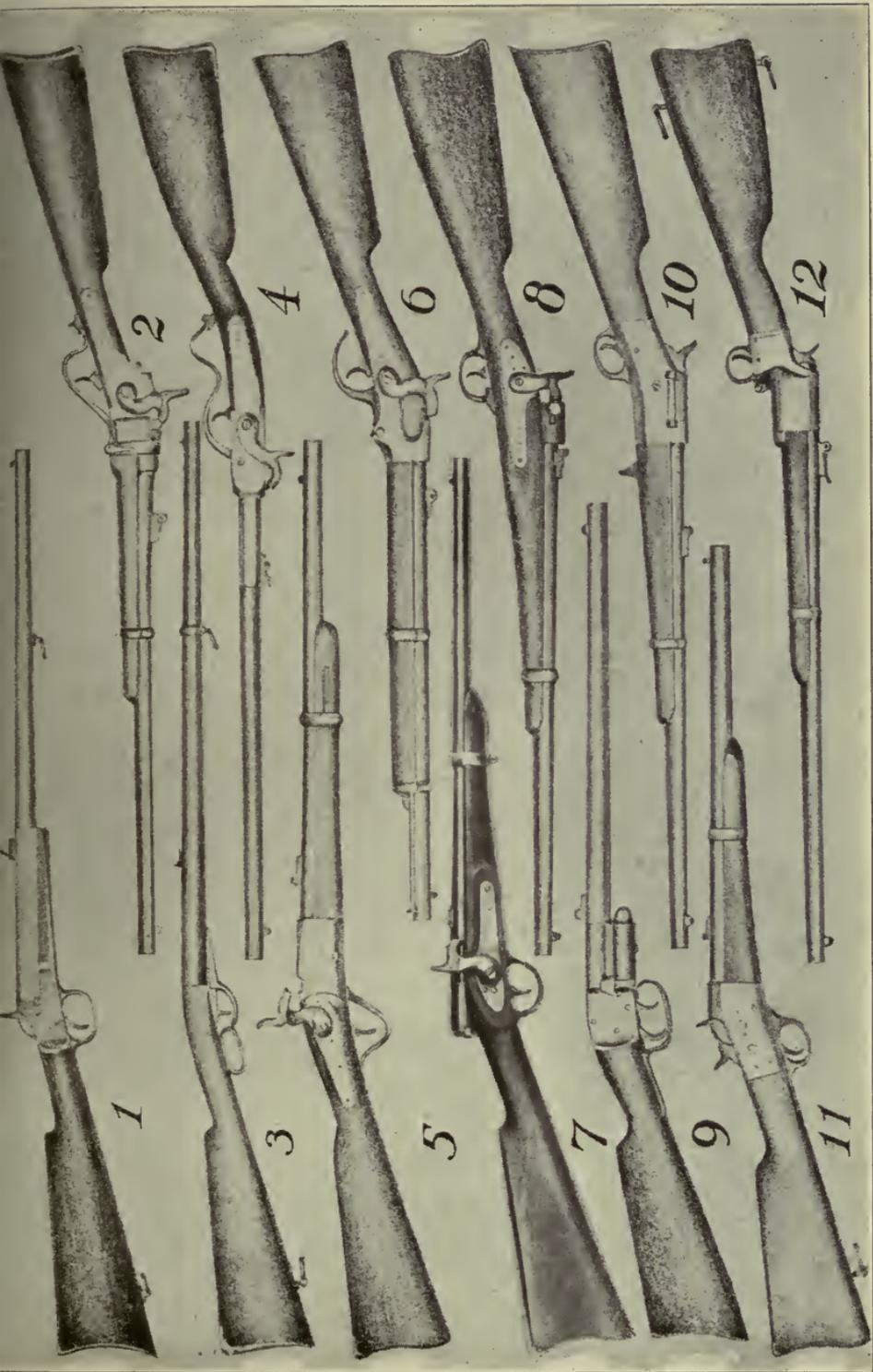
*No. 5, Peabody.* 1862. Henry O. Peabody's patent of 1862. The first few were made with internal hammer. Metallic cartridge, single shot, rim fire, calibre .50. Marked "Providence Tool Co."
