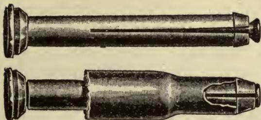
Extractor with section of broken shell
