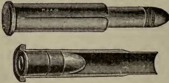
With the supplemental chamber .22 rim fire ammunition can be fired in a .22 hi-power rifle; .32 S. & W. in .30 and .303 rifles; .32 short Colt in .32-40; .38 S. & W. in .35; and .41 short Colt in .405 rifles. Only smokeless powder cartridges should be used with supplemental chambers because black powder in quick twist barrels leaves too much fouling.
