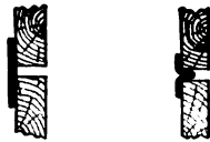
FIG. 530. FIG. 531. VEZIN'S DUST-PROOFING DEVICE.
