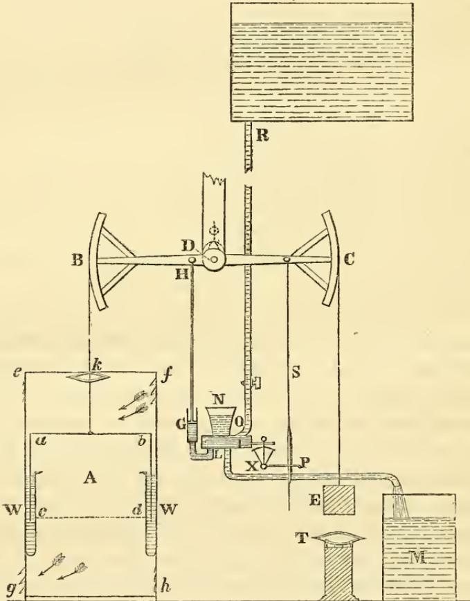
It hangs by a rope from the end of the beam B C, vibrating on an axis at D, at the other end of which beam hangs the counterpoise, E.
