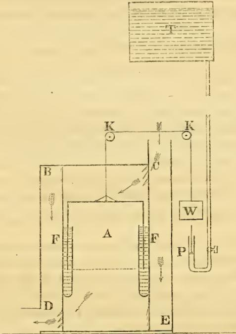
enters the pump simultaneously by corresponding admission valves near C and E, out of the channel C F E, by which the pure air approaches the pump. A cylinder containing 500 cubic feet, making two double strokes in the minute, would supply the required quantity; or one of smaller dimensions, with quicker motion. The choice to be determined by circumstances.
