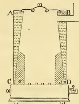
lid, not riveted but cemented in its place, which closure is sufficient where there is little pressure of water or steam against it.
