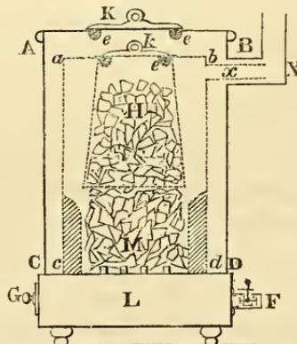
The letters A B C D mark the external case, which prevents the intense heat of the inner stove *a b c d* from damaging the air of the room.
