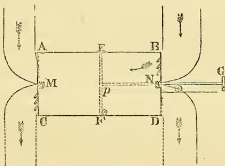
wood like a packing-case, made accurately square, resting on its side. Within the case is a moveable partition E F, fitting the box like the piston of a pump to within the 20th of an inch on all sides, so that it may be pushed to and fro with little friction and impediment. This moveable partition has a stalk or piston-rod P G, to the outer extremity of which G, a
