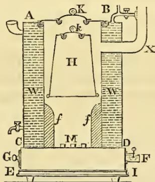
adjoining cut. The external case of the stove ABCD is double, and water, as represented by the short horizontal lines, is contained between the outer and inner plates or walls. This constitutes, what may be called, a water-clad stove.
