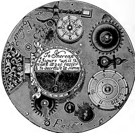
FIG. 830.—An early application of the Balance Spring.
