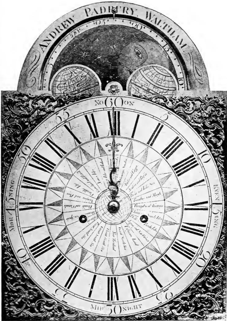
FIG. 684.—Dial of Clock, by Andrew Padbury, with rotating centre to indicate time all over the world.
