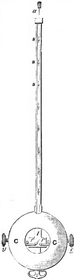
FIG. 479.—Ellicott's Compensation Pendulum.
