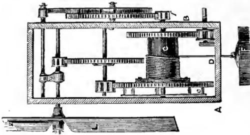
Fig. 27.—Side view of striking part.
