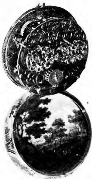
FIG. 233.—Movement and inside of Case.
