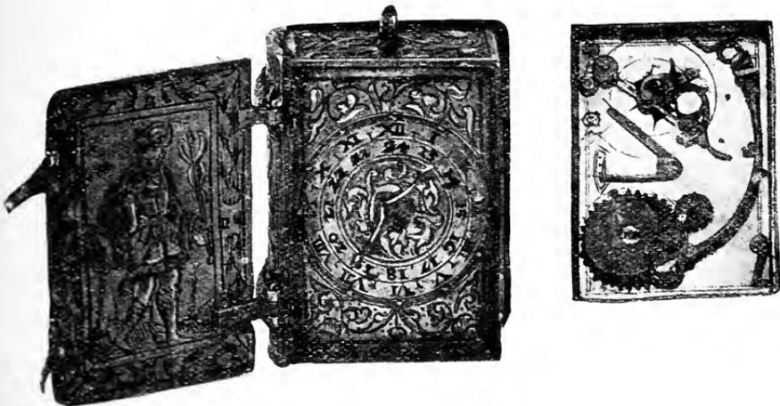
FIGS. 151-153.—Sixteenth-Century Book-Watch. Outside with Covers open, inside of front Cover and Dial. View of mechanism inside back Cover.
