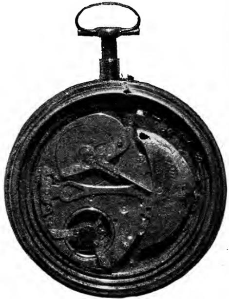
FIG. 840.—Self-winding or "Pedometer" Watch, by Breguet.
