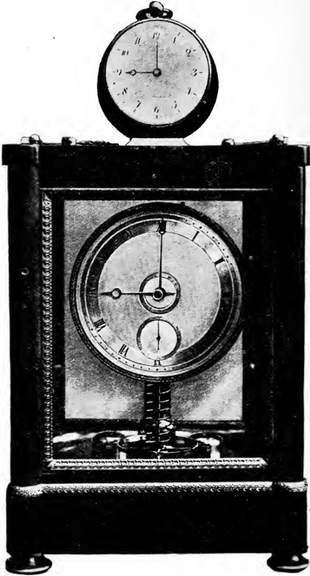
FIG. 516.—Breguet's Synchronizer. The mainspring barrels are in the base of the case, the winding being accomplished by means of a rack and lever underneath. Above the base may be seen the compensation balance, and rising from it part of a tall balance-spring, which is of gold.
