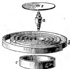
FIG. 77.—Mainspring and Barrel.
