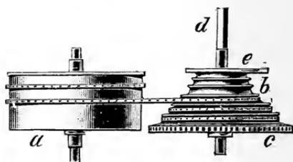
FIG. 78.—Mainspring Barrel and Fusee.
