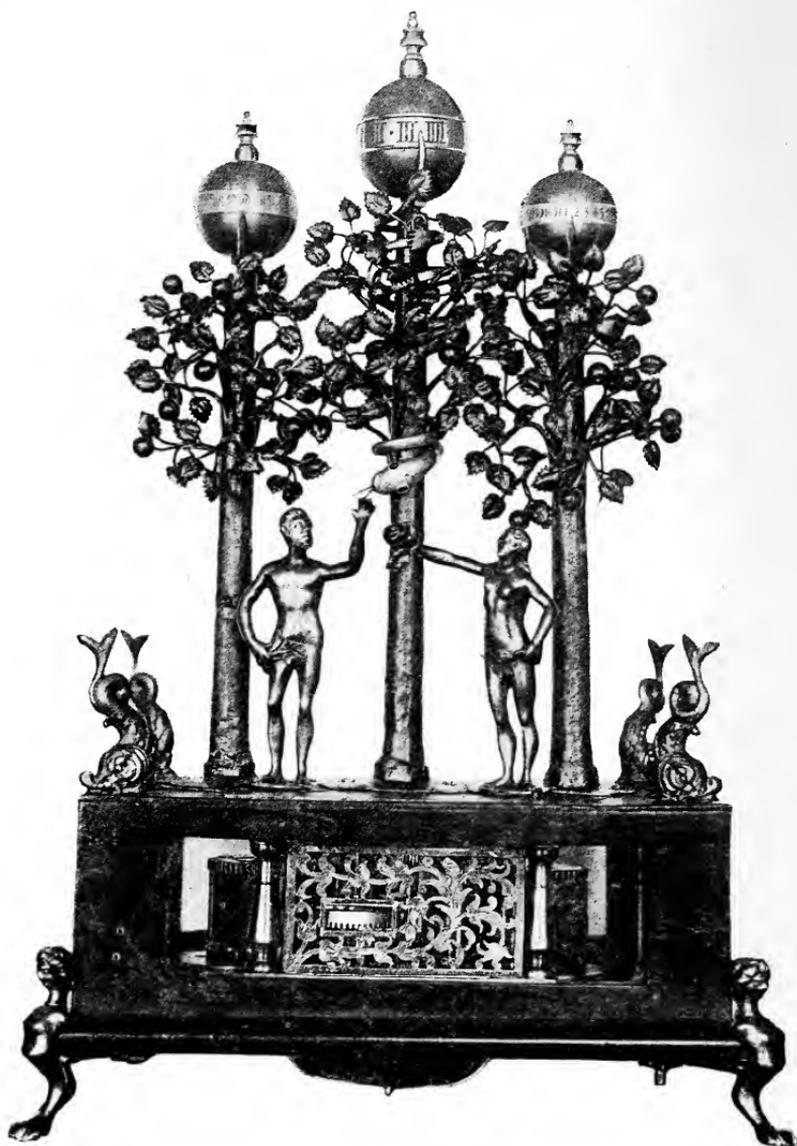
FIG. 117.—Clock with three horizontal band dials showing the hour, the day of the week, and the day of the month.
