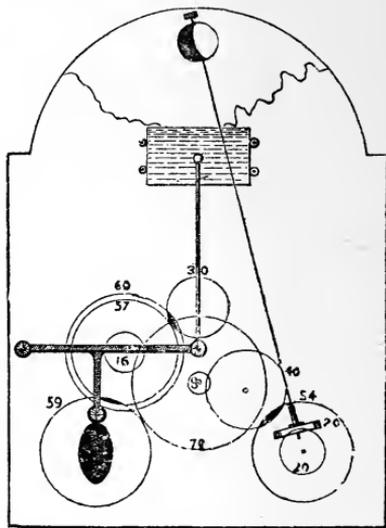
FIG. 510.—Mechanism at back of dial.
