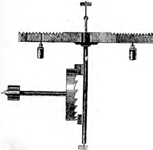
FIG. 28.—Verge Escapement with Cross-bar or "Foliot" Balance.
