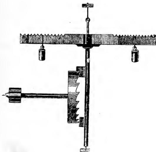
FIG. 28.—Verge Escapement with Cross-bar or "Foliot" Balance.
