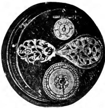
FIG. 349.—Watch with no balance spring.
