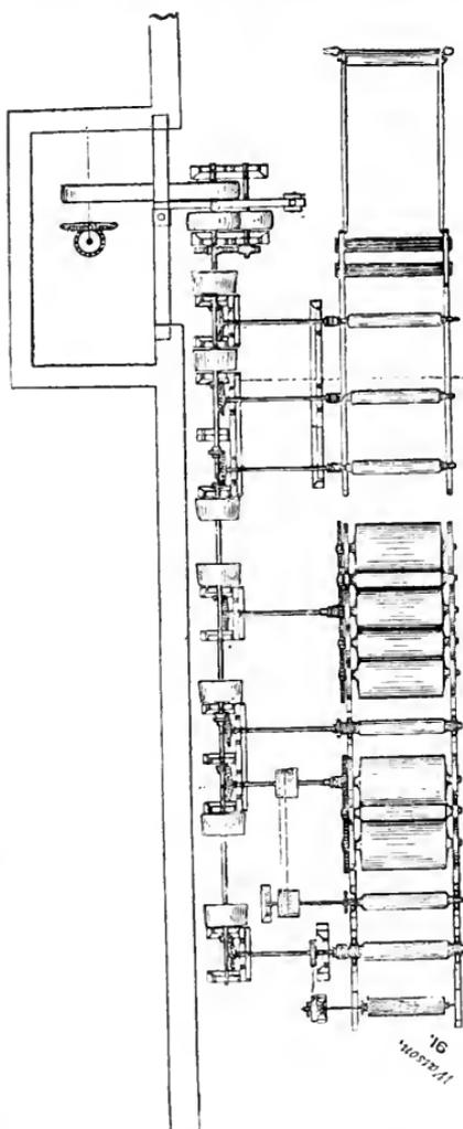
PLAN OF PAPER-MAKING MACHINE WITH "MARSHALL" DRIVING GEAR.
