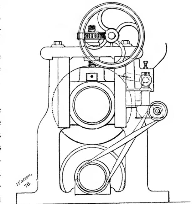
PRESS ROLLS WITH IMPROVED PARALLEL LIFTING GEAR.
