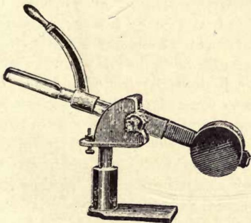
*Hollow-Ware Jolleys.*—Small hollow ware can be made on the machines used for flat ware; the heads, however, must be deeper, and shaped like an ordinary flower-pot, so that the moulds fit
