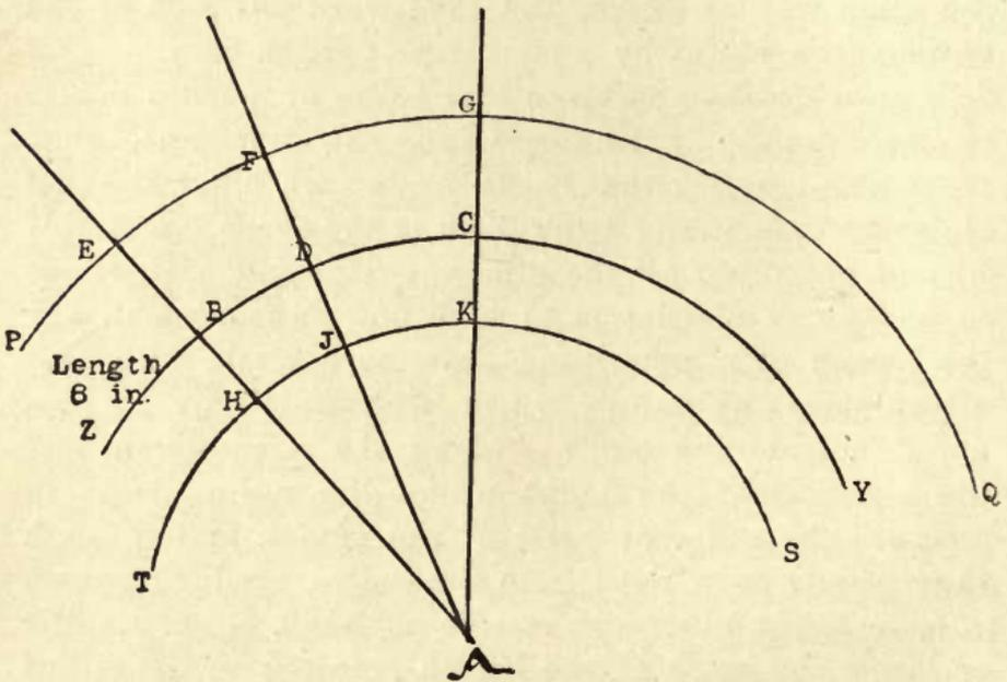
cuts the produced radii, measure to E along the circumference of the circle PQ, give the dimensions required. That is to say, the distance between E and F is the depth, and between E and G the width of the 10-inch dish. In like manner for the 6-inch dish, measure 6 inches from A to H and describe circle TS. H to J is the depth of the 6-inch dish and H to K is its width. In this manner any number of different measurements may be made, such as height, breadth of edge, slope
