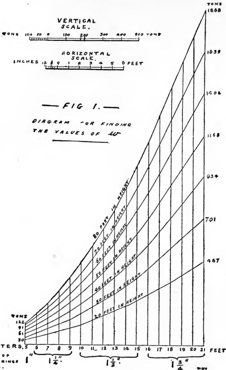
Note.—The weights in the diagram are calculated on the assumption that the hearting of the cylinder is Portland cement concrete. If brick-work, the weights will be about 16 per cent. less for picked stock bricks set in Portland cement mortar.
