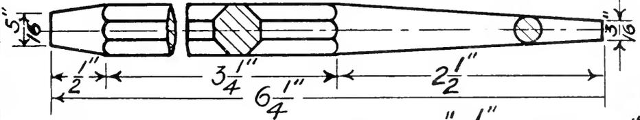
Cold Chisel. Stock  $5'' \times \frac{1}{2}''$  Oct. Steel.
