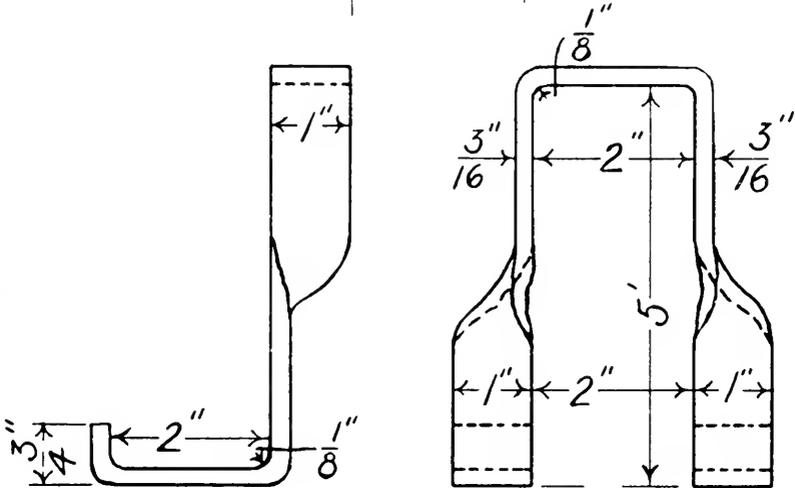
punch mark and bend over the horn. This must be done rapidly or the iron will become too cold. After bending at both marks, be sure the work is square and measurements correct.
