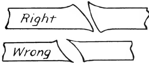
FIGURE 18. FORMING SCARF.
