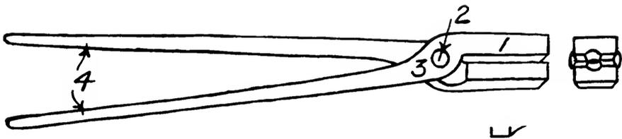
FIGURE 4. NAMES OF PARTS OF BLACKSMITH'S TONGS.
