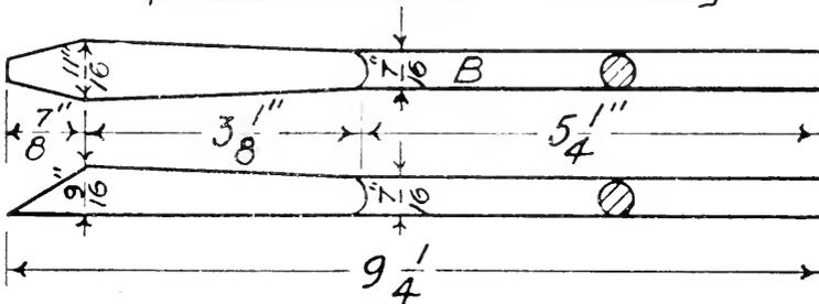
*wide side is much stronger than on the narrow side, the strain being downward and if made on the narrow side, it would have a tendency to open if it should be a weak weld.*
