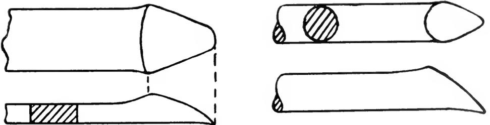
FIGURE 19. FORMING SCARF ON ROUND AND FLAT STOCK.
