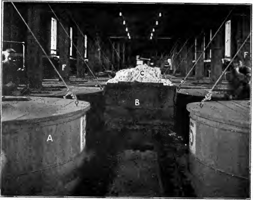
FIG. 286.—Nitrocellulose Wash House. A , Wash Vats, where the Nitrocellulose from Nitrating House is placed for the Preliminary Series of Washings with Steam. B , Truck, containing C , Nitrated Cotton. The Number of Separate Washings of the Nitrocellulose is Shown by means of the Indicators Shown at E . F , Wooden Steam Vent Flues. The Tanks Shown are about 7 Feet Diameter, and 8 Feet Deep, extending to the Floor of the Story Underneath. (See also Fig. 287.)
