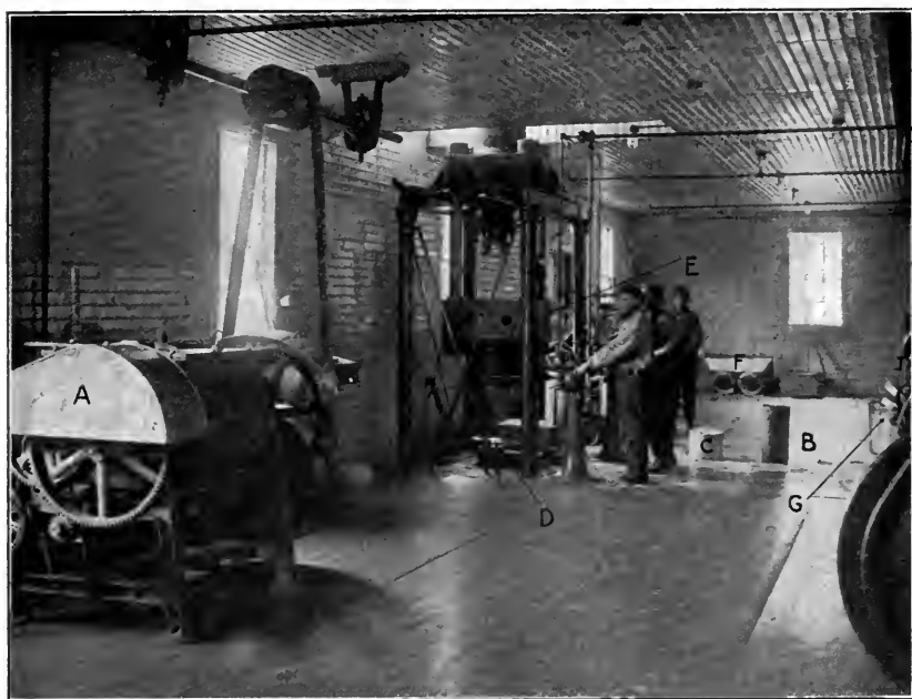
FIG. 291.—Smokeless Powder Manufacture. A , Kneading or Colloiding Mixer for Gelatinizing Nitrocellulose; B , Block of Colloid after having been Pressed into a Solid Cylinder; C , Block of Ungelatinized Nitrocellulose; D , Hydraulic Press for Transforming Loose Colloid from Mixer A into Cylinder B ; E , Macaroni Filtering Press; F , Arrangement for Transferring Equally the Colloid from A to the Cans G . The floor is linoleum covered.
