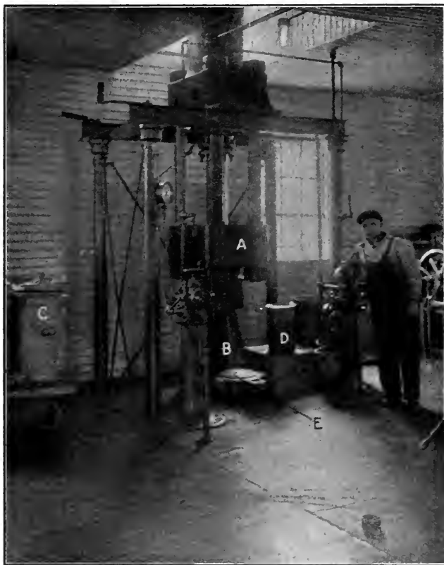
FIG. 288.—Hydraulic Filtering or “Macaroni” Press, for Removal of Solid Impurities from Colloided Nitrocellulose. A , Press; B , Filtered Colloid, in Strings as Issuing from the Press; C , Can, in which the Blocks D , of Colloid are Kept when not Passing through the Press. E , Top of Blocking Press, in which the Colloid Strings are Compacted again into a Solid Cylinder D .
