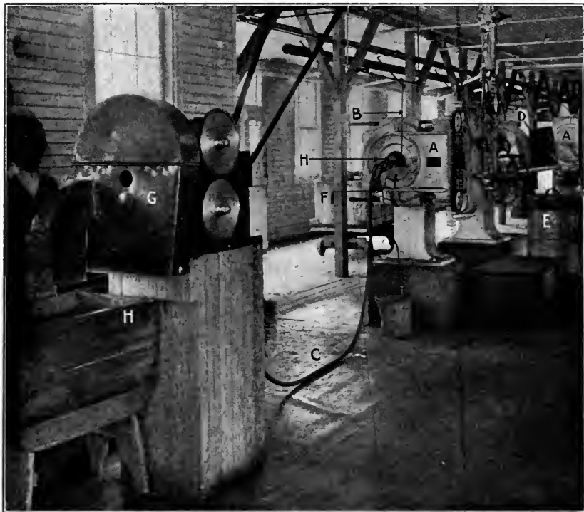
FIG. 293.—Formation of Smokeless Powder Grains. A , Hydraulic Press in which the Block A of Gelatinized Nitrocellulose, is Forced through the Orifice H , Resulting in the Formation of a Concentrically Perforated Tube C , which is Drawn over the Wheel F , to the Powder Cutter G , being Cooled as it Issues from the Press, by a Circulation of Cold Water through the Pipe B . C is a Rope of 12-in. Powder.
