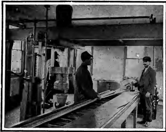
FIG. 298.—End View of Hydraulic Finishing Press for Smokeless Powder Manufacture. From the Issuing Orifice, the Endless Rope, Perforated from End to End with a Concentric Group of Circular Passages is Led to the Powder Cutter.
