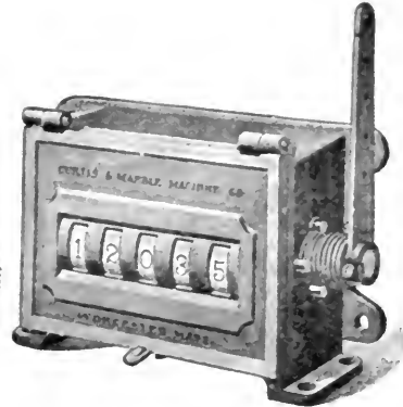
FIG. 103.—Counting Register for Measuring Cloth.
