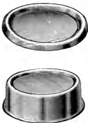
FIG. 78.—Tin Cup to Cover Varnish Can Nozzle after Opening.
